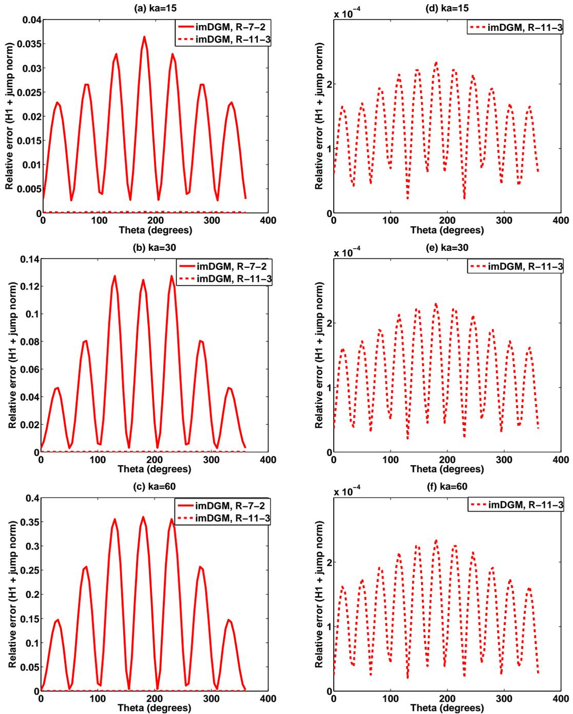
Fig. 14 – Performance comparison between imDGM ( $R-7-2$ ) and imDGM ( $R-11-3$ ) for  $kh = 3/2$  (left). Zoom on imDGM( $R-11-3$ ) for  $kh = 3/2$  (right).
