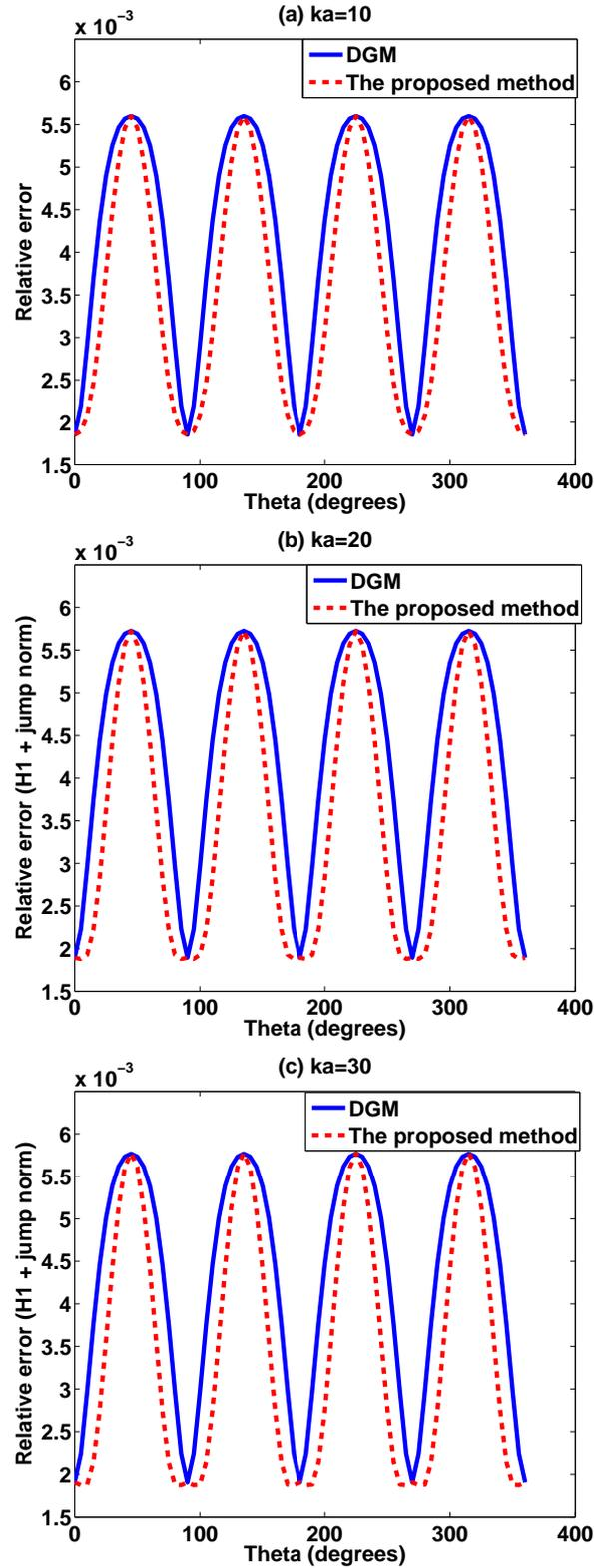
**Fig. 6** – Comparison between DGM and the formulation given by (31)-(30) in the case of the  $R$ -8-2b element for (a)  $ka = 10$ , (b)  $ka = 20$  and (c)  $ka = 30$
