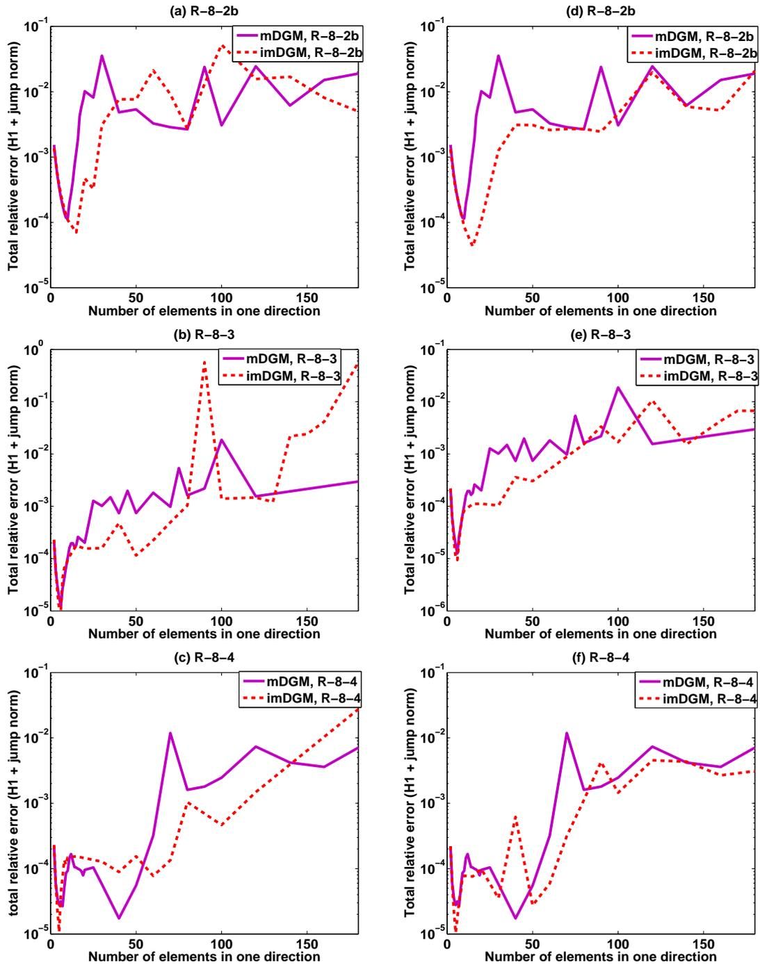
Fig. 4 – Sensitivity of the accuracy to the mesh refinement :  $ka = 1$  and weight parameters values :  $\beta_e = k^2$ ,  $\delta_e = \omega_e = 1$  (left),  $\beta_e = k^2$ ,  $\delta_e = \omega_e = h$  (right).
