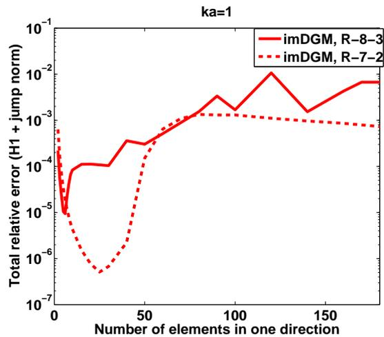
**Fig. 7** – Sensitivity of the total relative error to the mesh refinement : Comparison between imDGM ( $R$ -8-3) and imDGM ( $R$ -7-2) for  $ka = 1$ .
