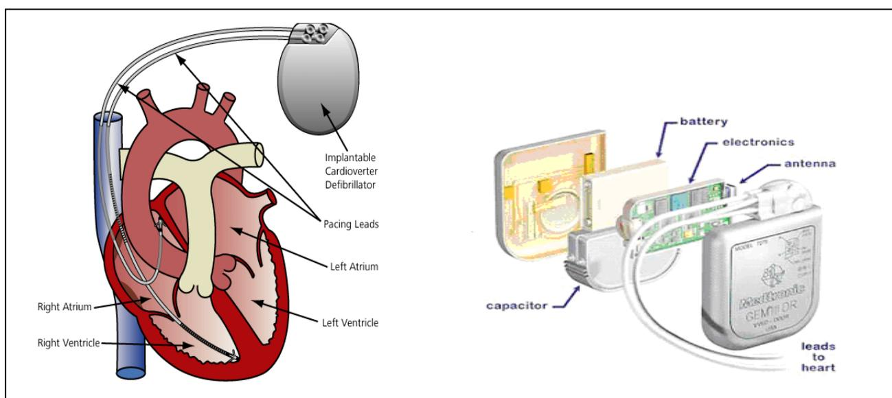
**Figure 24:** ICD Structure.
