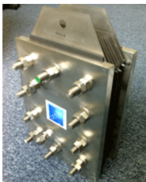
(a) Electrolyzer stack
