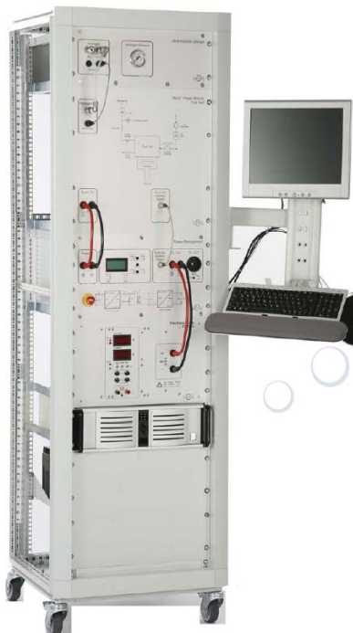
(c) Installation of the fuel cell system
