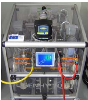
(c) Electrolyzer system
