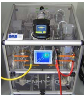
(c) Electrolyzer system
