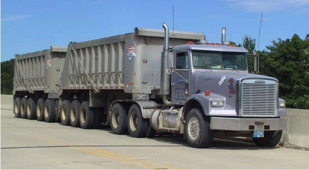
Figure 3.11 Three-unit 11-axle truck used in the field tests
