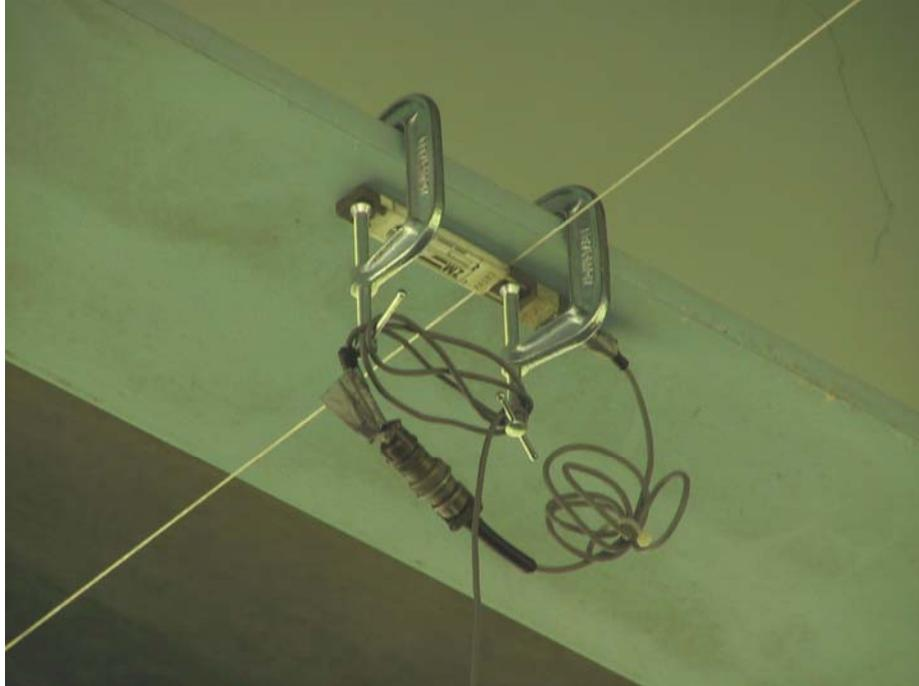
Figure 3.5 Removable Strain Transducer attached to the bottom flange
