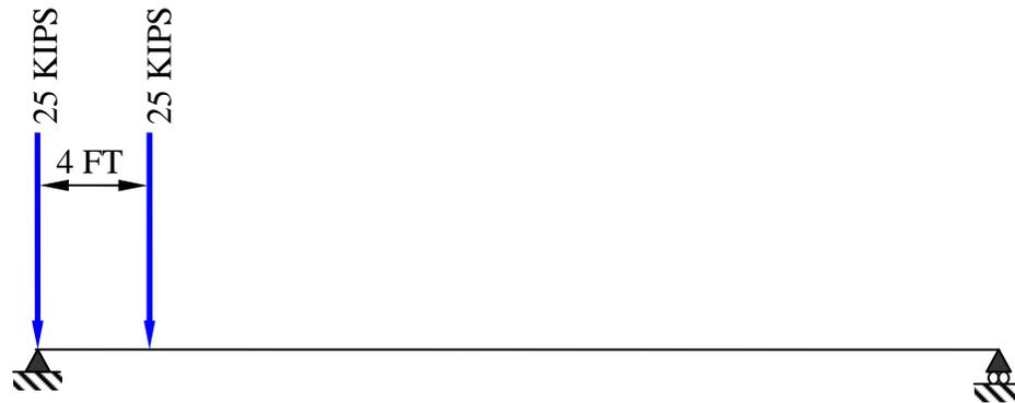
Figure A.8 Tandem placement for the maximum shear
