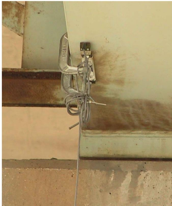
Figure 3.6 Strain transducer attached near support
