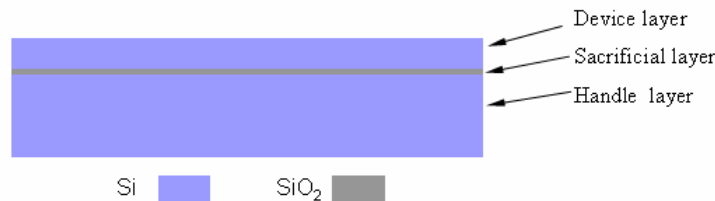
Fig. 4.20. Structure of SOI Wafer.
