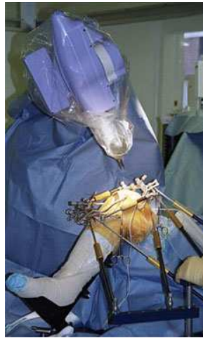
Figure 2.7: ACROBAT robot in orthopaedic surgery aimed at hip reparation. (Photo: http://medgadget.com ).
