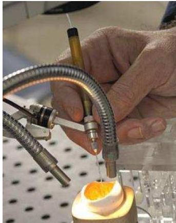
Figure 2.4: Cooperative manipulation: a microsurgical instrument held by both an operator and a robot. Device, developed by JHU robotics group, aimed at injecting vision-saving drugs into tiny blood vessels in the eye (Photo: http://www.sciencedaily.com ).
