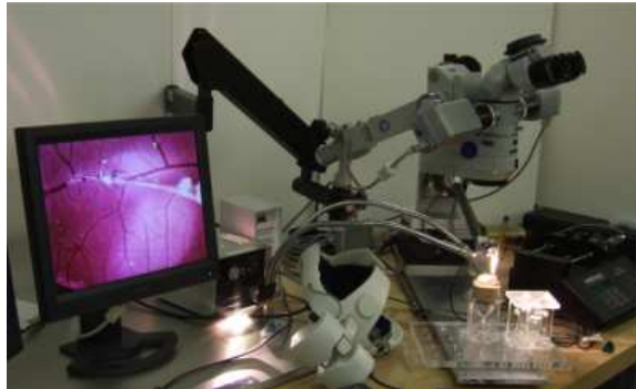
Figure 2.6: Microsurgery robotics: micro-surgical assistant workstation with retinal-surgery model. (Photo: http://www.cs.jhu.edu/CIRL/ ).
