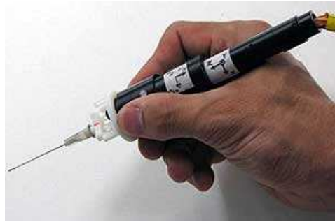
Figure 2.5: Hand-held instrument for microsurgery. (Photo: http://www3.ntu.edu.sg/ ).
