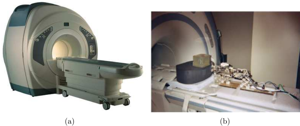
Figure 2.8: MRI-based needle insertion robot (a) High field MRI scanner (Photo: http://www.bvhealthsystem.org ) - (b) MRI needle placement robot [30] (Photo: www2.me.wpi.edu/AIM-lab/index.php/Research ).
