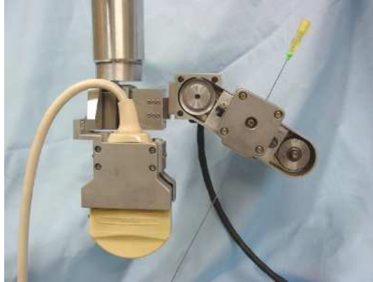
Figure 2.15: 2 DOFs robot for 2D ultrasound-based needle insertion. (Photo: taken from [38]).
