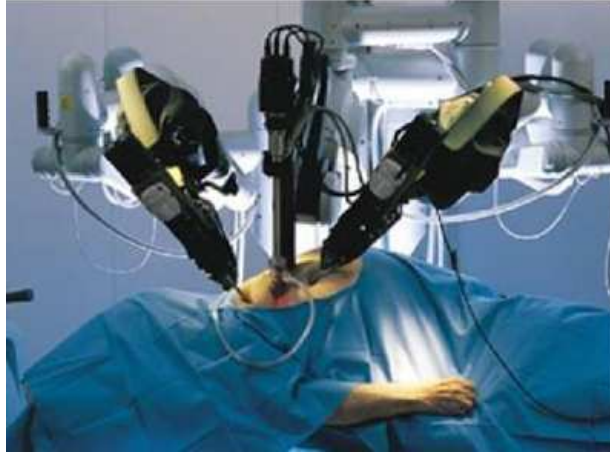
Figure 2.2: Example of endoscopic surgery robot (Da Vinci robot) in action. (Photo: http://biomed.brown.edu/.../Roboticsurgery.html )
