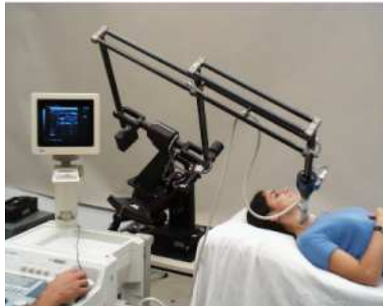
Figure 2.14: Robotic system for medical diagnostic ultrasound [1]. (Photo: S. E. Salcudean's research group web page http://www.ece.ubc.ca ).
