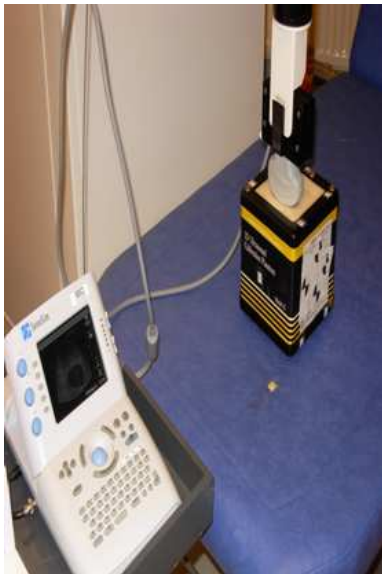
Figure 5.23: The probe transducer interacting with an ultrasound phantom.
