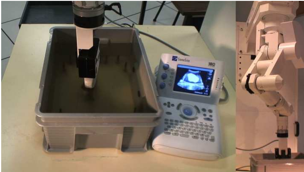
Figure 5.20: Experimental setup - A 6 DOFs medical robot arm (right) actuating a 2D ultrasound probe (left), which is interacting with an object immersed in a water-filled tank. The observed image is displayed on the imaging system screen (middle).
