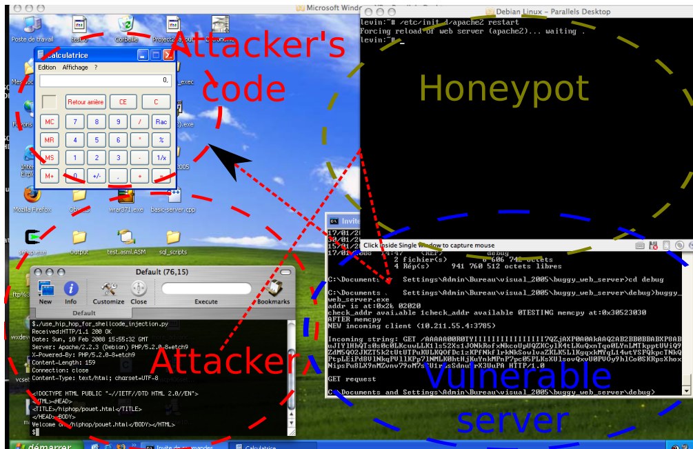
Figure 3.3: Making PHP.HoP launch a stack smashing exploit.
