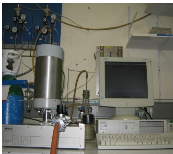
Figure II.9 : DSC NETZSCH ATD-DSC 404S.
