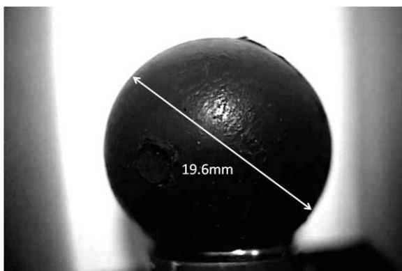
Fig.V.9a Spherical sample ( D=19.6\text{mm} ) without external field ( B_0=0\text{T} )
