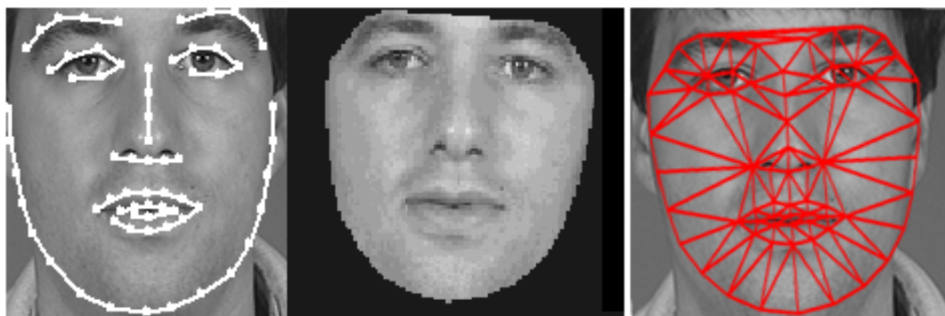
Figure 2.4: Shape, Texture and Delaunay Triangulation
