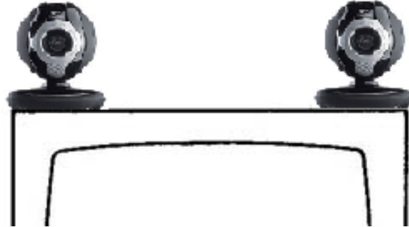
Figure 1.5: Example of double camera installation
