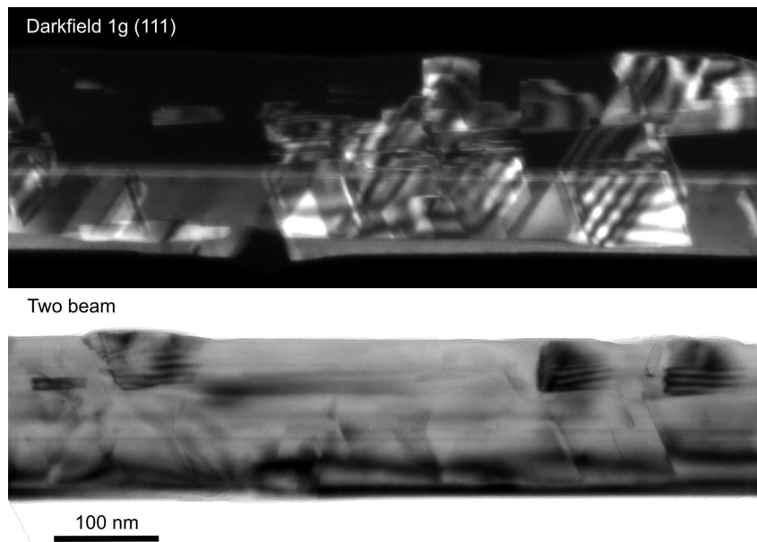
Figure 6.14: (A) Darkfield image of a nanowire grown using a Ni catalyst, made using the 1g (111) excitation. (B) Two beam image of the same nanowire. Sample 4530
