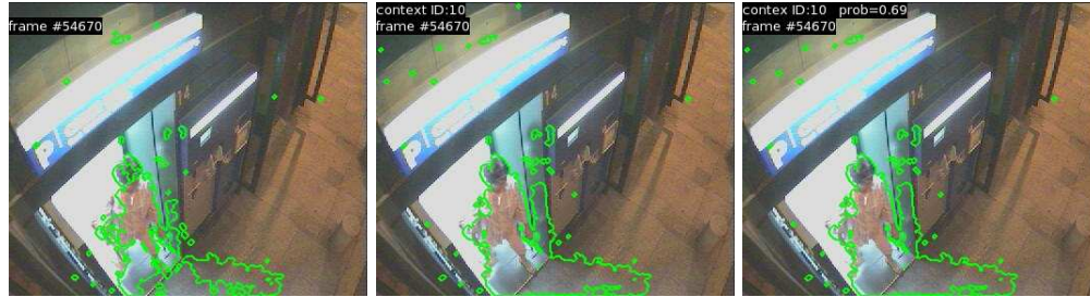
Figure 6.7: Illustration of the shadow removal problem when the background model is not trained to such situations.
