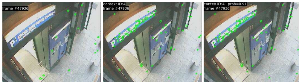
Figure 6.8: Illustration of the noise sensitivity of a poorly trained background model.
