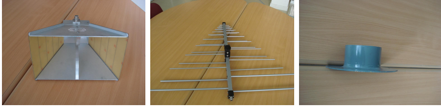
Figure 2.25: A snapshot of horn, log-periodic and CMA
