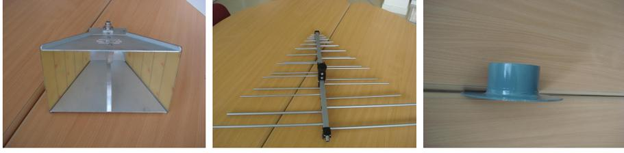
Figure 2.25: A snapshot of horn, log-periodic and CMA
