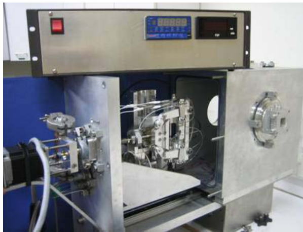
Fig. II.25. TSAXS in vacuum chamber and TSAXS control module
