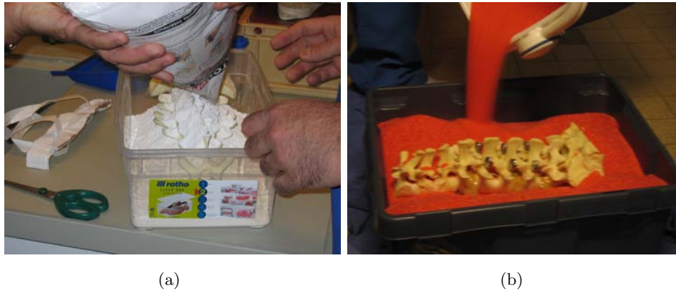
Figure 3.10: Phantom preparation (a) first emulation using chalk powder, (b) Third emulation using synthetic granules
