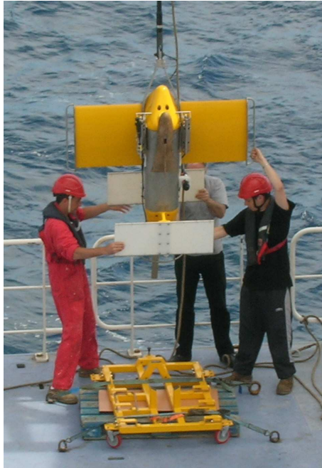
Figure 2.1: A picture of the Seasoar used onboard MOUTON 2007 survey. Towed behind the ship at 8 knots, it measures conductivity (salinity), temperature and pressure along a sinusoidal route in the water column.
