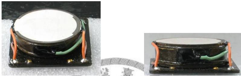
Figure 5-25. Pictures of the stacked disk-type piezoelectric transformer operating in radial mode
