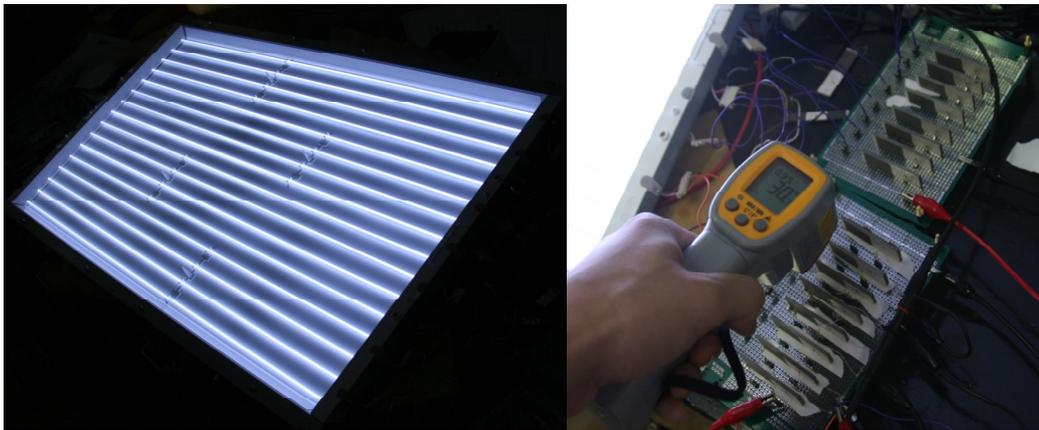
Figure 4-12. The piezoelectric transformer based inverter for commercial 32'' LCDTV backlight
