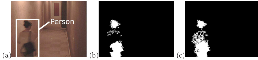
Figure 6.29: The detection results when the controller tunes the chromaticity threshold Th of our background subtraction algorithm. Image (a) is the original image sample at frame 29. Image (b) is the sample of detection results of EGMM with the initial value Th = 10 . This time, EGMM has not updated the chromaticity threshold yet because it has not collected enough data. Figure (c) shows the detection results of EGMM with the help of the controller to tune the parameter Th at frame 29. With this tuned Th value, EGMM can detect nearly the whole person.
