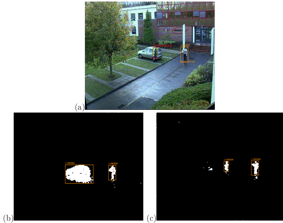
Figure 5.8: The effectiveness of managing stationary objects of interest. Figure (a) shows the original image of the video. In this video the car enters the scene then stops. After that, a person gets out of the car and enter the building. If we want to always detect the car even when it stops, we can request the background subtraction algorithm not to update the region corresponding to the car. However, with this solution, we cannot detect the person as illustrated in figure (b). Figure (c) shows the effectiveness of the controller in managing stationary objects, the background subtraction algorithm can detect the person when the car has stopped moving.
