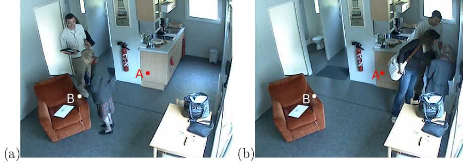
Figure 4.9: Problem of HSV color space to detect shadow. Figure (a) shows the scene in which there is no shadow at pixel A . The H value of pixel A in HSV color space is 180. Figure (b) shows the scene when there is a shadow over point A . This time, the H value of pixel A in the HSV color space is 96 which is very different from the original value (180). Therefore shadow detection algorithms using HSV color space have difficulties in distinguishing shadow from objects of interest.
