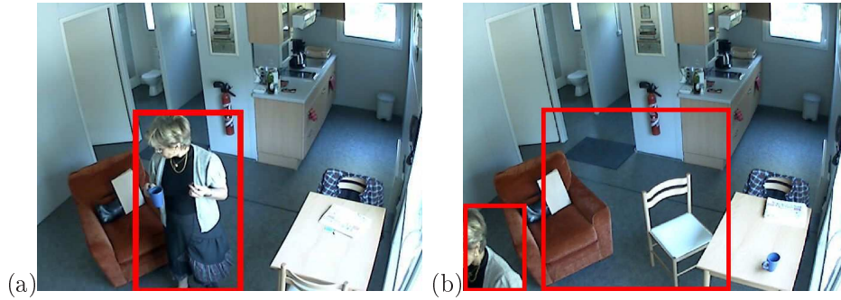
Figure 6.22: This figure illustrates the error due to not verifying the classification results. In figure (a), the original place of the chair is at the lower right corner of the image. Then, the chair is moved to the center of the image as illustrated in figure (b). Because the classification task classifies the chair blob as a person blob, the algorithm EGMM_1 does not update the region of the chair blob. Consequently, the chair blob stays in the detection results for a long time.
