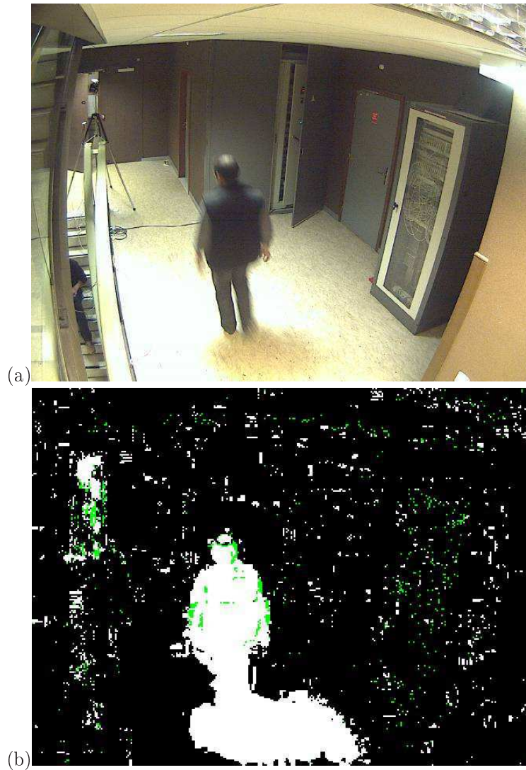
Figure 4.25: Shadow in the region with saturated illumination. Figure (a) shows the scene in which the illumination on the floor is saturated. Therefore, the camera cannot observe the texture and the chromaticity of the floor. Figure (b) shows the detection results of the background subtraction algorithm together with the shadow / highlight removal algorithm using texture and chromaticity. This algorithm fails to remove the shadow in the saturated region from the detection results.
