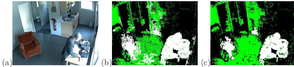
Figure 6.13: This figure illustrates the effectiveness of estimating parameter a_R , a_B . Image (a) shows the frame 1276. Without automatic estimating a_R, a_B , the chromaticity constraint NC using default values of white balance parameters ( a_R = a_B = 0 ) cannot detect the shadow on the floor, on the armchairs and on the wall (image (b)). On the same video, using the method to estimate a_R , a_B , after the last update of a_R , a_B at frame 1275, the chromaticity constraint NC can detect the shadow on the floor, on the armchair, and reduce the noise on the wall (image (c)). The green regions correspond to the detected shadow. The white regions correspond to the foreground region.
