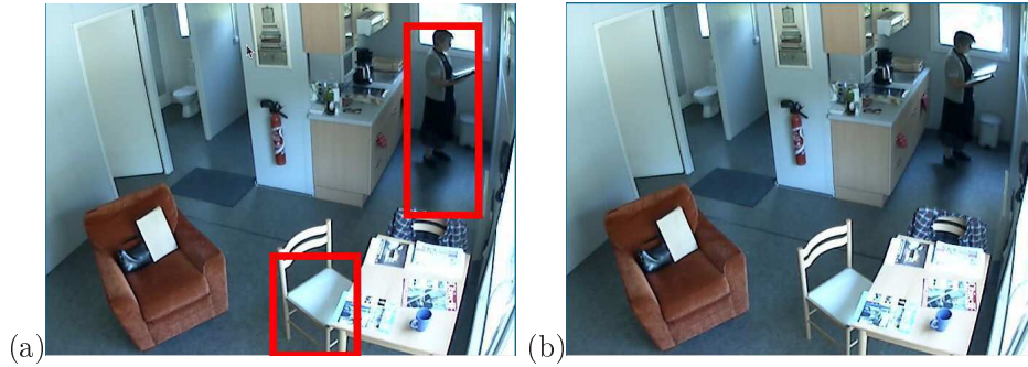
Figure 6.24: Image (a) illustrates the error of EGMM_1 which does not verify detected person blob. Without verification, EGMM_1 considers that the chair blob is a real person and it does not update this region. Image (b) illustrate the error of EGMM_2 . EGMM_2 can recognize that the chair is not a real person so it absorbs the chair in the detection result. However, because the person blob also includes the strong shadow region of this person which does not satisfy the edge condition, the people detector misclassifies this blob as an unknown blob.
