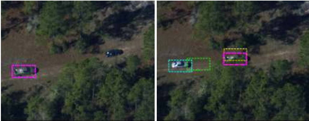
Figure 2.1: Example on a video from a tracking benchmark [CZT05]. An object of interest is defined on the first frame, and we search for the new position in a frame later in the video: purple algorithm is our method presented in chapter 6. Difficulties: the object is only partially visible, may not have the same size, may have changed appearance . . .
