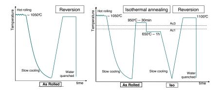
Figure 3.4: Heat treatments performed on the 16MnCr5+Nb steel. Treatments on the Iso state are performed without the cold forming.
