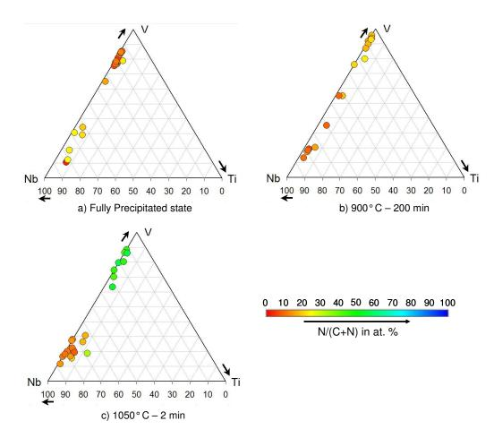
Figure 2.15: Ternary diagrams showing the chemical composition of each analyzed precipitates for: a) the Fully Precipitated state, b) the 900°C - 200 minutes state and c) the 1050°C - 2 minutes state. A nitrogen content scale is presented on the figure, from red for pure carbides to blue for pure nitrides. We can see that Nbrich precipitates are mainly rich in carbon, while V-rich particles are rich in both carbon and nitrogen.
