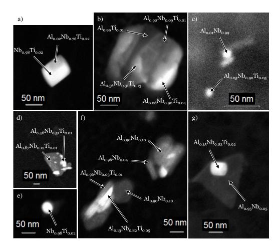
Figure 3.15: STEM-HAADF micrographs of precipitates extracted from the  $16MnCr_5+Nb$  alloy on carbon replicas : a) As Rolled state; b) As a); c) Iso state; d) As c); e) Iso state +  $1100^{\circ}$ C; f) As e); g) As Rolled state +  $1100^{\circ}$ C. Chemical compositions written on micrographs is obtained by EDX.
