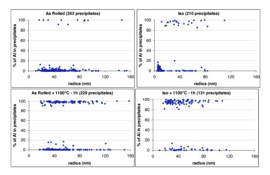
Figure 3.21: Comparison between the precipitate chemical composition and their size a) As Rolled state; b) Iso state; c) As Rolled state  $+ 1100^{\circ}$ C; d) Iso state  $+ 1100^{\circ}$ C.
