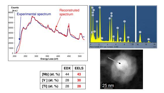
Figure 1.14: Experimental EELS spectrum of a carbonitride (Nb,V,Ti)(C,N) from the As Rolled state of the  $60SiCrV_7+Nb$  steel. The reconstructed spectrum shows a good fit. The spectrum obtained by EDX allows us to view the metallic elements but it is impossible to quantify the nitrogen and carbon. The table shows the results of the EDX and EELS analysis for metallic elements. We note that both methods give very close values.
