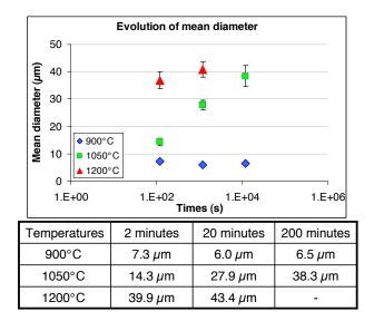
Figure 3.12: Mean grain diameter for all heat treatments. There is no significant difference at 900°C whereas we observe an increase of the mean grain diameter at 1050°C and 1200°C due to the presence of abnormal large grains, that can be seen on figure 3.13.
