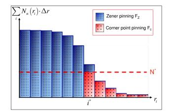
Figure 4.12: Integration of the size distribution (starting from the end). In this graph, the red part on the right corresponds to particles, which pin "corner points", and the blue part on the left corresponds to particles, which have a Zener-type pinning pressure. The class i\* is divided into two parts: Zener and corner points pinning types.
