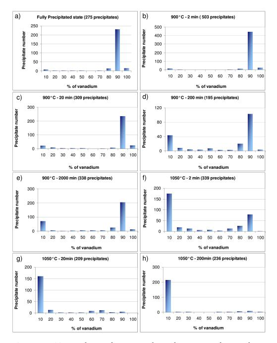
Figure 2.12: Time evolution of precipitate chemical composition for several temperatures (EDX analysis).
