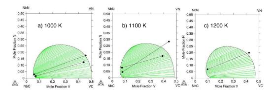
Figure 2.13: The calculated miscibility gap from in the Nb-V-C-N system at a) 1000 K, b) 1100 K and c) 1200 K, in equilibrium Fe-base matrix [Frisk 08], compared with experimental results (darks dots and lines) from the work of [Inoue 01].
