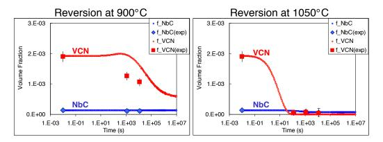
Figure 2.25: Model prediction for the volume fraction evolution during reversion at 900° and 1050° C. Experimental results are shown for  $VC_xN_y$  and NbC precipitates.
