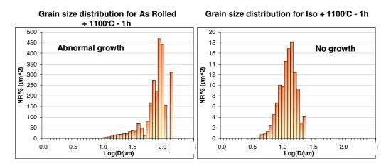
Figure 4.7: Experimental grain size distributions for both As Rolled and Iso state after a treatment at 1100°C during 1 hour. The kind of grain growth is as indicated on both graphs.
