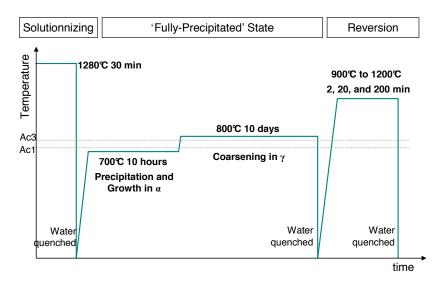
Figure 4.1: Heat treatments for the FeVNbCN alloy.
