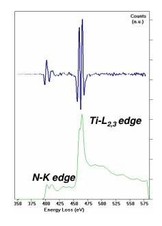
Figure 1.9: *EELS spectrum of a* TiN sample and its second derivative. Peaks corresponding to the N-K and Ti- $L_{2.3}$  edges are exacerbated by the second derivative (this treatment was performed on an experimental spectrum acquired on a TiN precipitate [Sennour 02]).
