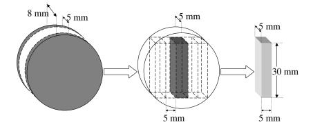
Figure 2.3: Samples preparation for the FeVNbCN alloy. Grey parts are removed to avoid decarburized and segregated areas.
