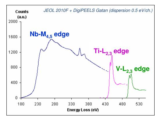
Figure 1.11: Ionization edges of the elements Nb, V and Ti. Each spectrum is normalized to one atom.
