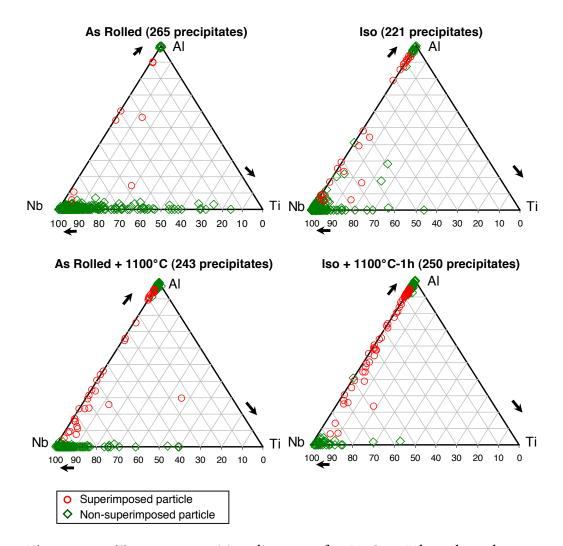
Figure 3.16: Ternary composition diagrams of 16MnCr5+Nb grade steel states. Red symbols (circles) represents Nb-rich precipitates superimposed to AlN. Green symbols (diamonds) correspond to non-superimposed precipitates.
