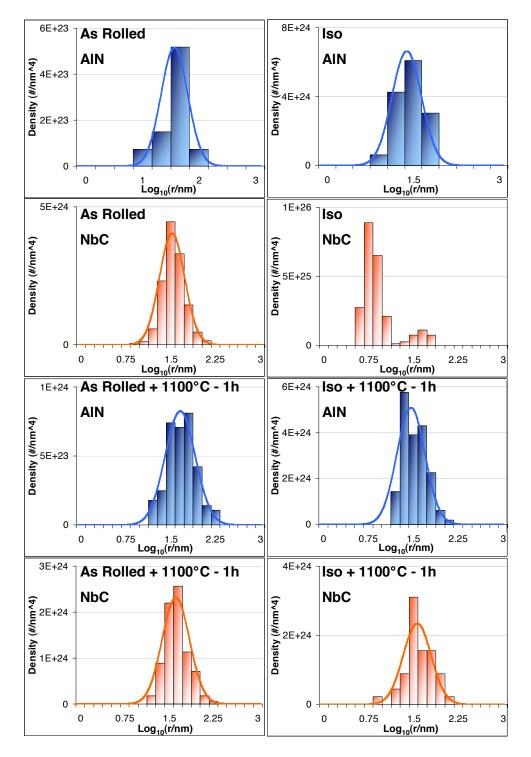
Figure 3.19: Density distribution of AlN and NbC for the As Rolled state, the Iso state, the As Rolled state  $+ 1100^{\circ}$ C and the Iso sate  $+ 1100^{\circ}$ C. Distributions are normalized in order to get the correct volume fraction and are fitted by a Lognormal when it is possible.
