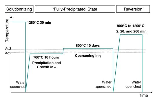
Figure 2.2: Thermal cycle performed on the model alloy FeVNbCN.
