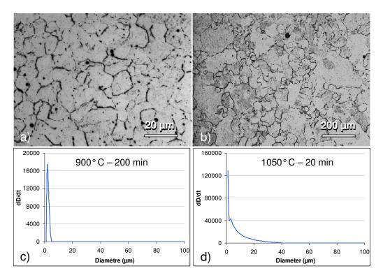
Figure 4.10: Comparison between experimental results and the model of Bréchet and Militzer. a and b: Optical micrographies obtain after Béchet-Beaujard etching for FeVNbCN alloy treated at 900°C during 200 minutes and 1050°C during 20 minutes respectively; c and d: growth rates obtained for these treatment respectively. As it can be seen, both calculation and experiments are not in perfect agreement, especially for the treatment at 1050°C.
