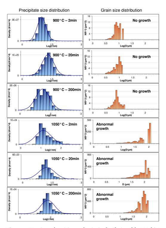
Figure 4.3: Experimental precipitate and grain size distribution of the FeVNbCN model alloy. The kind of grain growth is indicated on the graphs of grain size distributions.
