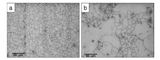
Figure 3.2: Optical micrographies of a microalloying steel after a Bechet-Beaujard etching. a) Normal grain growth or zero growth microstructure with an homogeneous grain size; b) AGG microstructure.
