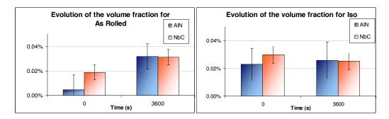
Figure 3.18: Evolution of volume fraction of AlN and NbC before and after 1 hour at  $1100^{\circ}$ C
