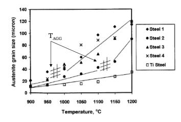
Figure 3.1: Mean austenitic grain size evolution with the increase of austenitizing temperature for Al-V-N and Al-V-Ti-N microalloyed steels. The curve highlights three steps during the growth: the zero growth, the abnormal grain growth and the normal grain growth.  $T_{AGG}$  represents the transition temperature zero growth/abnormal grain growth [Gao 98].
