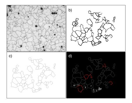
Figure 3.7: Example of a tracing treatment to obtain the grain size distribution. a) Optical micrograph; b) Digitized and thresholded tracing of the micrograph a); c) Skeletonizing of the tracing; d) Colour are reversed to use the ImageTool software. Grain in red, which are not closed, are not counted.
