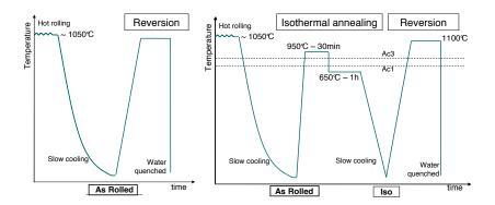
Figure 4.2: Heat treatments for the 16MnCr5+Nb steel.
