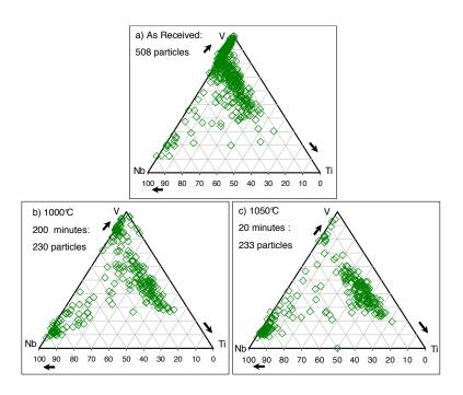
Figure 2.9: Particles chemistry evolution obtain by EDX in TEM. a) "As Rolled" state: many V-rich particles; b) "200 minutes at 1000° C" state and c) "20 minutes at 1050° C" state: particles are richer in niobium and titanium due to the solutionizing of vanadium. Results from the D. Acevedo's PhD and from the further study performed during this work are reassembled on the figure.
