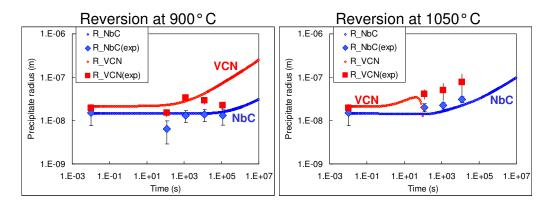
Figure 2.26: Model prediction for the mean radius evolution during reversion at 900° and 1050° C. Experimental results are shown on the figure for  $VC_xN_y$  and NbC precipitates.
