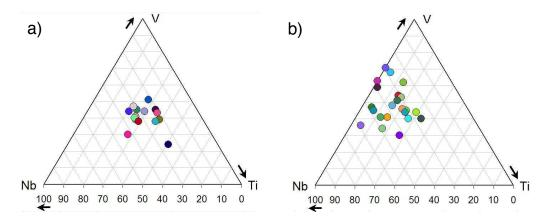
Figure 1.17: Graphical representation of results obtained by EELS for all treated spectra. a) Analysis performed in the core of precipitates and b) in the shell. There is a clear titanium enrichment in cores of precipitates.
