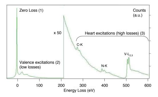
Figure 1.3: EELS spectrum obtained on a vanadium carbonitride.
