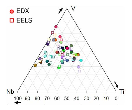
Figure 1.15: Graphical representation of results obtained by EDX and EELS analysis for all treated spectra of the 60SiCrV7+Nb steel at the As Rolled state. The ternary diagram allows to view the quantities of metallic elements in the carbonitrides. Each colour represents a test. Results show that values obtained by EDX are very close to those obtained by EELS (each square is associated with the disk of same colour).
