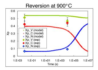
Figure 2.27: Model prediction for the  $VC_xN_y$  composition evolution during reversion at 900°. Experimental results obtain by EELS are shown on the figure.
