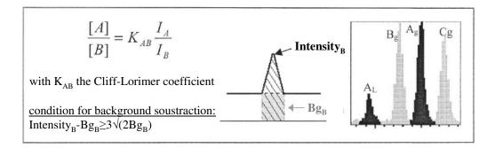
Figure 2.5: Principle and limit of the EDX detection.
