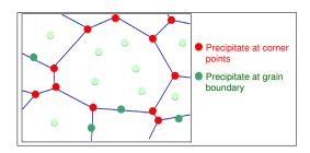
Figure 4.8: Schematic representation of different location types for precipitates in a polycrystalline material. Spheres in red represent precipitates, which pin corner points, and green ones are for precipitates pinning grain boundaries.
