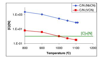
Figure 2.17: Thermo-Calc calculation of the C/N ratio in vanadium and niobium particles [TCFE 5 05].
