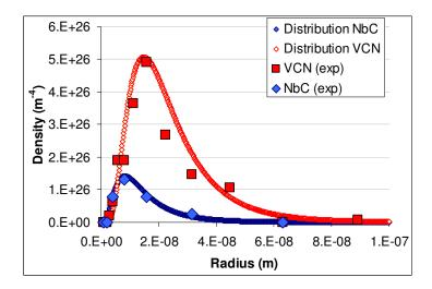
Figure 2.24: Initial precipitate size distributions of NbC and  $VC_xN_y$  used for the model. These distributions are normalized in order to obtain the correct volume fraction.
