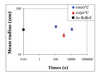
Figure 2.10: Mean radius measured for three states using HAADF in STEM micrographies. Results from D. Acevedo's PhD have been completed by the analysis of a few hundreds additional particles.
