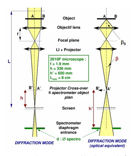
JEOL 2010F microscope, the factor h/h' was previously measured to 0.56.
