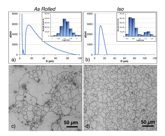
Figure 4.17: Comparison between prediction of the model and experimental observations. *a*) and *b*): Prediction of the model for As Rolled and Iso states respectively. *c*) and *d*): Optical micrographies of As Rolled and Iso states after a treatment at 1100°C during 1 hour respectively.
