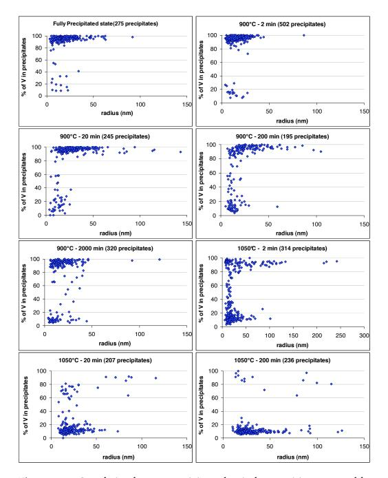
Figure 2.19: Correlation between precipitate chemical composition measured by EDX and their size measured on HAADF images for all investigated states. We observe an evolution of the particle sizes but also of the chemistry: the higher the temperature, the higher the ratio of niobium particles.
