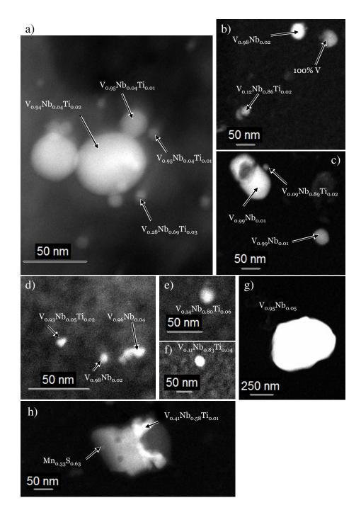
Figure 2.11: HAADF in STEM micrographies of microalloyed steel FeVNbCN for states: a) Fully Precipitated State; b)  $900^{\circ}$ C - 20 minutes; c)  $900^{\circ}$ C - 200 minutes; d) and e)  $1050^{\circ}$ C - 2 minutes; f) and g)  $1050^{\circ}$ C - 20 minutes; h)  $1200^{\circ}$ C - 2 minutes. Precipitate chemical composition shown on the figure were obtained by EDX.
