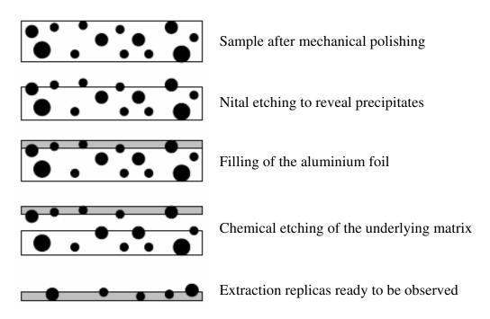
Figure A.2: Schematic procedure of the preparation of aluminium replicas.
