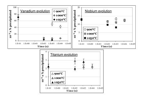
Figure 2.7: Evolution of vanadium, niobium and titanium precipitated mass fractions during heat treatment at 900°C, 1000°C and 1050°C for the 60SiCrV7+Nb industrial steel. Time O.1 s corresponds to the As Rolled state.
