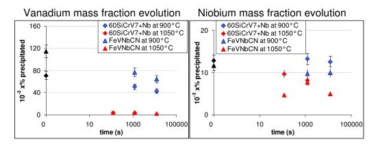
Figure 2.22: Evolution of mass fraction for the 60SiCrV7+Nb industrial steel and for the FeVNbCN model alloy of a): Vanadium and b) Niobium.
