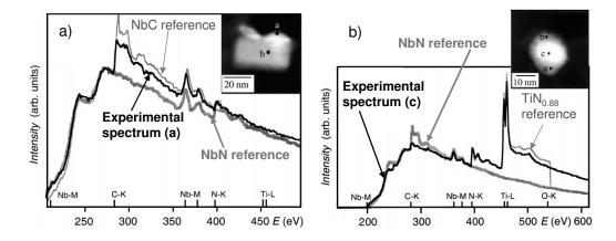
Figure 1.5: Adjustment of experimental spectra with a linear combination of standards NbN, NbC and  $TiN_{0.88}$ . a) Spectrum of a precipitate shell with no titanium and nitrogen, b) Spectrum of a precipitate core, with nitrogen and titanium. There appears to be an enrichment of Ti and N in the core of particles [Craven 00a].
