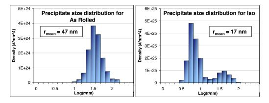
Figure 4.5: Experimental precipitate size distributions for the As Rolled and Iso states in the industrial steel 16MnCr5+Nb.
