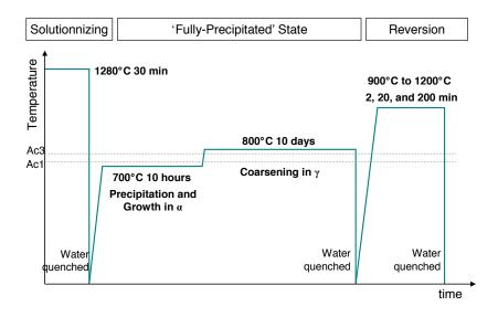
Figure 3.6: *Heat treatments for the FeVNbCN alloy.*
