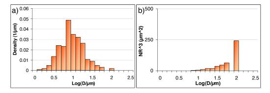
Figure 3.10: *a)* Number density and *b)* grain volume density of a same state. With the grain volume density, we clearly observe the presence of small and large grains, while the number density presents Log-normal distribution.
