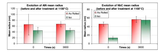
Figure 3.20: Evolution of the particle mean radius during isothermal reversion at  $1100^{\circ}$ C in 16MnCr5+Nb alloy on As Rolled and Iso states. Values of mean radium have been determined from size distributions measured on STEM in SEM images; the error bar reflects the amount of particles observed.
