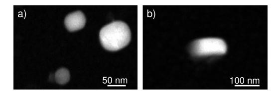
Figure 2.6: HAADF micrographies of particles of the FeVNbCN alloy on an aluminium film: a) Spherical precipitates of the state treated 20 minutes at 900°C; b) Elongated precipitate of the state treated 200 minutes at 1050°C.
