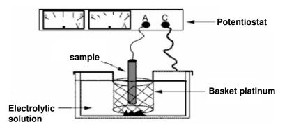
Figure B.1: Scheme of the electrolytic dissolution system.
