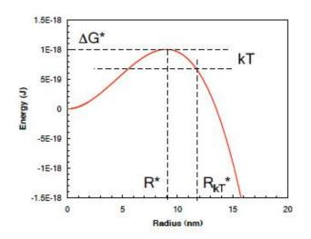
Figure 2.23: Schematic representation of the nucleation free energy variation versus precipitate radius.
