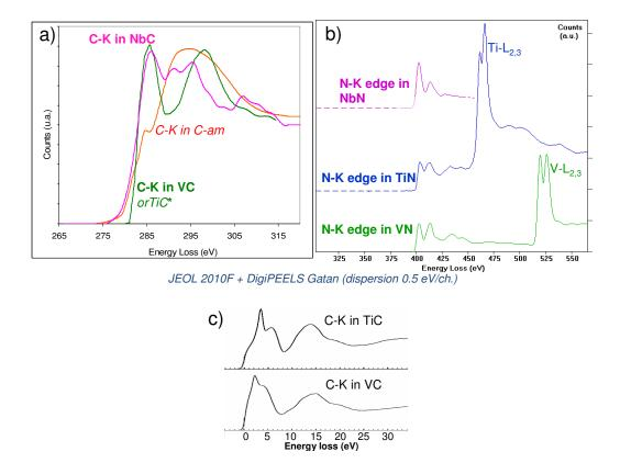
Figure 1.12: Ionization edge of non-metallic elements. a) C-K edge in NbC, VC (or TiC) and C-amorphous. b) N-K edge in NbN, VN and TiN. c) C-K edge in VC and TiC [Scott 01]. We note that both edges are quite similar, which is why we had not differentiated.
