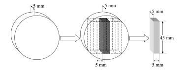
Figure 3.5: Samples preparation of the 16MnCr5+Nb alloy. Grey parts are removed to avoid decarburized and segregated areas.
