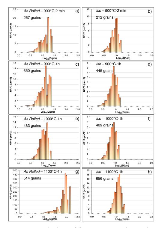
Figure 3.9: Grain size distributions of all reversion treatments. There no evolution for the Iso state, where as we observe an abnormal grain growth for the treatment of 1 hour at 1100°C performed on the As Rolled state.
