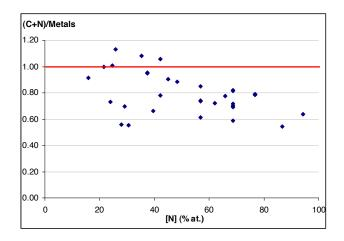
Figure 1.16: Results obtained by EELS for the quantification of carbon and nitrogen. The graph shows the percentage of nitrogen in precipitates and the stoichiometry particles. We can see that most of the precipitates are sub-stoichiometric (the stoichiometry is represented by the red line).
