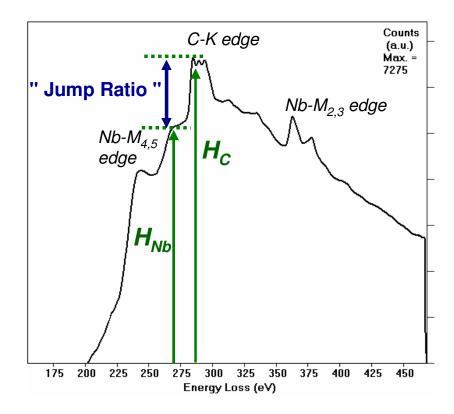
Figure 1.6: Carbon "Jump Ratio" of an EELS spectrum obtained from a bulk Nb<sub>6</sub>C<sub>5</sub> [Courtois 06].
