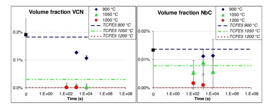
Figure 2.20: Evolution of volume fraction of a): VCN and b) NbC. Thermodynamic equilibria calculated with the ThermoCalc software [TCFE 5 05] are given on the figure.
