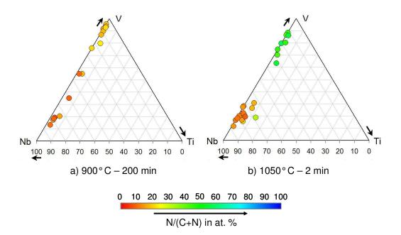
Figure 3.23: Ternary diagrams showing the chemical composition of each analyzed precipitate category for: a) the 900°C - 200 minutes state and b) the 1050°C - 2 minutes state. A nitrogen content scale is presented on the figure, showing that Nb-rich precipitates are carbides while V-rich particles are carbonitrides.
