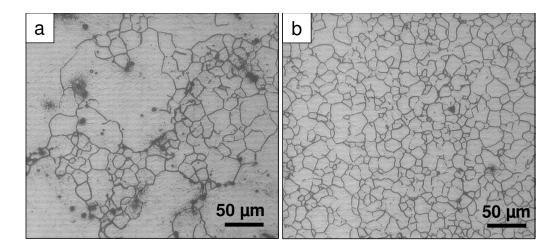
Figure 3.8: Micrographies of the  $16MnCr_5+Nb$  alloy after a treatment of 1 hour at  $1100^{\circ}C$  for a) As Rolled state and b) Iso state. We observe an abnormal grain growth in the case of the As Rolled state but not for the Iso state. Thus we have a better grain growth control for the Iso state. Note that initial grain sizes (900°C -2 minutes) are similar for both As Rolled and Iso states.
