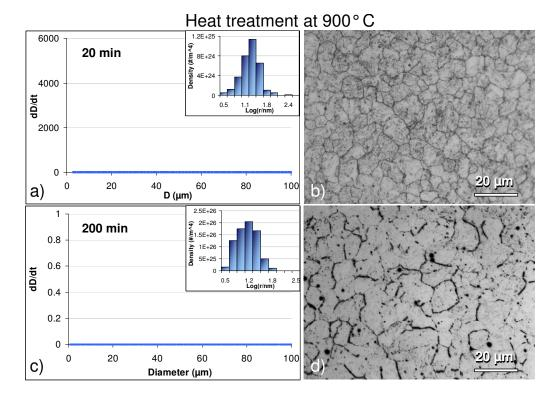
Figure 4.15: Comparison between experimental results and the model for heat treatments at 900°C. a and c: Growth rate obtained after 20 minutes and 200 minutes; b and d: Optical micrographs obtained after Béchet-Beaujard etching for these treatments. There is a good agreement between the predictions of the model and the experimental results.
