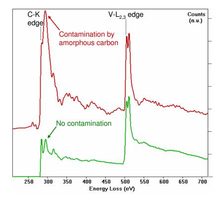
Figure 1.1: Two EELS spectra from vanadium carbides in a thin foil. The first one (green curve) does not show amorphous carbon while the second one (red curve) shows a massive contamination due to carbon pollution. The presence of amorphous carbon makes the determination of the exact precipitate chemistry harder.
