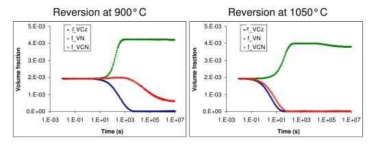
Figure 2.28: Model prediction for  $VC_z$ , VN and  $VC_xN_y$  volume fraction evolution during reversion at 900° and 1050° C.
