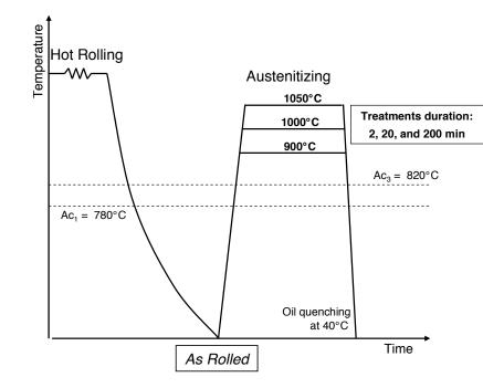
Figure 2.1: Heat treatments performed on the 60SiCrV7+Nb microalloyed steel.
