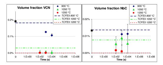
Figure 4.4: Evolution of volume fraction of a): VCN and b) NbC. Thermodynamic equilibria calculated by [TCFE5 05] are given on the figure.
