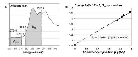
Figure 1.7: Determination of the dependence calibrated curve of "Jump ratio" versus the chemical composition C/Nb. a) Calculation of areas  $A_{\rm Nb}$  and  $A_{\rm C}$  to determine the "Jump Ratio"; b) calibration curve of the "Jump ratio" on the carbon K edge citeCourtoiso6.
