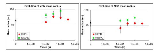
Figure 2.18: Evolution of VCN and NbC mean radius with treatment duration and temperature in the FeVNbCN model alloy. Precipitates with more than 50% of vanadium are considered as VCN. Error bars take into account the quantity of observed particles.
