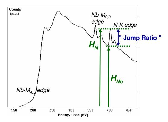
Figure 1.8: Nitrogen "Jump Ratio" of an EELS spectrum obtained from a bulk NbN /Courtois 06].
