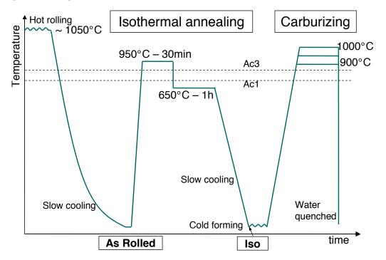
Figure 3.3: Industrial thermomechanical treatment performed on the  $16MnCr_5+Nb$  steel. After hot forming, an isothermal annealing followed by a cold forming is performed on the steel. This industrial treatment is finished by a carburizing treatment.
