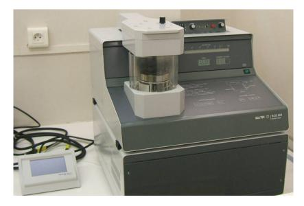
Figure A.1: Secondary vacuum metallizing SCD 500 BALTEC
