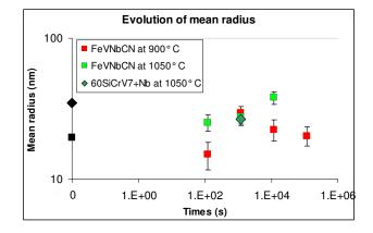
Figure 2.21: Evolution of the precipitate mean radius for the FeVNbCN and the 60SiCrV7+Nb microalloyed steel.
