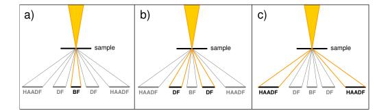
Figure 2.4: Detection principle of electron in a) Bright Field; b) Dark field and c) HAADF.
