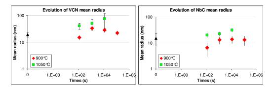
Figure 3.25: Evolution of VCN and NbC mean radius with treatment duration and temperature. Error bars take into account the quantity of observed particles.
