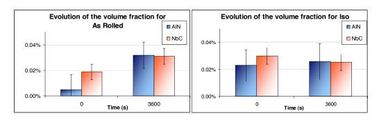
Figure 4.6: Evolution of volume fraction of AlN and NbC before and after 1 hour at  $1100^{\circ}$ C
