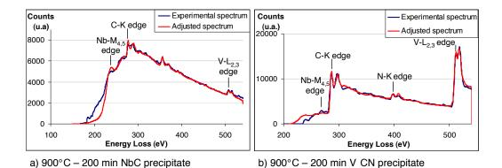
Figure 2.14: *EELS spectra from carbonitrides on aluminium replica of the FeVNbCN alloy treated 200 minutes at 900°C. a) Spectrum of niobium carbide with some vanadium; b) spectrum of vanadium carbonitride with some niobium.*
