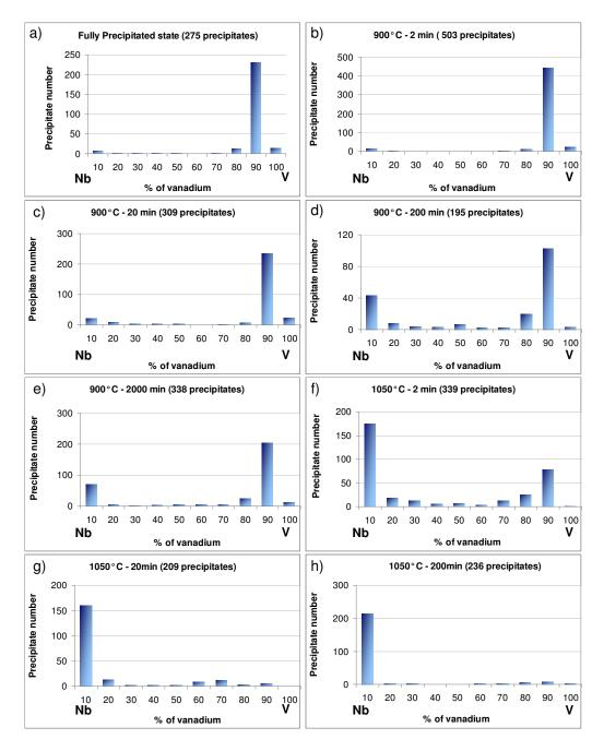
Figure 3.22: *Evolution of the precipitate chemical composition with the treatment duration and temperature.*
