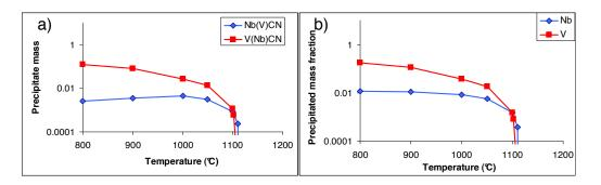
Figure 2.16: Evolution with the temperature of a) V(Nb)CN and Nb(V)CN precipitates mass and b) precipitated mass fraction of vanadium and niobium in the FeVNbCN model alloy (results obtained with the Thermo-Calc software [TCFE5 05]).
