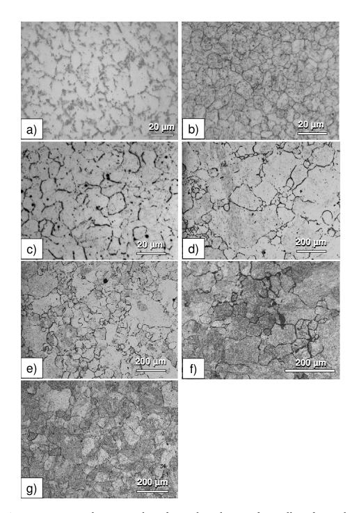
Figure 3.13: Optical micrographies obtained on the FeVNbCN alloy after Bechet-Beaujard etching for various reversion treatments: a)  $900^{\circ}$ C - 2 minutes; b)  $900^{\circ}$ C - 20 minutes; c)  $900^{\circ}$ C - 200 minutes; d)  $1050^{\circ}$ C - 2 minutes; e)  $1050^{\circ}$ C - 200 minutes; f)  $1050^{\circ}$ C - 200 minutes; g)  $1200^{\circ}$ C - 2 minutes
