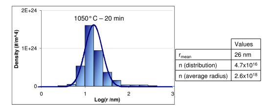
Figure 4.11: Size distribution of precipitates for FeVNbCN alloy treated at 1050°C during 20 minutes. The mean radius, and the number of precipitates (calculated from the distribution or from the average radius) are indicated on the figure.
