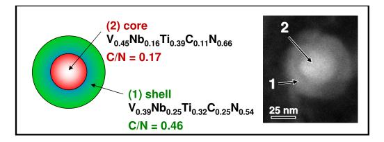
Figure 1.19: Precipitate chemical composition obtained in the core and in the shell of the precipitate after a modelling of its shape. We effectively observe an nitrogen enrichment in the core. The apparently high Ti contents of the shell is probably linked to the non-ideal shape of the particle and uncertainty of the probe position.
