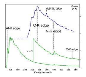
Figure 3.17: EELS spectra from a Nb-rich precipitate observed on an alumniumbased replica (upper spectrum, after background subtraction before the Nb-M edge) and from a Al-rich one (lower spectrum, after background subtraction before the Al-K edge) on a aluminium replica (16MnCr5+Nb alloy in the As Rolled state); for the latter, the zooming by a factor 5 shows the absence of significant carbon.
