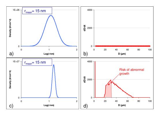
Figure 4.13: *a)* and *c):* Example of two precipitate size distribution with the same precipitate average radius and same volume fraction, but with different widths. *b)* and *d)*; Prediction of the model for these distributions. In the second case there is a risk of AGG.
