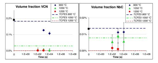
Figure 3.24: Evolution of volume fraction of a): VCN and b) NbC. Thermodynamic equilibrium calculated by [TCFE5 05] are given on the figure.
