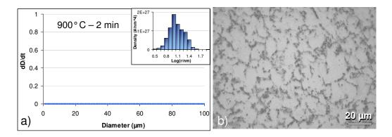
Figure 4.14: Comparison between experimental results and the model. a: Growth rate obtained for the "first state" and precipitate size distribution; b: Optical micrograph obtained after Béchet-Beaujard etching for FeVNbCN alloy treated at 900°C during 2 minutes. There is a good agreement between the model, which predicts an inhibition of the grain growth, and the experimental results.
