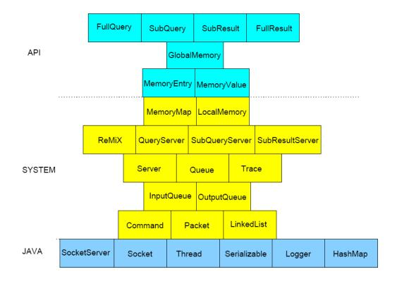
Figure 8.4: The ReMIX programming framework API [182].
