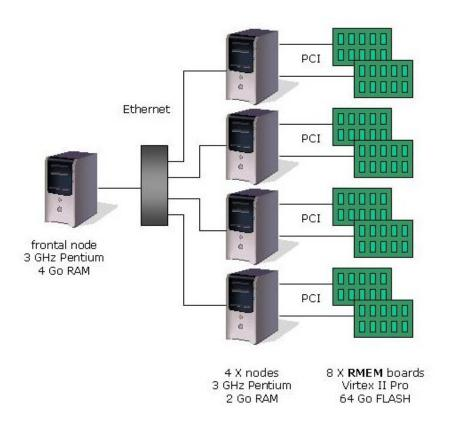
Figure 8.1: ReMIX System Architecture.
