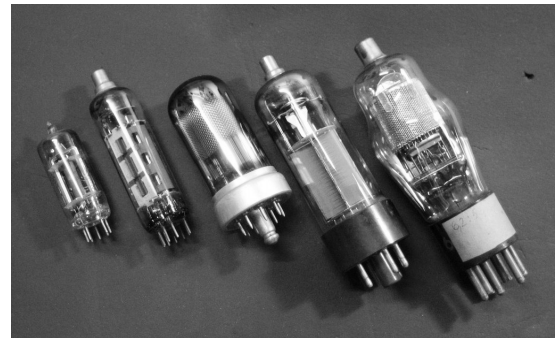
FIGURE 2: Vacuum tubes technology.
