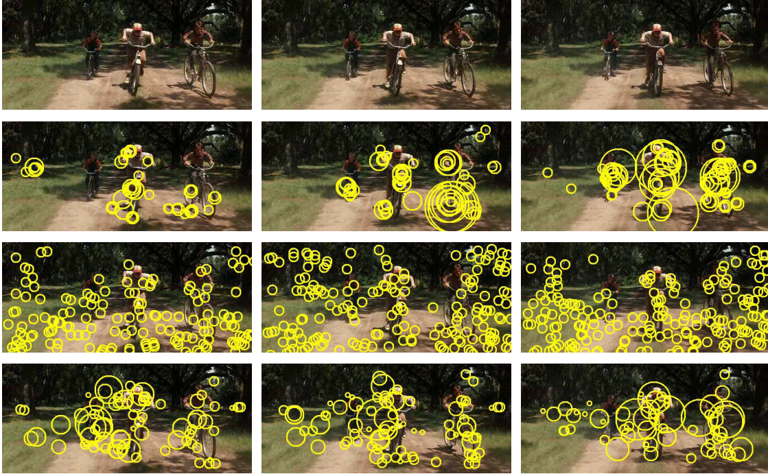
Figure 4.3: Visualization of interest points detected by the different detectors: Harris3D (second row), Gabor (third row), Hessian3D (fourth row).
