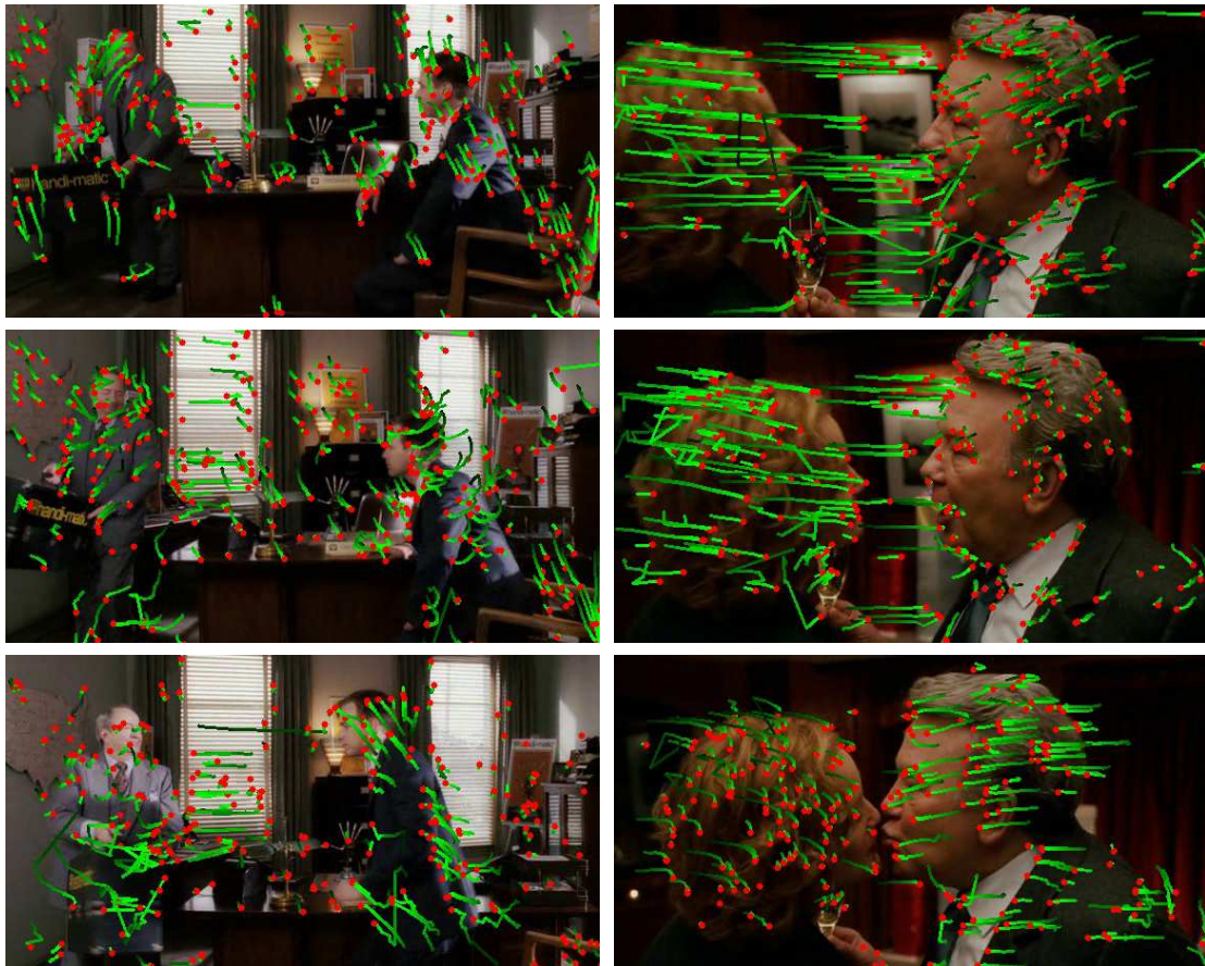
Figure 5.1: Feature trajectories for sample actions of the Hollywood2 dataset. Left column: sample sequence for the action “StandUp” where the person on the right side stands up, and the trajectories accurately capture the body motion. Right column: sample frames from a “Kiss” action. The motion of two persons approaching each other can be clearly deduced from the trajectories. Red dots indicate trajectory position in the current frame.
