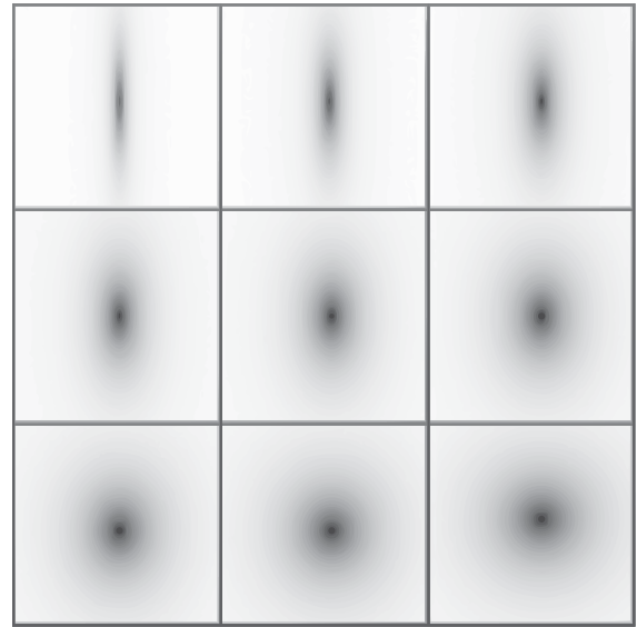
Fig. 5. Example of SEs obtained with a variation of elongations convolved with a Gaussian point spread function.
