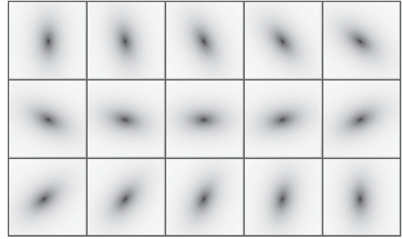
Fig. 4. Example of SEs obtained with a variation of orientations convolved with a Gaussian point spread function.
