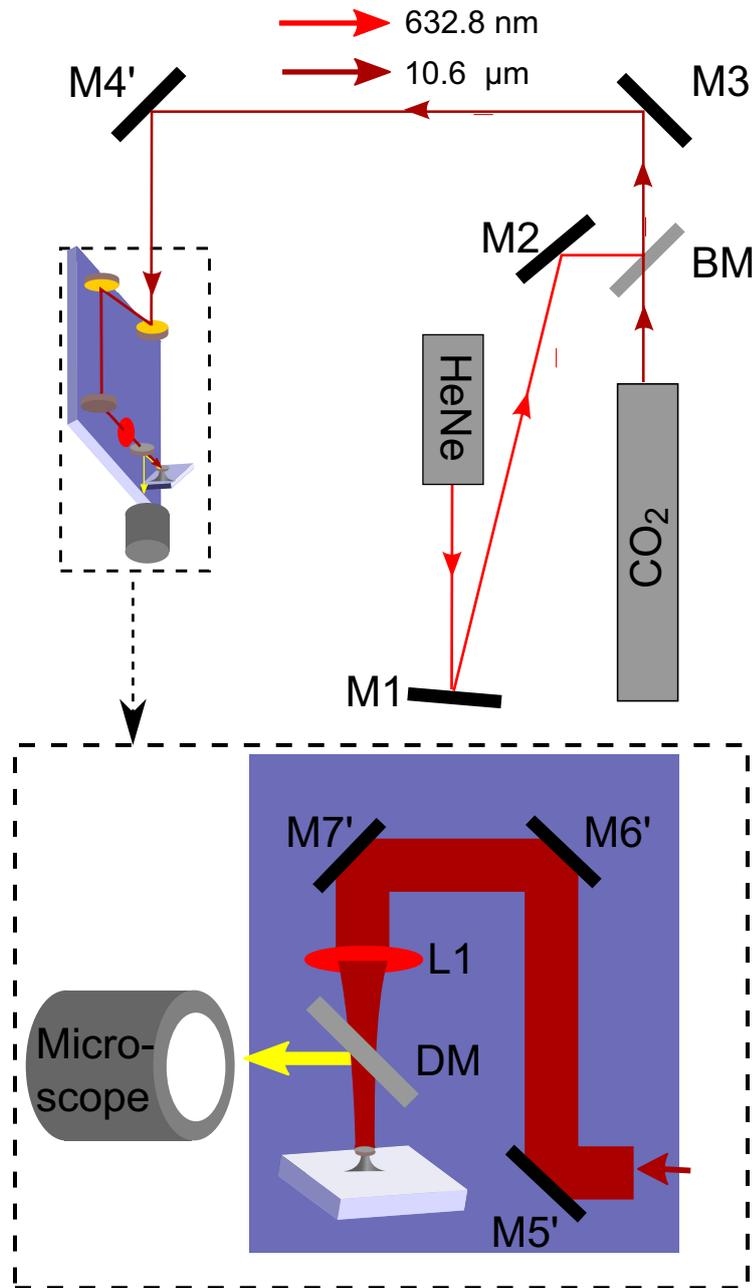
Figure 1.17: Schematic of CO<sub>2</sub> optical setup for microtoroid fabrication. M1-M3 and M4'-M7' are high reflection silicon mirrors; BM denotes beam combiner and DM dichroic mirror. Mirror L1 is a ZnSe lens. Inset shows a zoom view of the dashed line zone.
