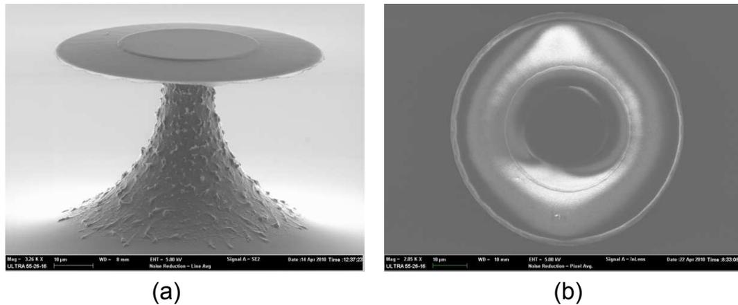
Figure 5.7: SEM graphs of a produced neodymium implanted microdisk. (a)  $76^\circ$  angle view; (b)  $90^\circ$  top view.
