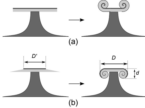
Figure 5.8: Schematics of the rolling process of microdisk under CO<sub>2</sub> irradiation. (a) Rolling up; (b) Rolling down. The gray layer denotes the ion implanted region.
