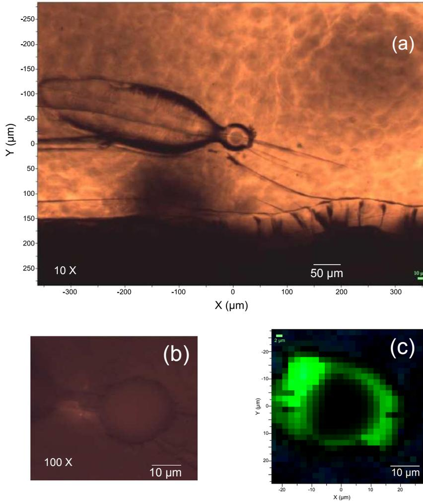
Figure 4.4: Photograph of a side-polished silica microsphere fixed on a resin: (a) X10 objective lens; (b) X100 with focus on the polished face. (c): Photoluminescence mapping image of the Nd ions on the polished face.
