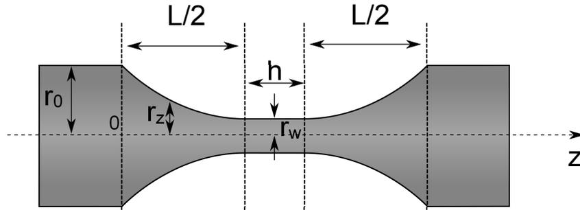
Figure 2.1: The shape of a tapered fiber.  $r_w$  is the radius of the waist;  $h$  is the hot zone length;  $L$  is the pulling length;  $r_0$  is the initial radius; the  $z = 0$  position is also defined.
