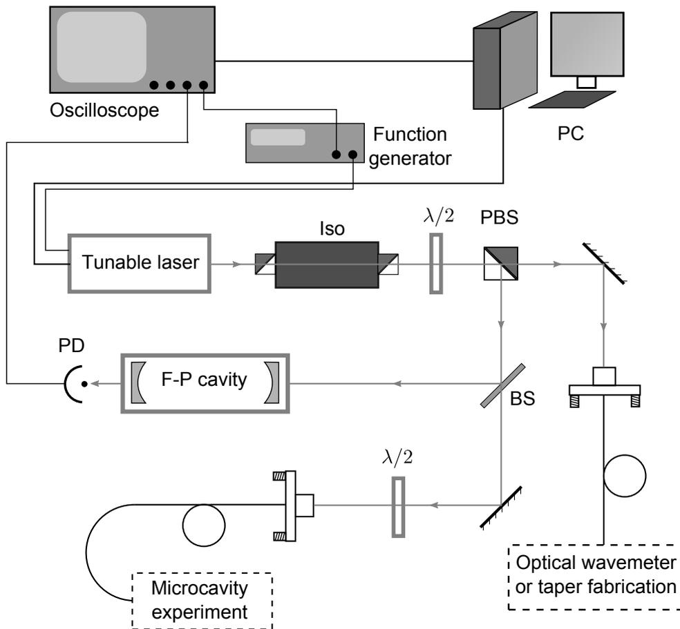
Figure 2.10: Schematic of the setup for the characterization of high  $Q$  WGMs. Iso is an optical isolator; BS is a beam splitter and PBS is a polarizing beam splitter; PD is a photodiode detector.
