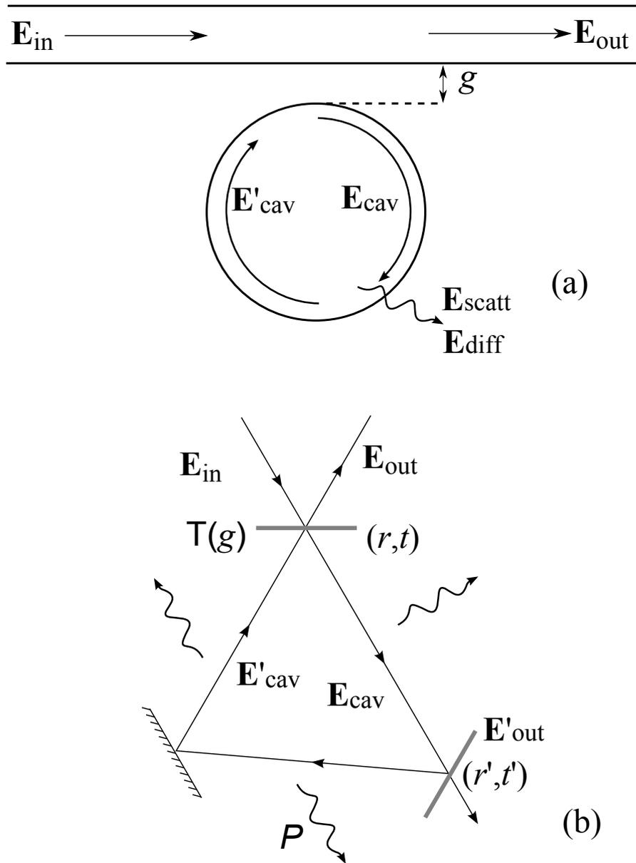
Figure 2.7: (a) Schematic of the fiber taper coupled WGM microcavity system. The gap  $g$  is the air distance between the fiber and the cavity. (b) Schematic of a Fabry Perot cavity as a model for the coupling of WGMs in a microcavity. The transmission of the input mirror is  $T(g)$ , which in the case of evanescent coupling is dependent on the gap  $g$ .  $P$  designates internal optical loss, and  $T'$  describes the other radiation losses.
