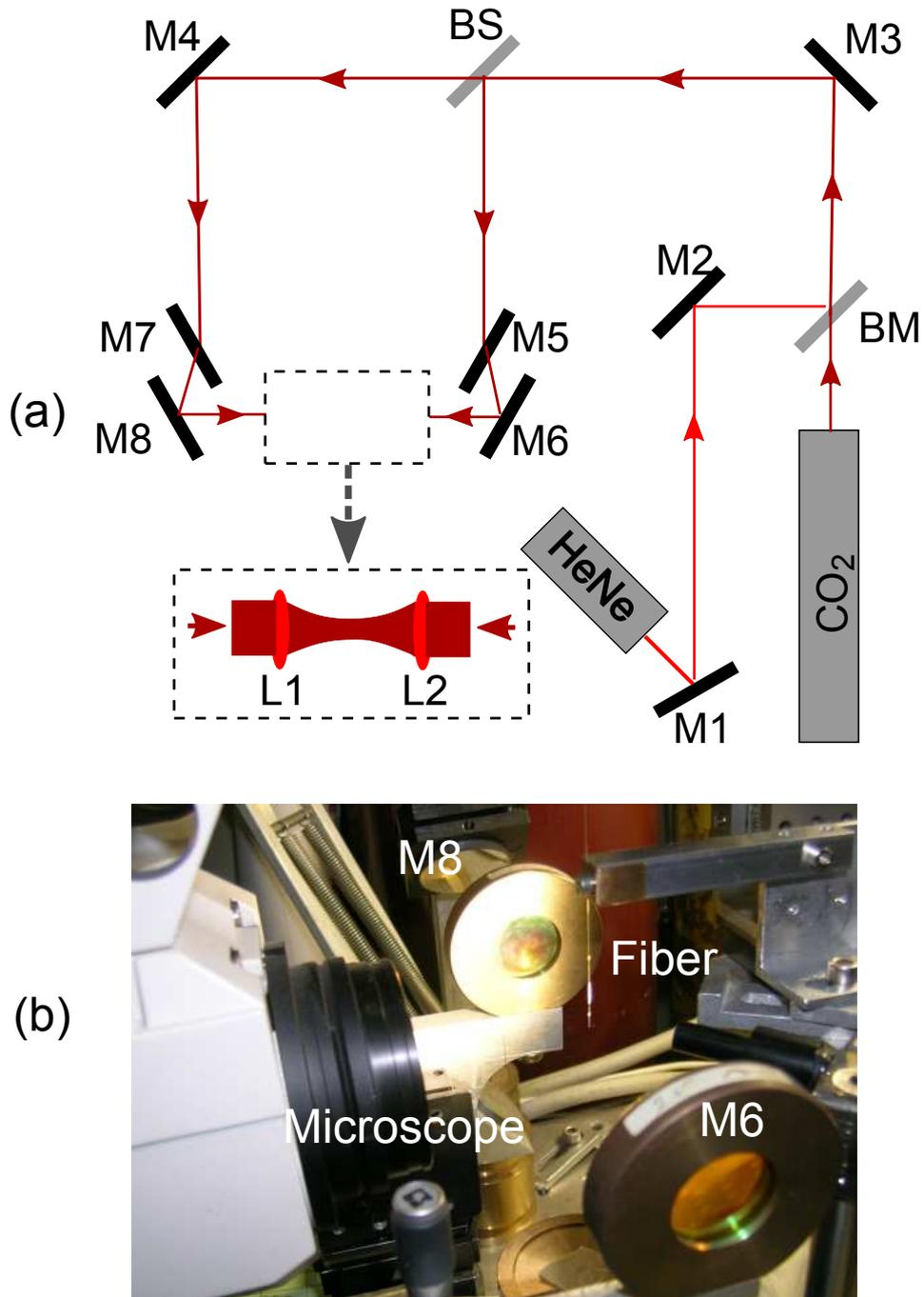
Figure 1.11: (a): Sketch of experimental setup. HeNe and CO<sub>2</sub> are the corresponding lasers. M1–M8 are reflection mirrors; BM is a beam combiner to transmit infrared light and reflect visible light; BS is a 50:50 beam splitter for CO<sub>2</sub> laser. L1 and L2 are ZnSe lenses. (b): Picture of the setup.
