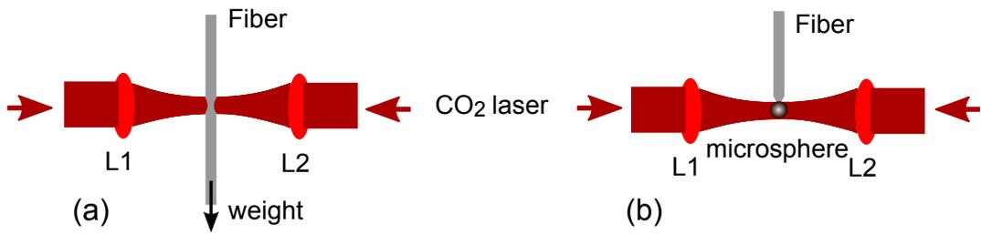
Figure 1.12: (a). Schematic of tapering process. (b). Schematic of microsphere melting.
