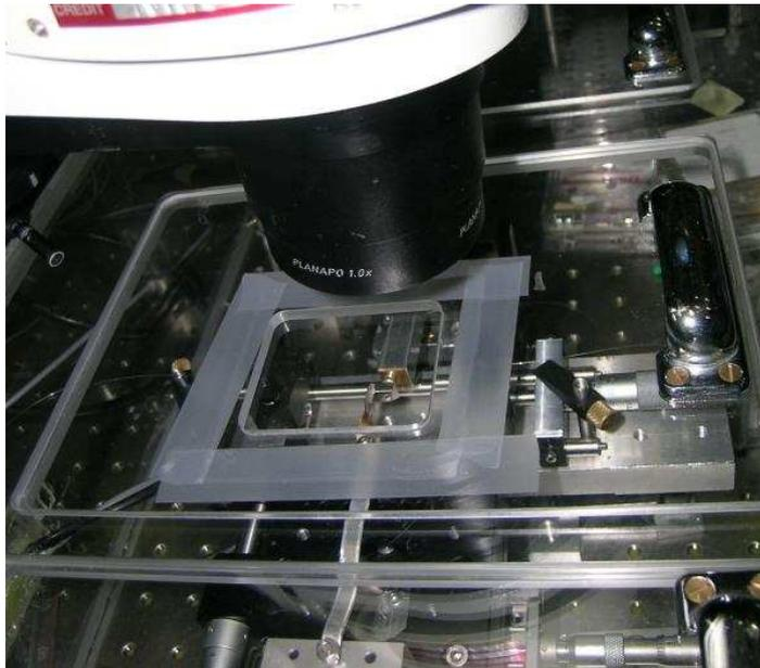
Figure 2.11: (a) Schematic of the experimental setup, with definition of the  $x, y$  axes and two rotational directions  $\alpha$  along  $x$ ,  $\beta$  along  $y$  used hereafter. S: microsphere (not to scale), T: taper, PZT: three-axis piezoelectric stage, G: goniometer, M: Compact mirror mount, PD: photodiode. (b) The picture of experimental setup.
