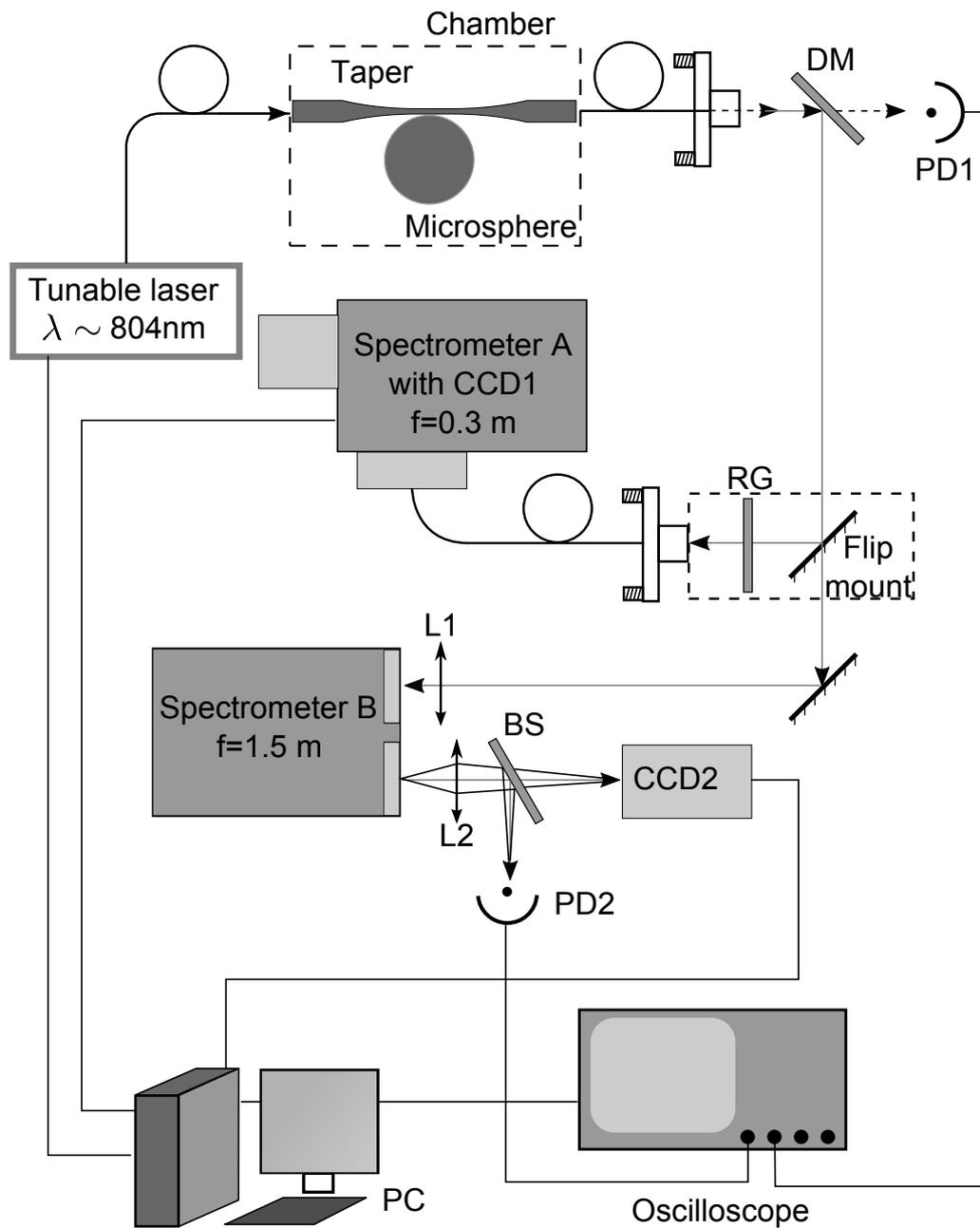
Figure 3.2: Schematic of the experimental setup for microlaser characterization. A free running diode laser ( $\lambda \sim 804\text{ nm}$ ) is used as pump source. The pump and microlaser beams in the taper throughput are denoted as dashed line and solid line, respectively. DM: dichroic mirror; RG: 850 nm long pass filter; BS: 50 : 50 beam splitter; PD1: silicon photodetector; PD2: InGaAs photodetector.
