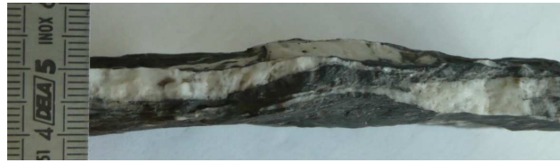
Figure 4: Profile picture of the calcite vein, C14, located at 14 m depth near the complex zone shown in Fig. 2b. The picture shows the typical thickness of the calcite vein and the complexity of the sample because of multi-layer structure.
