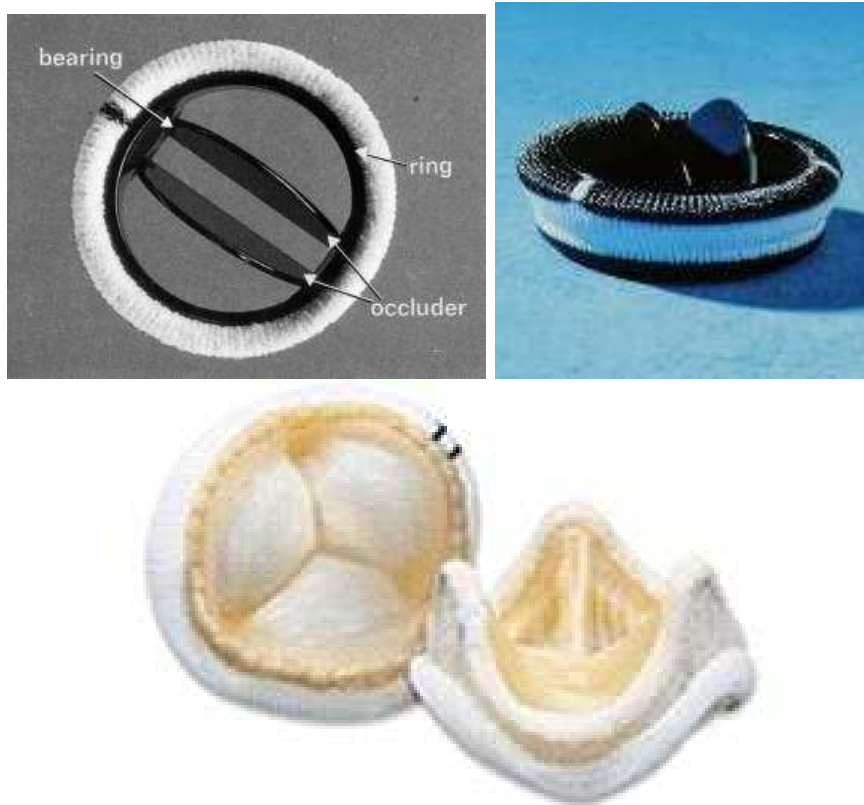
Figure 1.8: Example of two mechanical valves (top) and a tissue valve (bottom) used in heart valve surgery (from University of Birmingham and CVT Surgical Center, respectively).
