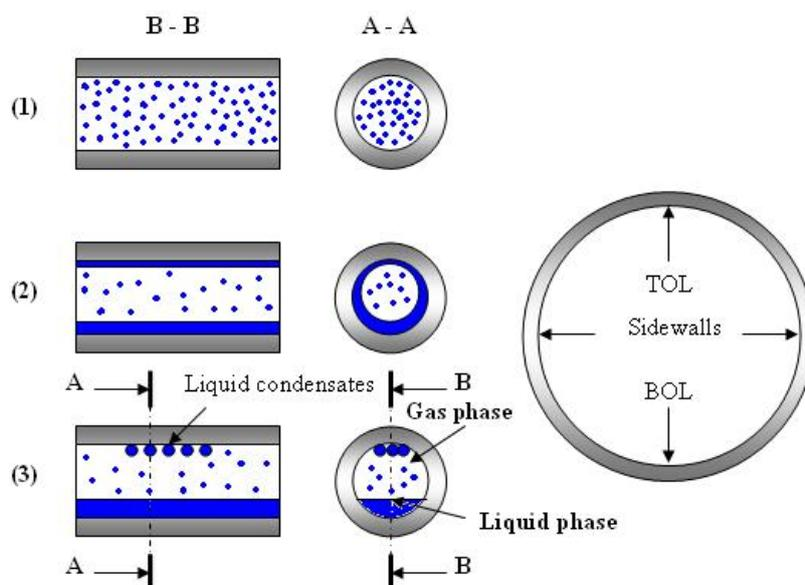
**Figure II.10.** Main patterns of gas flow encountered in wet gas pipelines. (1) Mist flow regime; (2) Annular (-mist) flow regime; (3) Stratified flow regime. This last is the most common type, particularly observed at moderate velocities of the gas flow.
