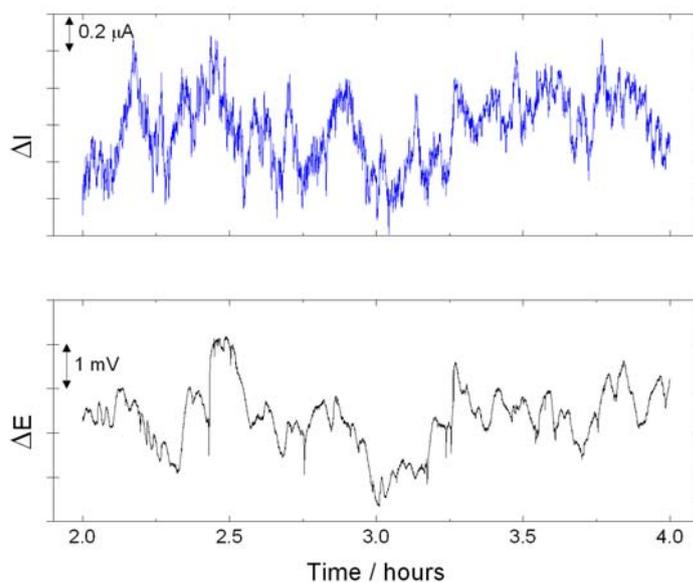
**Figure V.2.** Time records of current and potential for a freely corroding X65 electrode in 17 mM NaCl and 600 ppm HAc solution saturated with 1 bar CO<sub>2</sub> at pH 3.5 and room temperature.
