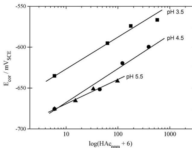
**Fig. 3.** Corrosion potential as a function of the undissociated HAC concentration at different pH values in 0.01 M NaCl saturated with 1 bar CO<sub>2</sub>. The total concentrations of acetic species were 0, 60, 180 and 600 ppm.
