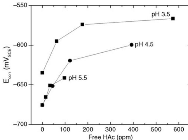
**FIGURE 6.** Variation of the corrosion potential of X65 steel with free HAc concentration at different pH values. 0.1 wt% NaCl, 1 bar CO<sub>2</sub>, room temperature.
