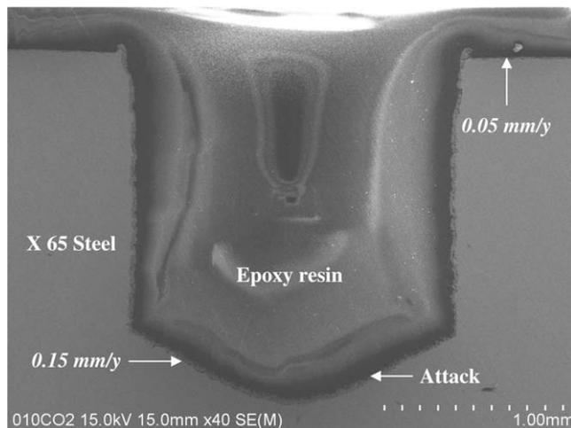
**Fig. 7.** SEM cross-section of 2 mm-depth attack on API 5L X65 sample after immersion during 3 months in 17 mM NaCl and 0 ppm HAC saturated with 1 bar CO<sub>2</sub>.
