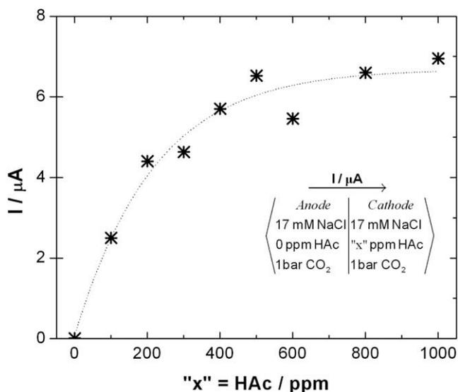
**Fig. 9.** Current flow between two identical electrodes in a split-cell composed of two identical compartments separated by a high conductivity salt bridge. One of the compartments (cathode) contained the base 17 mM NaCl aqueous solution containing "x" ppm HAC and saturated with 1 bar CO<sub>2</sub>. The other compartment (anode) was filled with HAC-free solution of 17 mM NaCl saturated with 1 bar CO<sub>2</sub>.
