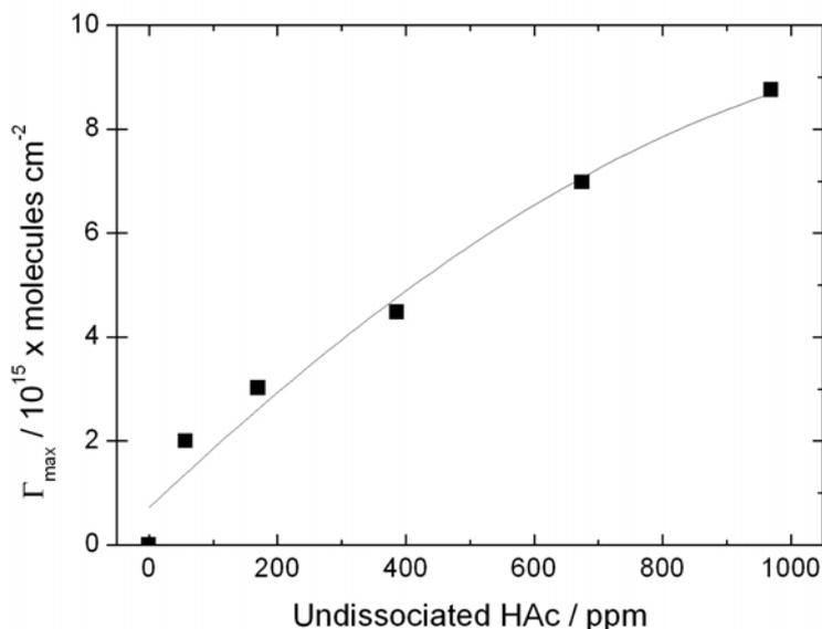
**Figure IV.16.** The dependence of the maximum surface concentration of undissociated HAC on the bulk concentration of this compound in 1 bar CO<sub>2</sub>-saturated 17 mM NaCl solutions at  $E = -600 \text{ mV}_{\text{SCE}}$ , pH 3.5, room temperature. Unstirred conditions.
