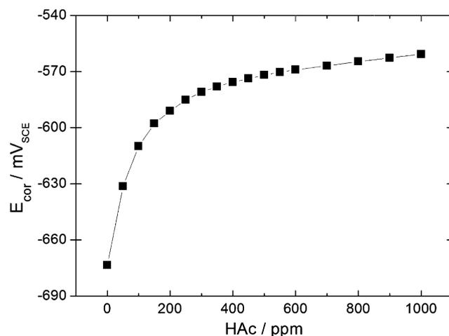
Fig. 2. Corrosion potential of X65 steel in 0.01 M NaCl and 1 bar CO<sub>2</sub> as a function of HAC concentration. In this case,  $E_{\text{corr}} \text{ (mV)} = -740 + 27 \ln([\text{HAC}] + 6)$ . Magnet stirrer rotation  $\omega = 100 \text{ rpm}$ .
