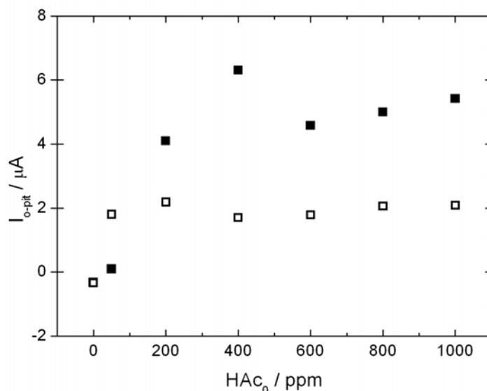
**Figure V.5.** Average values after 12 h of exposure, of the current flowing to a pre-initiated 2 mm depth artificial pit as a function of HAc concentration. 17 mM NaCl and 1 bar CO<sub>2</sub>. (■)  $\omega = 100$  rpm. (□)  $\omega = 200$  rpm.
