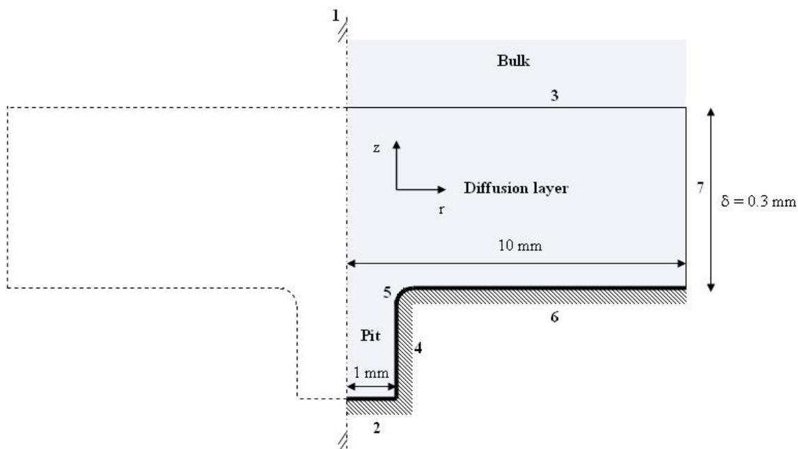
**Figure VI.2.** Dimensional description of the 2D-axisymmetric pit and the corresponding boundary settings. 1- Axial symmetry; 2- Pit bottom:  $i = i_a + i_c$ ; 3-  $C_j = C_j^{eq}$ ; 4- Pit sidewall: Electric insulation; 5- Chamfer: Electric insulation; 6- Outer surface:  $i = i_a + i_c$ ; 7- Electric insulation. The chamfer (boundary 5) was used to smooth the straight corner, thereby simplifying the numerical grid pattern.
