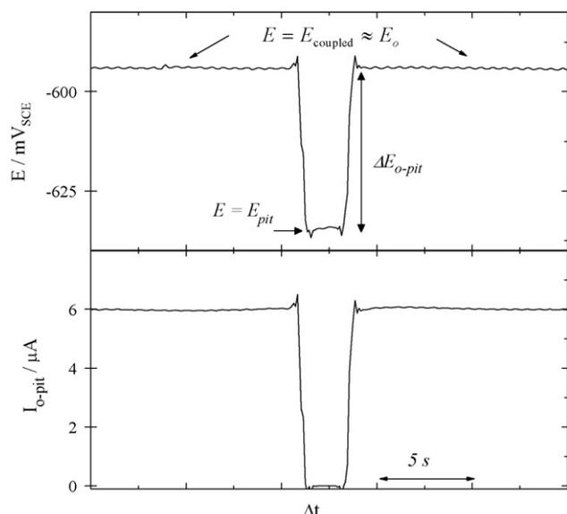
**Fig. 2.** Interrupting the ZRA connection for the determination of the potential difference between the outer large electrode (o) and the inner artificial pit electrode for the case of a 8 mm depth pit after 2 h of immersion in 0.01 M NaCl, 600 ppm HAC and 1 bar CO<sub>2</sub>. Arbitrary time origin.
