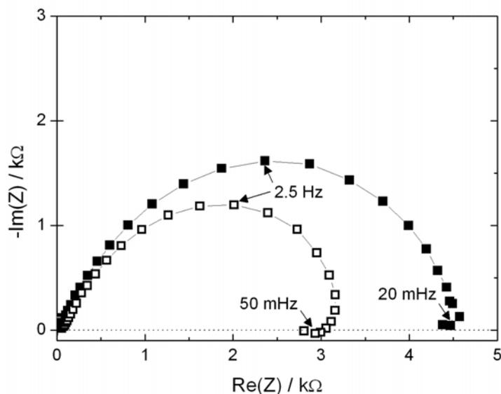
**Figure IV.12.** Nyquist plots obtained for a 2 mm diameter X65 electrode at the corrosion potential in respectively CO<sub>2</sub>-free (■) and 1 bar CO<sub>2</sub>-saturated (□) solutions. 17 mM NaCl, 600 ppm of total HAc, pH 3.5, room temperature.
