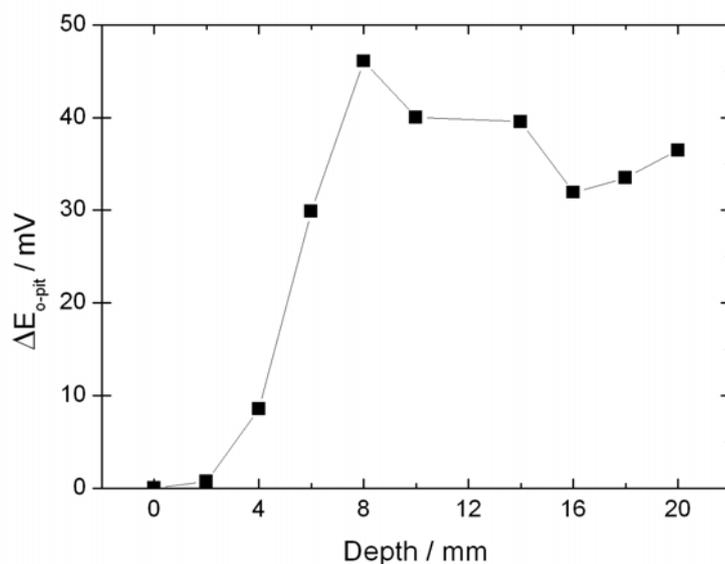
**Figure V.8.** Potential difference between the outer large electrode and the artificial pit electrode as a function of the pit depth in 17 mM NaCl, 600 ppm HAc and 1 bar CO<sub>2</sub>.
