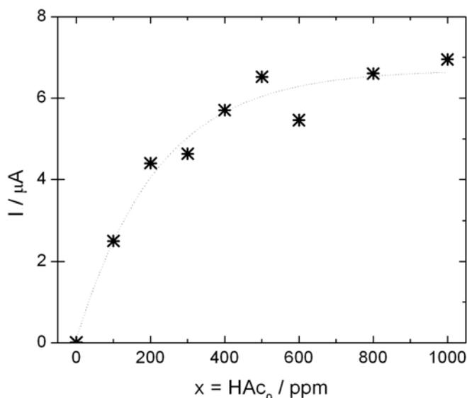
**Figure VI.11.** Current flow between two identical electrodes in a split-cell composed of two identical compartments separated by a high conductivity salt bridge. One of the compartments contained the base  $\text{CO}_2$  saturated (1 bar  $\text{CO}_2$ ) 17 mM NaCl aqueous solution containing  $x$  ppm of HAc. The other compartment was filled with HAc-free solution of 17 mM NaCl saturated with 1 bar  $\text{CO}_2$ .
