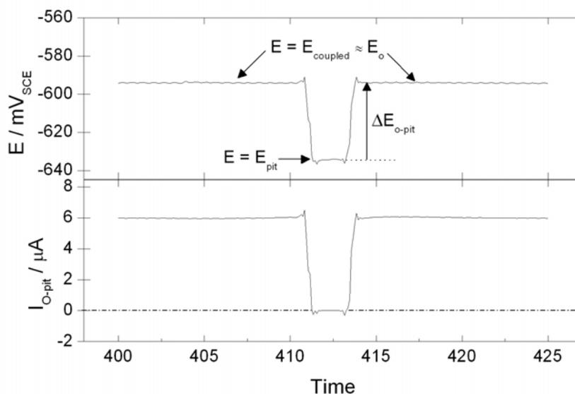
**Figure V.7.** Interrupting the ZRA connection for the determination of the potential difference between the outer large electrode (O) and the inner artificial pit electrode (pit) for the case of a 8 mm depth pit after 2 hours of immersion in 17 mM NaCl, 600 ppm HAc and 1 bar CO<sub>2</sub>. Arbitrary time origin.
