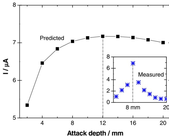
**Fig. 11.** Simulated and measured distributions of the coupling current in the base solution (17 mM NaCl, 600 ppm HAC, 1 bar CO<sub>2</sub>).
