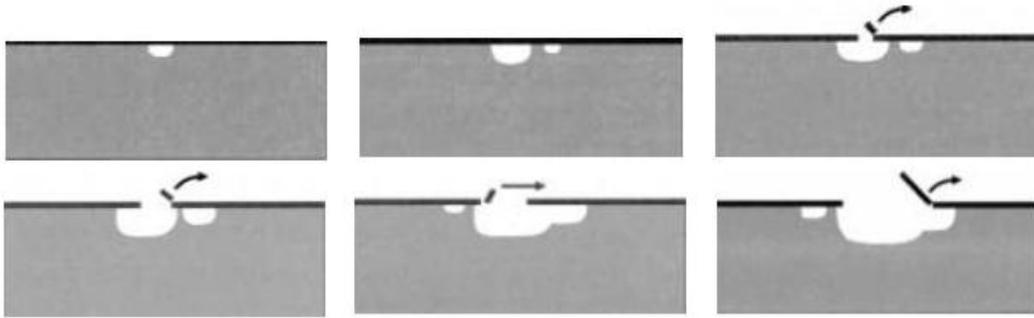
**Figure II.9.** Mechanism for initiation and growth of mesa attacks according to Nyborg [110].
