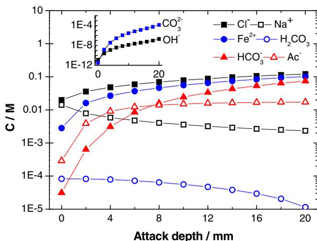
**Fig. 2.** Simulated steady-state composition of the electrolyte along the pit depth in the base solution (17 mM NaCl, 600 ppm HAC, 1 bar  $\text{CO}_2$ ).
