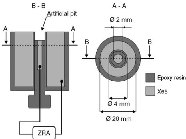
**FIGURE 1.** Schematic illustration of the artificial pit assembly.
