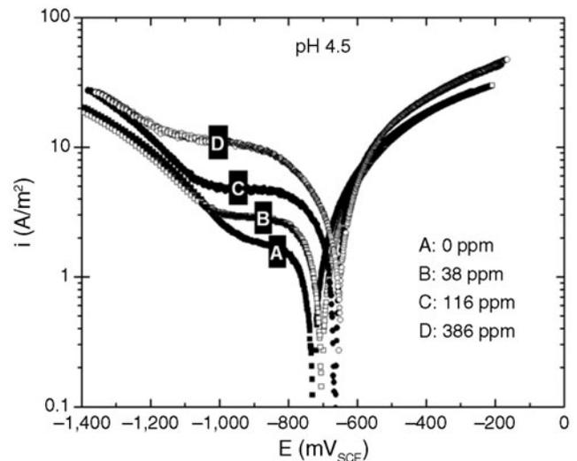
**FIGURE 4.** Polarization curves of X65 steel at different concentrations (A, B, C, D) of free HAC at pH 4.5. 0.1 wt% NaCl, 1 bar CO<sub>2</sub>, room temperature.
