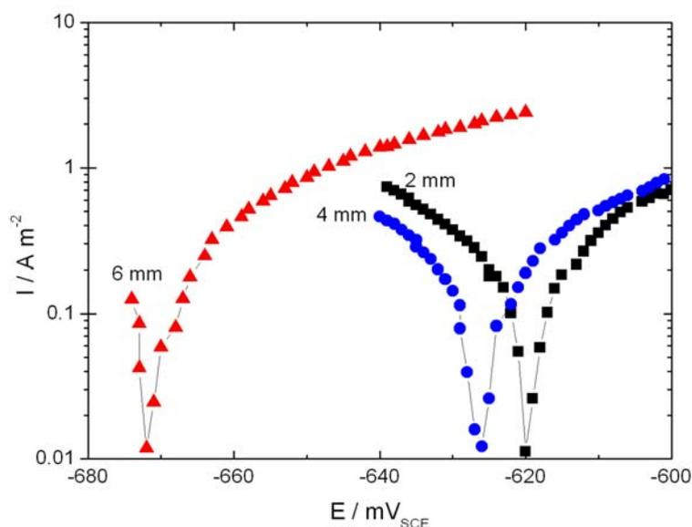
**Figure V.13.** IR-compensated polarization curves of the uncoupled inner electrode of Figure III.5 at different depths in 17 mM NaCl, 600 ppm HAc and 1 bar CO<sub>2</sub>.
