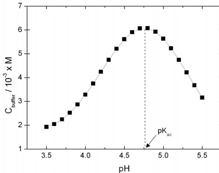
**Figure IV.17.** Variation of the buffer capacity for 600 ppm of total acetic species with pH at room temperature.
