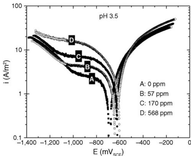
**FIGURE 3.** Polarization curves of X65 steel at different concentrations (A, B, C, D) of free HAC at pH 3.5. 0.1 wt% NaCl, 1 bar CO<sub>2</sub>, room temperature.
