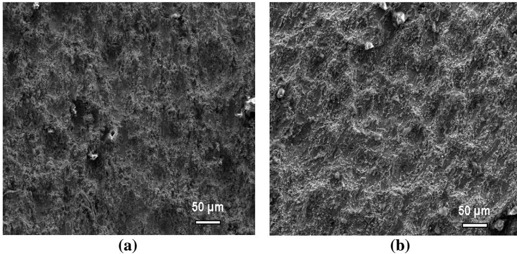
**Figure IV.20.** SEM front view images of sample surfaces after removing the corrosion product layers. 1 bar CO<sub>2</sub>-saturated 17 mM NaCl with 0 ppm (a) and 600 ppm (b) of HAc, initial pH 3.5, room temperature. Magnification = 100X.
