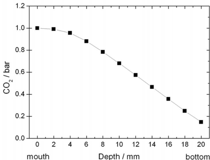
**Figure VI.5.** Simulated steady-state profile of CO<sub>2</sub> concentration, reported as equilibrium partial pressure.
