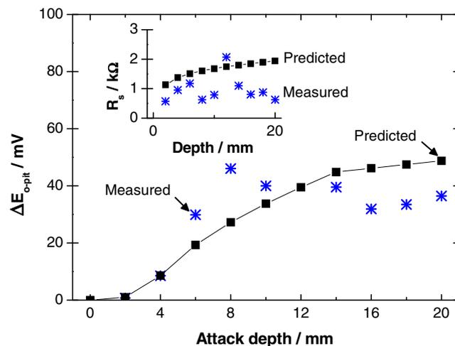
**Fig. 10.** Simulated and measured IR-uncompensated distributions of the potential difference between the outer large surface and the pit bottom in the base solution (17 mM NaCl, 600 ppm HAC, 1 bar CO<sub>2</sub>). Also shown in the inset is a comparison between simulated and measured values of the ohmic resistance of the narrow electrolyte path inside the pit.
