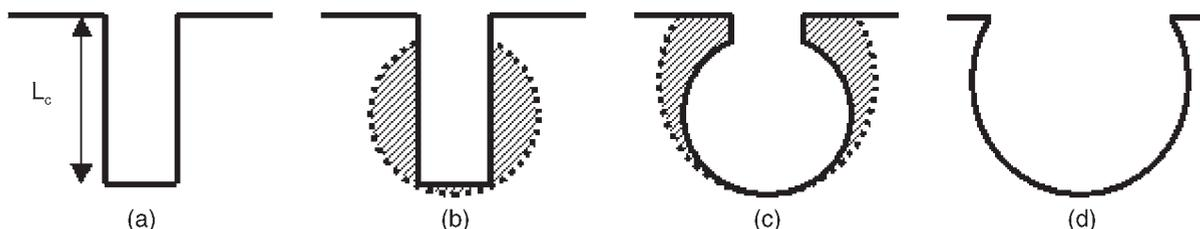
**FIGURE 14.** Descriptive scenario for propagation and stabilization of localized attacks. (a) The attack stops propagating downward when reaching the critical depth  $L_c$ . (b) The attack undergoes a lateral growth. (c) The attack propagates upward. (d) The attack is stabilized.
