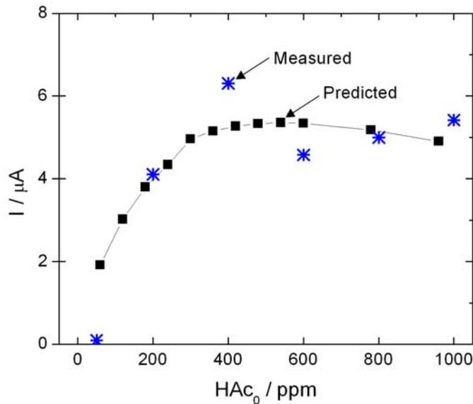
**Figure VI.14.** Simulated and measured coupling currents vs. the initial concentration of HAc for a pit of 2 mm diameter and 2 mm depth in 17 mM NaCl and 1 bar CO<sub>2</sub>.
