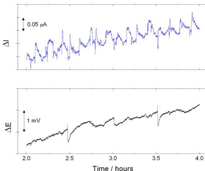
**Figure V.1.** Time records of current and potential for a freely corroding X65 electrode in 17 mM NaCl solution saturated with 1 bar CO<sub>2</sub> at pH 3.5 and room temperature.
