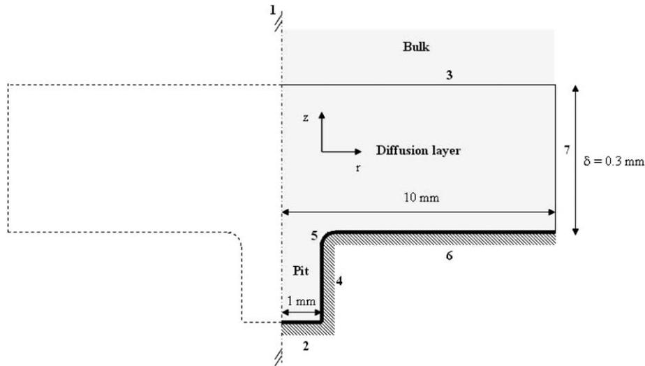
**Fig. 1.** Dimensional description of the 2D-axisymmetric pit and the corresponding boundary settings. 1- Axial symmetry; 2- Pit bottom:  $i = i_a + i_c$ ; 3-  $C_j = C_j^0$ ; 4- Pit sidewall: Electric insulation; 5- Chamfer: Electric insulation; 6- Outer surface:  $i = i_a + i_c$ ; 7- Electric insulation. The chamfer (boundary 5) was used to smooth the straight corner, thereby simplifying the numerical grid pattern.
