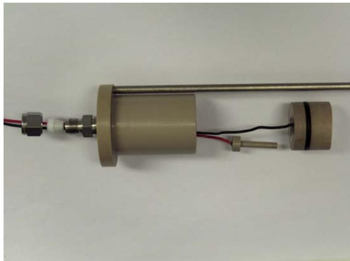
*Figure III.A1b. Detailed side view of the artificial pit device.*
