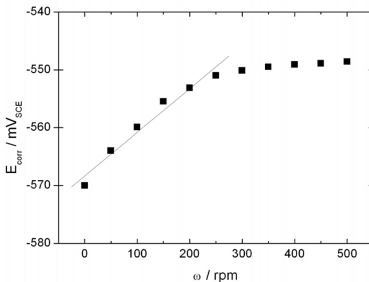
**Figure IV.15.** Corrosion potential of X65 pipeline steel at various rotation rates of the magnet stirrer in 1 bar CO<sub>2</sub>-saturated 17 mM NaCl solution containing 600 ppm of total HAc. pH 3.5, room temperature. rpm = rotation per minute.
