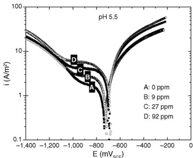
**FIGURE 5.** Polarization curves of X65 steel at different concentrations (A, B, C, D) of free HAc at pH 5.5. 0.1 wt% NaCl, 1 bar CO<sub>2</sub>, room temperature.
