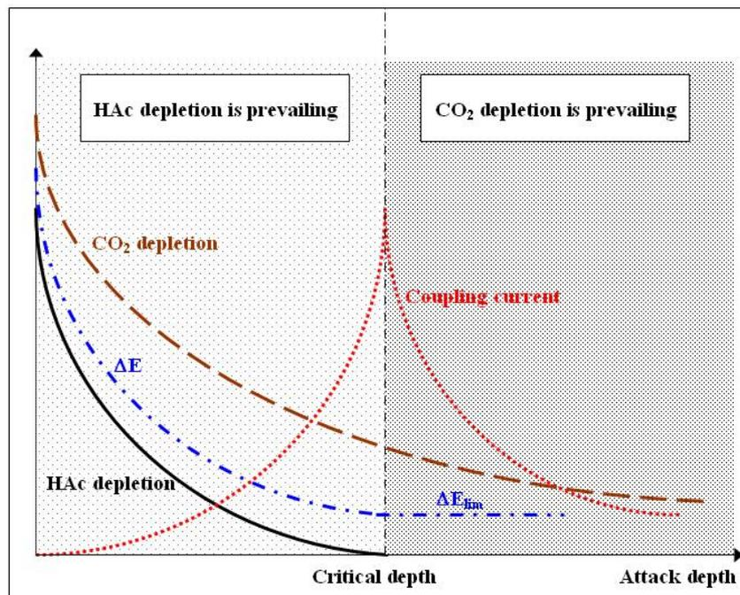
**Figure VII.1.** Schematic illustration for the mechanisms of growth and stifling of localized corrosion attacks according to the counteracting depletions of HAc and  $\text{CO}_2$ .  $\Delta E$  = potential difference.
