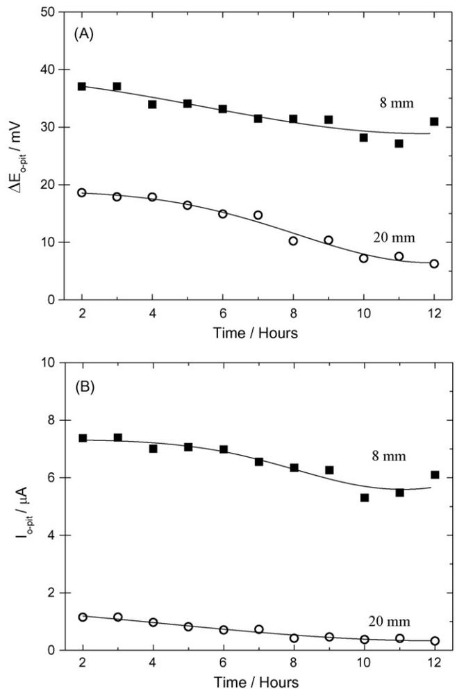
**Fig. 6.** Typical time evolution of the potential difference (A) and the coupling current flow (B) between the outer large electrode and the artificial pit electrode for 8 mm and 20 mm depths in 0.01 M NaCl, 600 ppm HAC and 1 bar  $\text{CO}_2$ .
