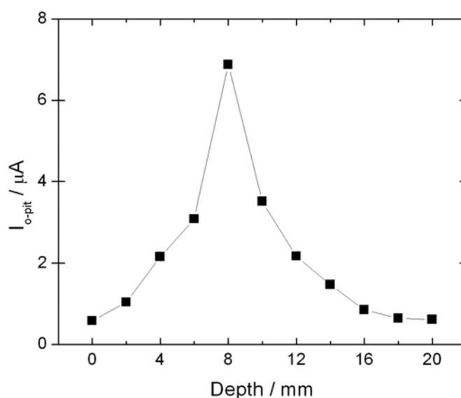
**Figure V.6.** Average coupling current vs. pit depth in 17 mM NaCl, 600 ppm HAc and 1 bar CO<sub>2</sub>.
