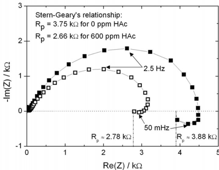
**Figure IV.11.** Nyquist plots obtained for a 2 mm diameter X65 electrode at the corrosion potential in 1 bar CO<sub>2</sub>-saturated 17 mM NaCl solution for 0 ppm (■) and 600 ppm (□) of total HAc. pH 3.5, room temperature.
