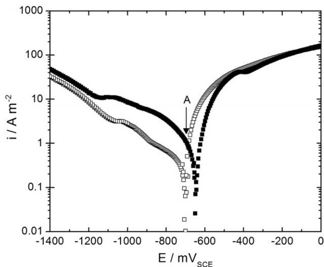
Fig. 1. Polarization curves of X65 steel in 0.01 M NaCl and 1 bar CO<sub>2</sub> at 0 (□) and 600 ppm of HAC. Natural convection.
