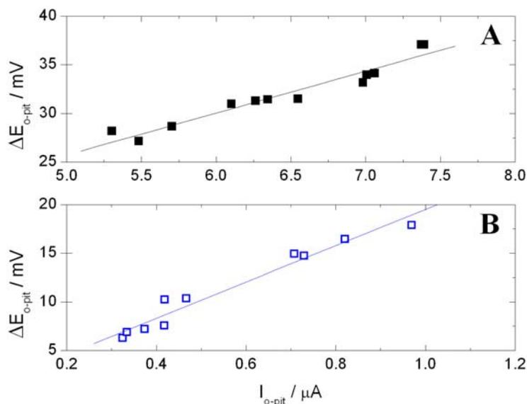
**Figure V.11.** Potential-current relationship for 8 mm (A) and 20 mm (B) pit depth during the time evolution of the potential difference and the coupling current between the outer large surface and the artificial pit as depicted in Figure V.10. 17 mM NaCl, 600 ppm HAc and 1 bar CO<sub>2</sub>.
