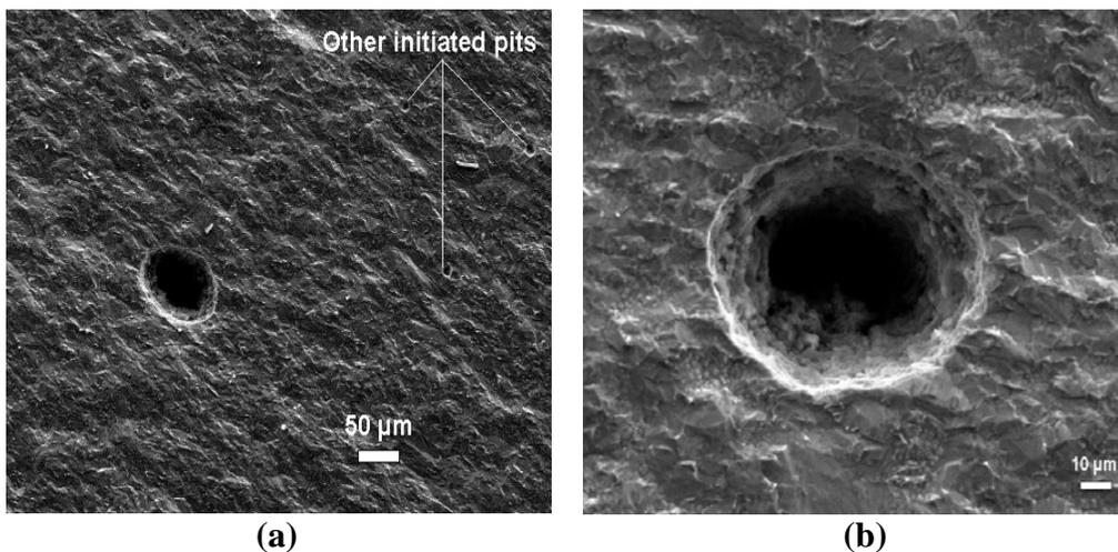
**Figure IV.23.** Pitting morphologies on X65 sample immersed during 30 days in 600 ppm HAC-containing solution. 1 bar CO<sub>2</sub>-saturated 17 mM NaCl, initial pH 5.5, room temperature. Magnification = 100X (a), 500X (b).
