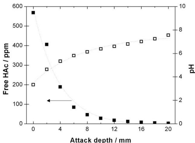
**Fig. 6.** Simulated steady-state profiles of HAC concentration and pH in the base solution (17 mM NaCl, 600 ppm HAC, 1 bar CO<sub>2</sub>).
