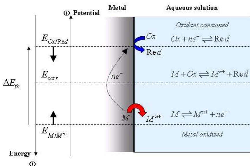
**Figure I.4.** Thermodynamic driving force of aqueous metallic corrosion in the presence of a soluble oxidant. The coupling between the two half-reactions occurs at the corrosion potential,  $E_{corr}$ . The latter depends on the relative rates of the anodic and cathodic reactions.
