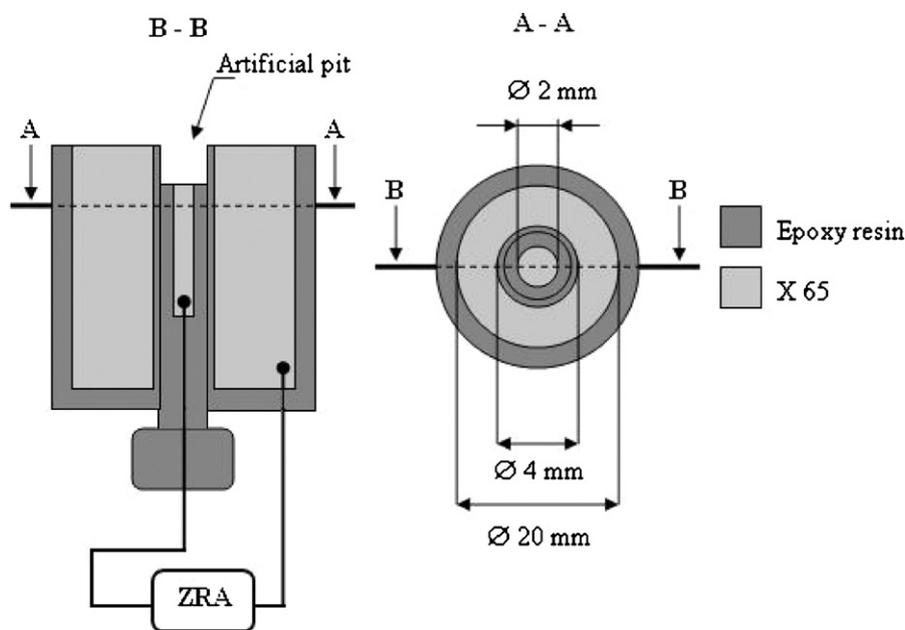
Fig. 1. Artificial pit assembly and ZRA connection.
