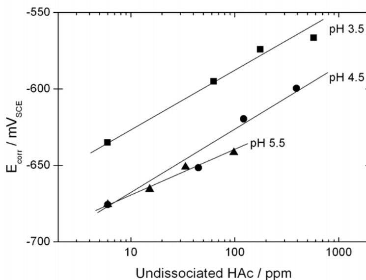
**Figure IV.14.** Linear dependence of the corrosion potential on the concentration of undissociated HAc at constant pH in 1 bar CO<sub>2</sub>-saturated 17 mM NaCl solutions. Room temperature.
