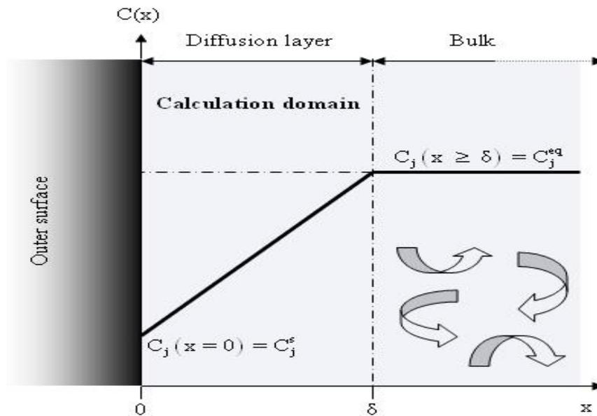
**Figure VI.1.** Concentration profile for a species  $j$  as a function of the distance from the outer surface in steady-state diffusion - convection regime. The terms  $C_j^{eq}$  and  $C_j^s$  stand for the equilibrium and surface concentrations, respectively.
