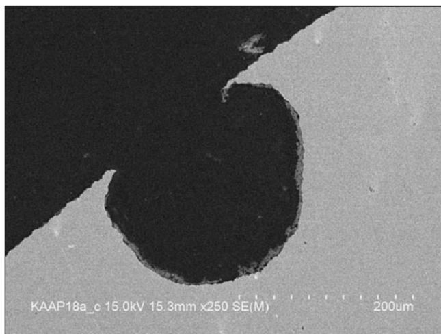
**FIGURE 15.** SEM image of a typical hemispherical morphology of localized corrosion attacks observed for carbon steel exposed to  $\text{CO}_2/\text{HAc}$  environment. 0.3 wt% NaCl, 1 bar  $\text{CO}_2$ , 600 ppm of total acetic species, room temperature.
