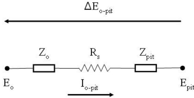
**Figure V.14.** Equivalent circuit for the asymmetric artificial pit electrode assembly of Figure III.5.
