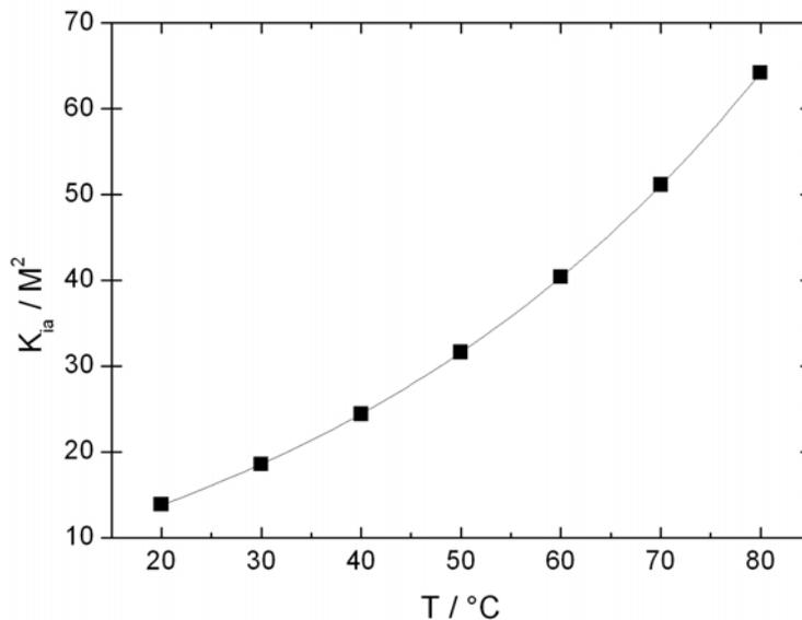
**Figure II.11.** Variation of ferrous acetate's solubility with temperature in 0.3% NaCl. Data were obtained by polynomial fitting of those reported by Palmer and used later by Gulbrandsen and Bilkova [3, 10].
