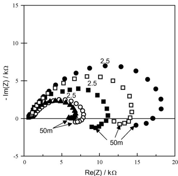
**Fig. 10.** Nyquist plots of the electrochemical impedance of artificial pits of different depths in 0.01 M NaCl, 600 ppm HAC and 1 bar CO<sub>2</sub>: (■) 2 mm; (○) 6 mm; (▲) 10 mm; (□) 16 mm; (◆) 18 mm. Frequency values in Hz.
