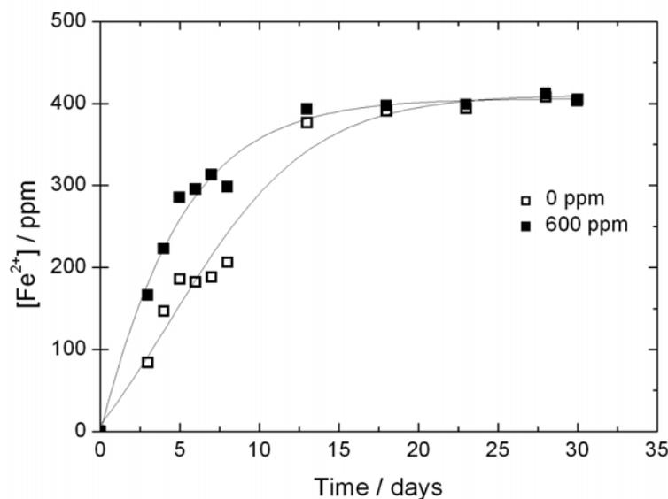
**Figure IV.18.** Experimental iron (II) content-time curves in respectively HAc-free and 600 ppm HAc-containing solutions saturated with 1 bar CO<sub>2</sub>. 17 mM NaCl, initial pH 3.5, room temperature. No HAc replenishment was made thereafter.
