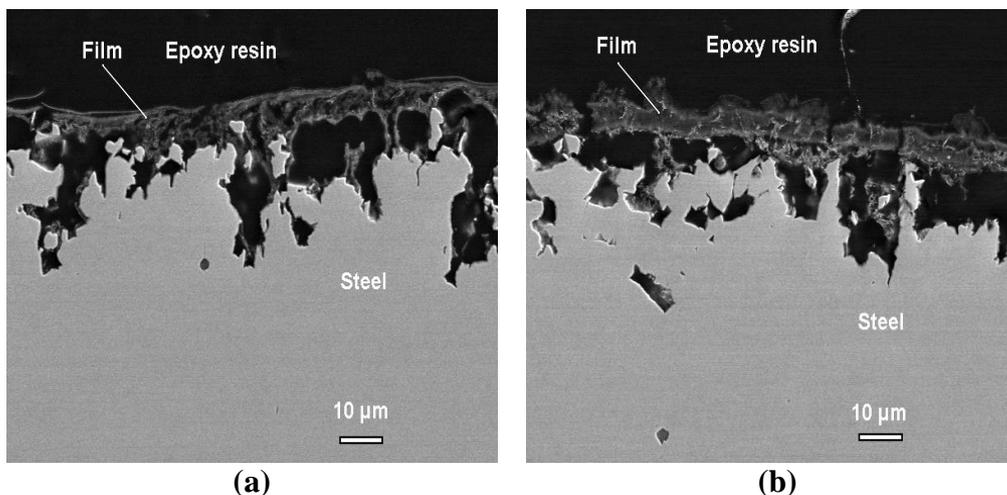
**Figure IV.21.** SEM images of sample cross-sections. 1 bar CO<sub>2</sub>-saturated 17 mM NaCl with 0 ppm (a) and 600 ppm (b) of HAc, initial pH 3.5, room temperature. Magnification = 500X.
