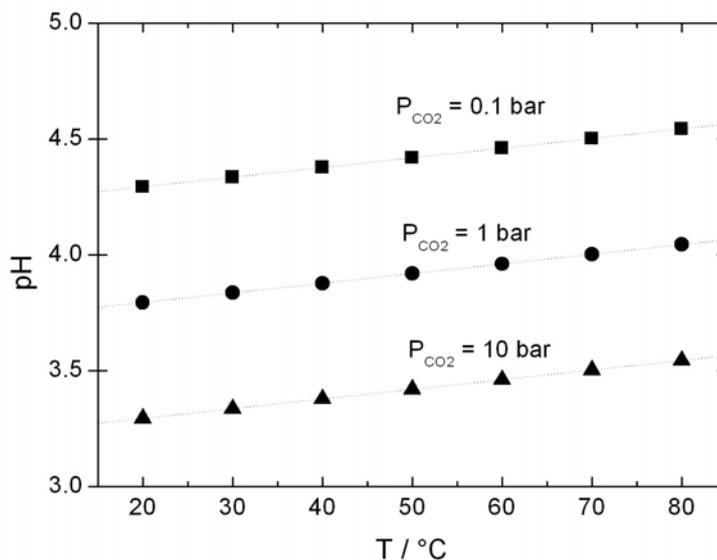
**Figure II.6.** Graphical illustration of a pH-T- $P_{CO_2}$  diagram in pure CO<sub>2</sub>-water systems according to equation (II.23).
