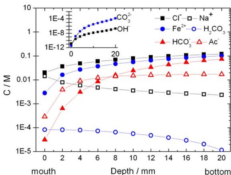
**Figure VI.4.** Simulated steady-state composition of the electrolyte along the pit depth.
