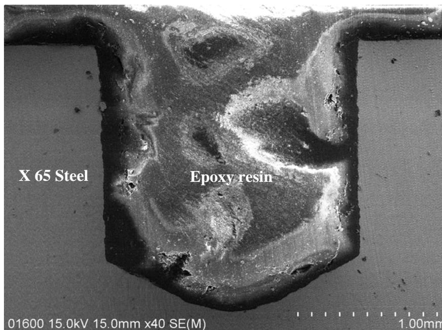
**Figure VI.7.** SEM cross-section of 2 mm-depth attack on X65 sample after immersion during 3 months in 17 mM NaCl and 600 ppm HAc (0 bar CO<sub>2</sub>). The solution was continuously purged with nitrogen to prevent oxygen ingress.
