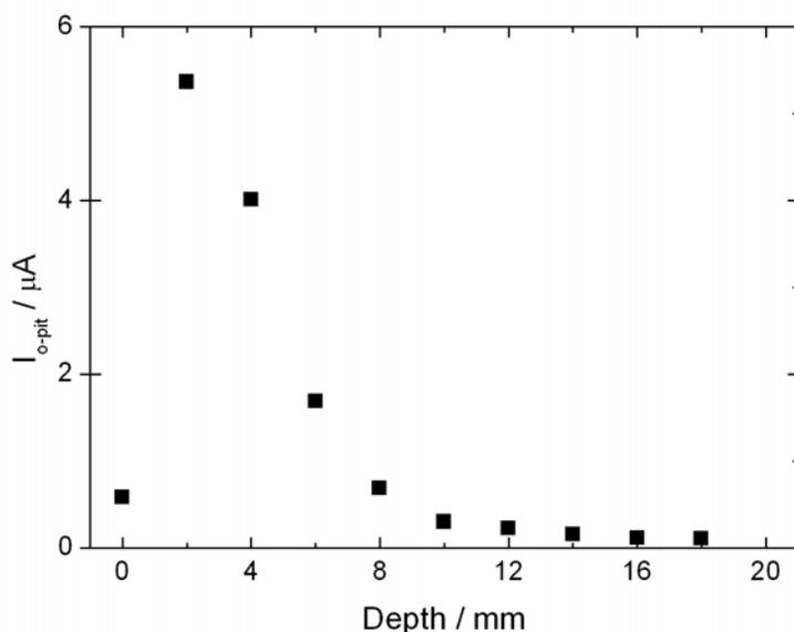
**Figure V.16.** Average coupling current versus pit depth with corroding steel sidewalls in 17 mM NaCl, 600 ppm HAc and 1 bar CO<sub>2</sub>.
