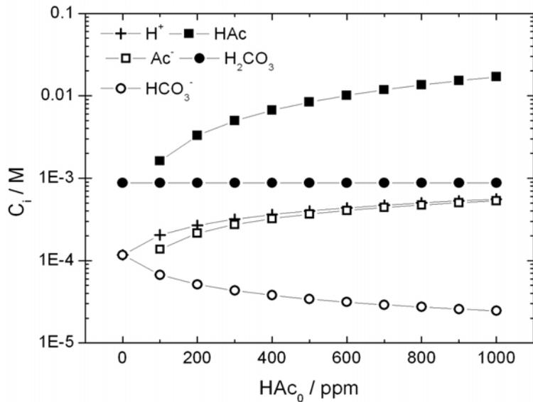
**Figure IV.2.** System speciation at 25 °C as a function of the initial concentration of acetic acid. 17 mM NaCl, 1 bar CO<sub>2</sub> (open system).
