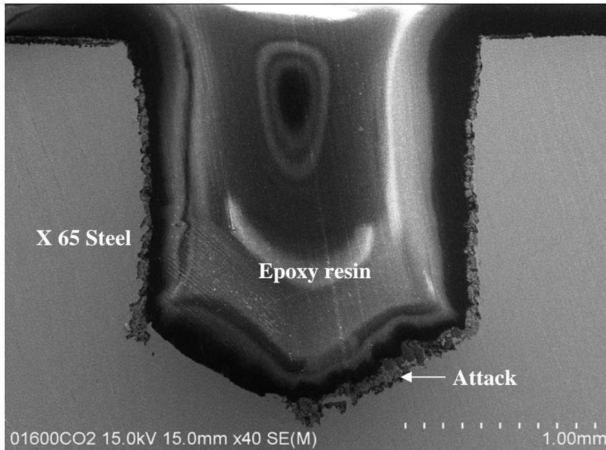
**Figure VI.10.** SEM cross-section of 2 mm-depth attack on X65 sample after immersion during 3 months in 17 mM NaCl and 600 ppm HAc saturated with 1 bar CO<sub>2</sub>.
