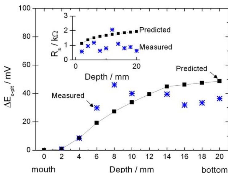
**Figure VI.12.** Simulated and measured IR-uncompensated distributions of the potential difference between the outer large surface and the pit base. Also shown in the inset is a comparison between predicted and measured values of the ohmic resistance of the narrow electrolyte path inside the pit.
