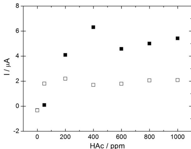
Fig. 3. Average values after 12 h of exposure, of the current  $I$  flowing to a pre-initiated 2-mm depth artificial pit as a function of HAc concentration. 0.01 M NaCl and 1 bar  $\text{CO}_2$ . (■)  $\omega = 100$  rpm. (□)  $\omega = 200$  rpm.
