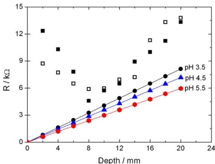
**Figure V.12.** Experimental values of the slope  $R$  of the potential-current linear relationship as shown in Figure V.11 as a function of the pit depth (■); theoretical electrolyte resistance  $R_s$  at different pH values for a perfect cylindrical geometry (solid lines) and  $R$  values computed from equation (V.13) with  $R_s$  and  $R_{p, pit}$  obtained from electrochemical impedance measurements (□), see Figure V.14 below.
