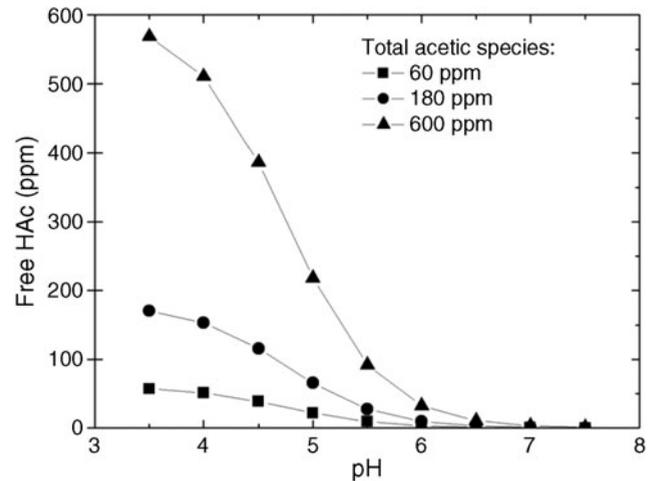
**FIGURE 2.** Variation of the free HAC concentration with pH at different amounts of total acetic species. 0.1 wt% NaCl, 1 bar CO<sub>2</sub>, room temperature.
