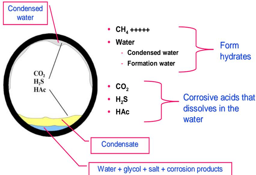
**Figure I.3.** Key factors involved in TLC phenomenon. Any injected corrosion inhibitor remains at the bottom of the line, and is not able to protect the top of the line.
