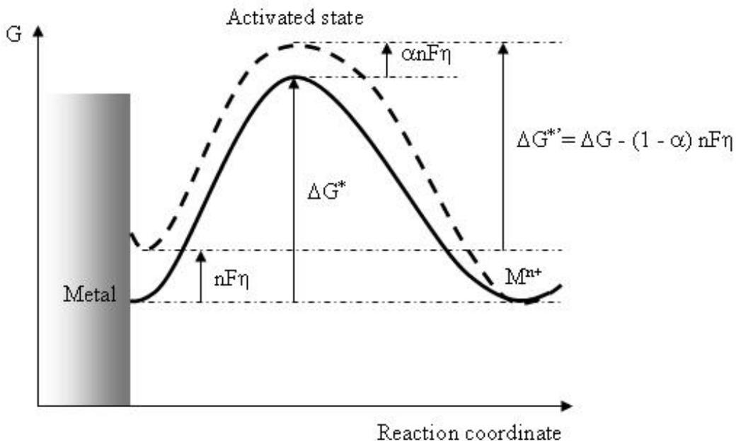
**Figure I.6.** Schematic distribution of free energies for an anodically polarized electrode under activation control (overpotential  $\eta_A > 0$ ). The parameter  $\alpha \in [0; 1]$  denotes the symmetry factor that defines the position of the activated state in respect with the two minima.
