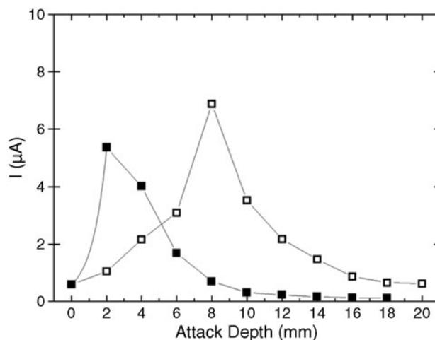
**FIGURE 13.** Average coupling current for artificial pits with (□) reactive and (■) inert insulating sidewalls in 0.1% NaCl, 600 ppm of total acetic species, 1 bar  $CO_2$ , room temperature.
