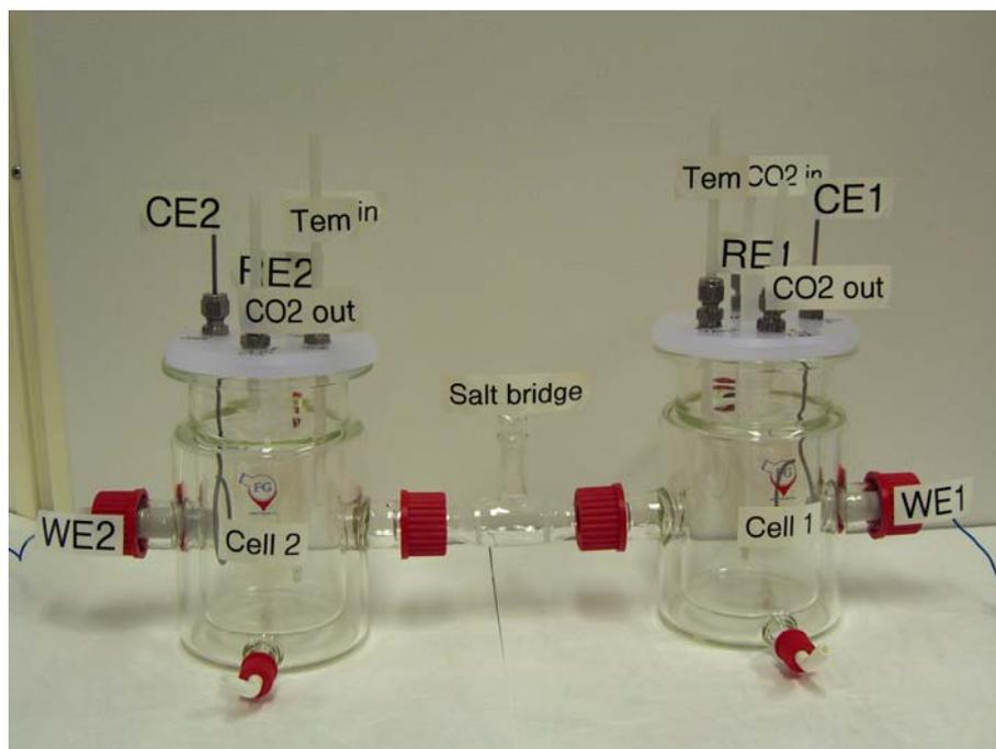
**Figure III.6.** View of the split cell assembly.
