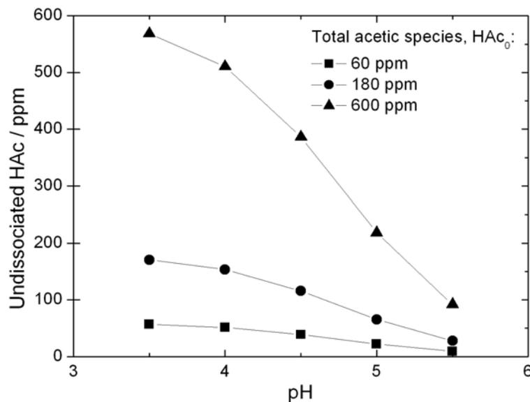
**Figure IV.3.** Calculated concentrations of undissociated HAc as a function of pH at room temperature for various total amounts of acetic species initially added to the test solution.
