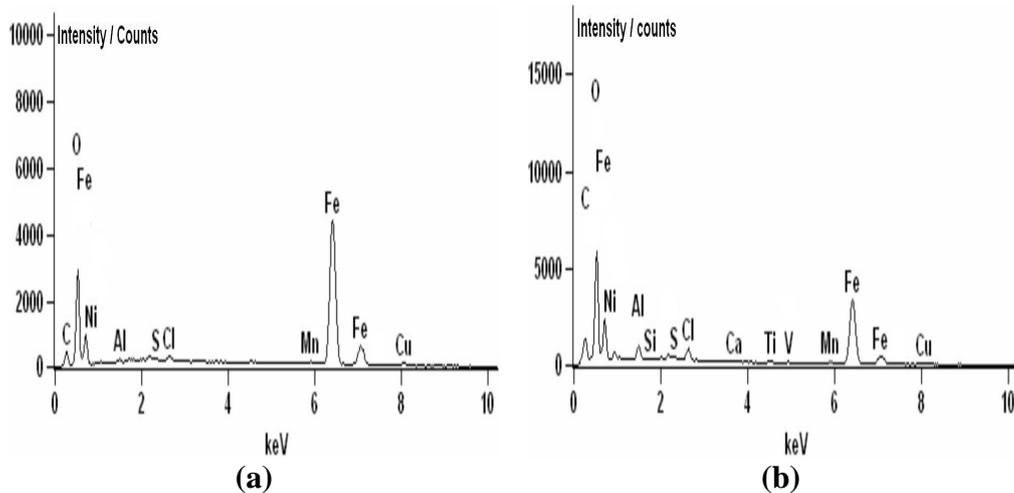
**Figure IV.22.** EDS patterns of the two corrosion films. 1 bar CO<sub>2</sub>-saturated 17 mM NaCl with 0 ppm (a) and 600 ppm (b) of HAC, initial pH 3.5, room temperature.
