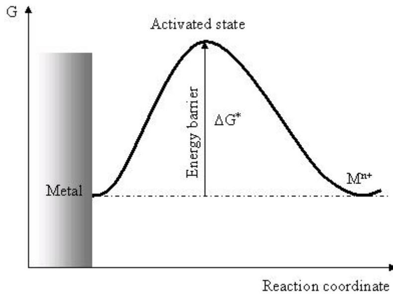
**Figure I.5.** Schematic distribution of the free energy. The activation Gibbs free energy  $\Delta G^*$  is the excess of energy that must be acquired by the metallic element to transform into a soluble metallic ion  $M^{n+}$ .
