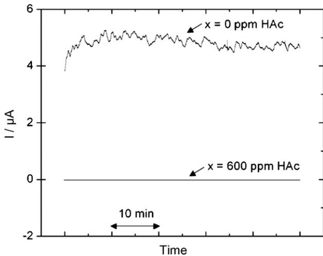
**Fig. 4.** Current flow between two identical electrodes in a split-cell composed of two identical compartments separated by a high conductivity salt bridge. One of the compartments contained the base  $\text{CO}_2$  saturated (1 bar  $\text{CO}_2$ ) 0.01 M NaCl aqueous solution containing 600 ppm. The other compartment simulated distinct conditions of no depletion ( $x = 600$  ppm) and total depletion ( $x = 0$  ppm) of HAC.
