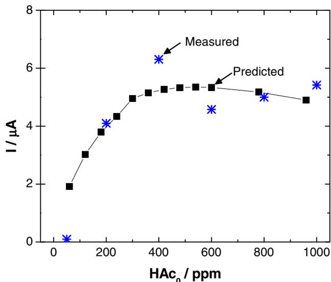
Fig. 12. Simulated and measured coupling currents versus the initial concentration of HAC for a pit of 2 mm diameter and 2 mm depth in 17 mM NaCl solution saturated with 1 bar CO<sub>2</sub>.
