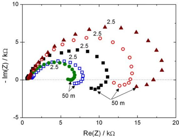
**Figure V.15.** Nyquist plots of the electrochemical impedance of artificial pits at different depths in 17 mM NaCl, 600 ppm HAc and 1 bar CO<sub>2</sub>. (■) 2 mm; (□) 6 mm; (●) 10 mm; (○) 16 mm; (▲) 18 mm. Frequency values in Hz.
