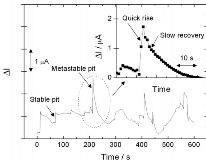
**Figure V.3.** Typical current transients generated on freely corroding X65 electrode in CO<sub>2</sub>/HAc brine at room temperature. Also shown is an expanded time scale featuring an individual metastable pit current spike.
