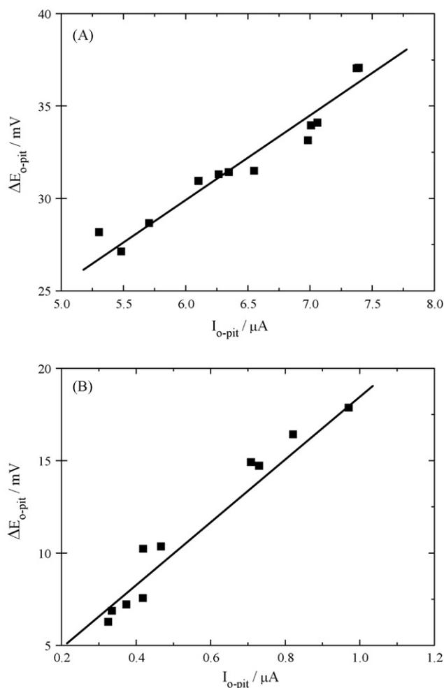
**Fig. 7.** Potential–current relationship for 8 mm (A) and 20 mm (B) pit depth during the time evolution of the potential difference and the coupling current between the outer large surface and the artificial pit as depicted in Fig. 5. 0.01 M NaCl, 600 ppm HAc and 1 bar CO<sub>2</sub>.
