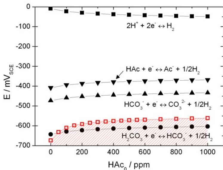
**Figure IV.10.** Comparison between the measured corrosion potentials of X65 pipeline steel (red unfilled-square symbols) and the calculated equilibrium potentials of cathodic reactions (see Tables IV.2 and IV.4) for various concentrations of total HAc at free pH. 1 bar CO<sub>2</sub>, 17 mM NaCl, room temperature.
