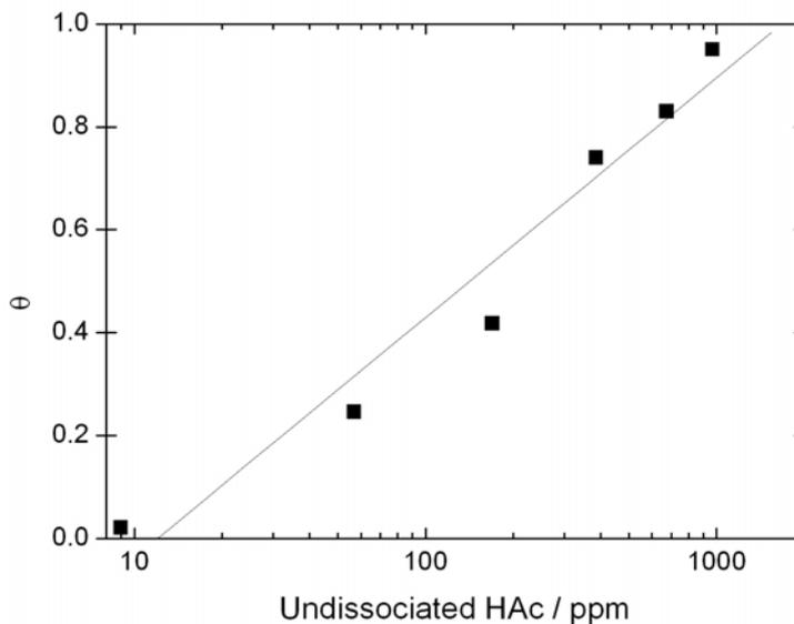
**Figure IV.13.** Adsorption isotherm of undissociated HAc molecules on X65 carbon steel electrodes in 1 bar CO<sub>2</sub>-saturated 17 mM NaCl solutions at  $E = -600 \text{ mV}_{\text{SCE}}$ , pH 3.5, room temperature.
