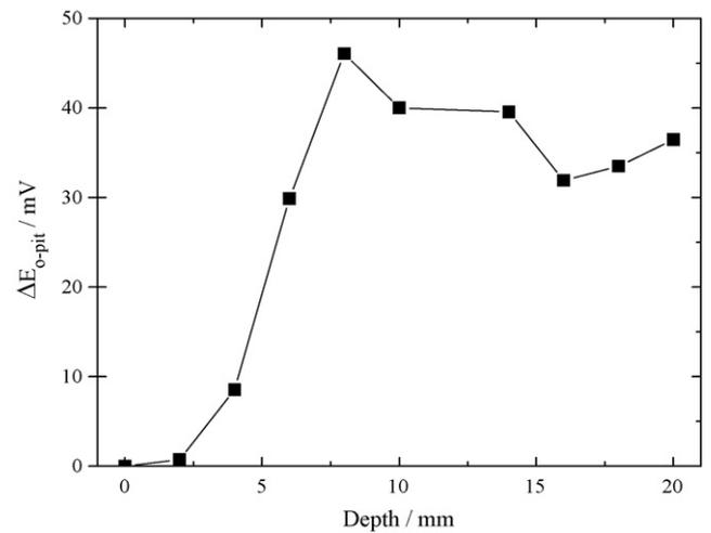
**Fig. 5.** Potential difference between the outer large electrode and the artificial pit electrode as a function of the pit depth in 0.01 M NaCl, 600 ppm HAC and 1 bar  $\text{CO}_2$ .
