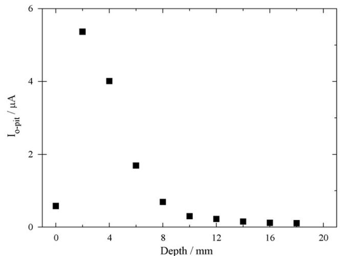
**Fig. 11.** Average coupling current versus pit depth with corroding steel sidewalls in 0.01 M NaCl, 600 ppm HAC and 1 bar CO<sub>2</sub>.
