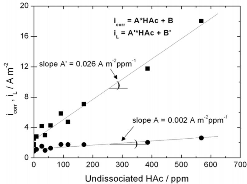
**Figure IV.7.** Respective variations of the cathodic limiting current density (■) and the corrosion current density (●) with the concentration of undissociated HAc for a pH within the range 3.5 – 5.5. Data were obtained for X65 pipeline steel corroding in 1 bar CO<sub>2</sub>-saturated 17 mM NaCl solutions at room temperature.
