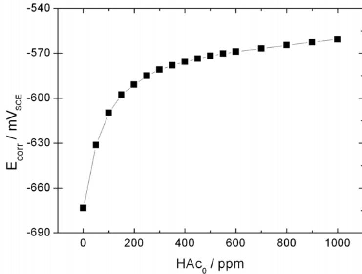
**Figure IV.8.** Corrosion potential of X65 pipeline steel in 1 bar CO<sub>2</sub>-saturated 17 mM NaCl as a function of total HAc concentration at free pH. Room temperature.
