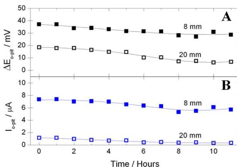
**Figure V.10.** Typical time evolution of the potential difference (A) and the coupling current flow (B) between the outer large electrode and the artificial pit electrode for 8 mm and 20 mm depths in 17 mM NaCl, 600 ppm HAc and 1 bar CO<sub>2</sub>.
