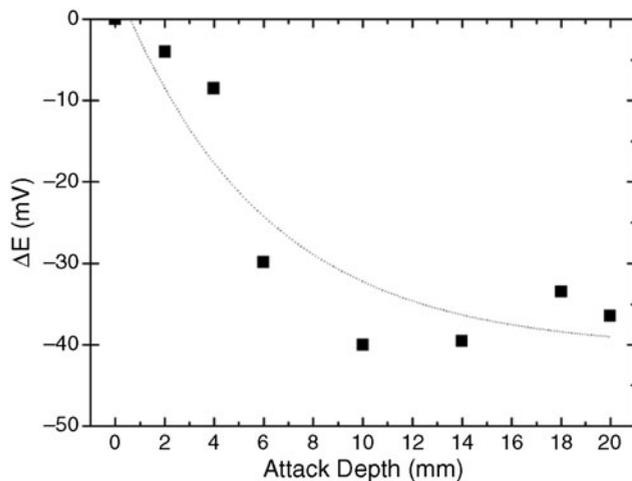
**FIGURE 10.** Variation of the potential difference  $\Delta E$  with attack depth with insulating sidewalls in the base solution at room temperature. At a given depth,  $\Delta E$  is reported as the average of many interrupt measurements during 2 h of exposure time.
