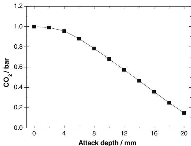
**Fig. 3.** Simulated steady-state profile of  $\text{CO}_2$  concentration, reported as equilibrium partial pressure, along the pit depth in the base solution (17 mM NaCl, 600 ppm HAC, 1 bar  $\text{CO}_2$ ).
