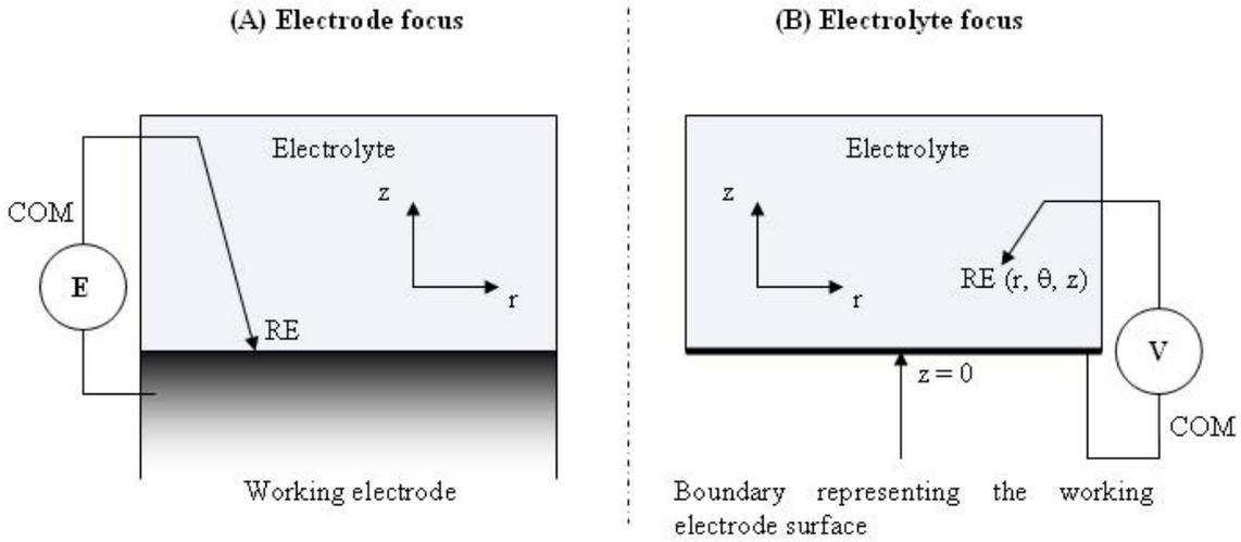
**Figure VI.3.** Determination of the electrode potential according to the experimental approach (A) and the modelling approach (B). RE = reference electrode.
