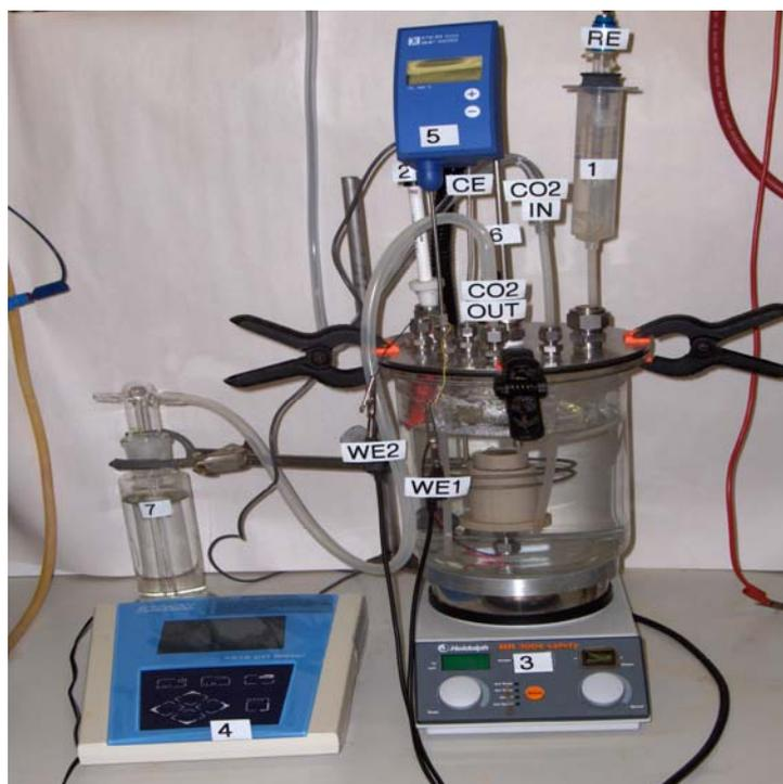
**Figure III.3.** Experimental setup. 1 (RE): reference electrode; 2: pH probe; 3: thermostatically controlled heating plate; 4: pH-meter; 5: temperature probe; 6: specimen holder; 7: bubble flask; CO<sub>2</sub> IN: CO<sub>2</sub> gas inlet; CO<sub>2</sub> OUT: CO<sub>2</sub> gas outlet.
