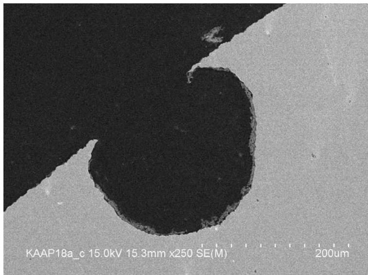
**Figure V.18.** SEM image of a pit cross-section showing a hemispherical morphology typically observed for attacks on carbon steel in CO<sub>2</sub>/HAc brine at room temperature. 0.051 M NaCl, 1 bar CO<sub>2</sub>, 600 ppm HAc. Magnification = 250X.
