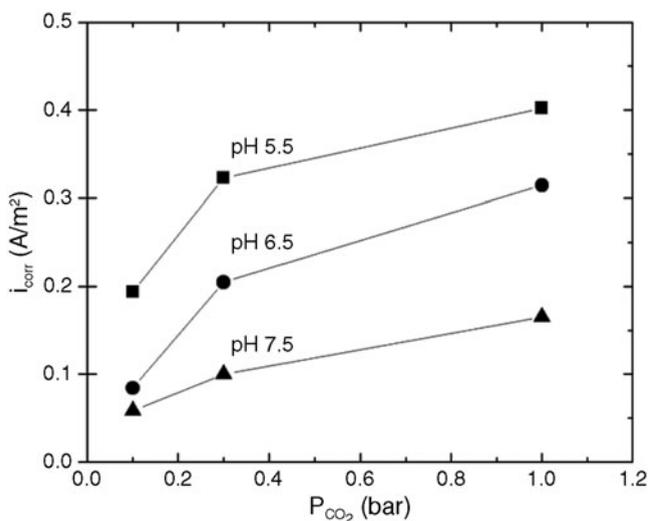
**FIGURE 12.** The effect of  $CO_2$  partial pressure on the corrosion current density at different pH values. Data were estimated from polarization curves measured on X65 steel under different  $CO_2$  partial pressures and pH. 0.1 wt% NaCl, 600 ppm of total acetic species, room temperature.
