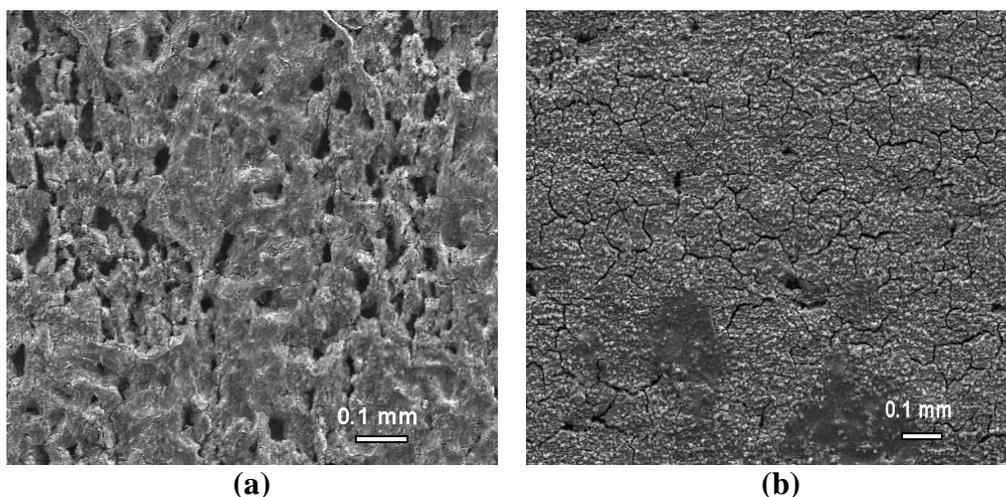
**Figure IV.19.** SEM front view images of X65 samples after 30 days immersion in HAc-free (a) and 600 ppm HAc-containing (b) solutions saturated with 1 bar CO<sub>2</sub>. 17 mM NaCl, initial pH 3.5, room temperature. Magnification = 50X.
