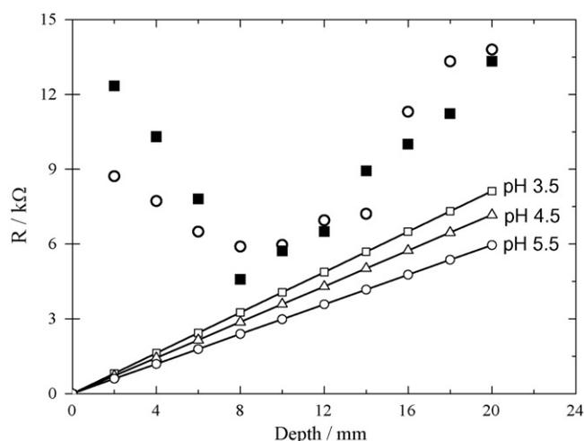
**Fig. 8.** Experimental values of the slope  $R$  of the potential–current linear relationship as shown in Fig. 6 as a function of the pit depth (■); theoretical electrolyte resistance  $R_e$  at different pH values for a perfect cylindrical geometry (solid lines) and  $R$  values computed from Eq. (3) with  $R_s$  and  $R_{p,pit}$  obtained from electrochemical impedance measurements (○), see Fig. 9.
