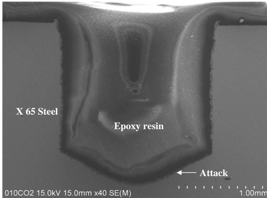
**Figure VI.9.** SEM cross-section of 2 mm-depth attack on X65 sample after immersion during 3 months in 17 mM NaCl and 0 ppm HAc saturated with 1 bar CO<sub>2</sub>.
