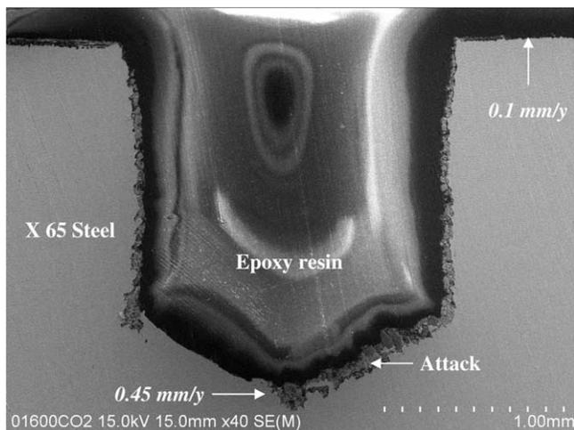
**Fig. 8.** SEM cross-section of 2 mm-depth attack on API 5L X65 sample after immersion during 3 months in 17 mM NaCl and 600 ppm HAC saturated with 1 bar CO<sub>2</sub>.
