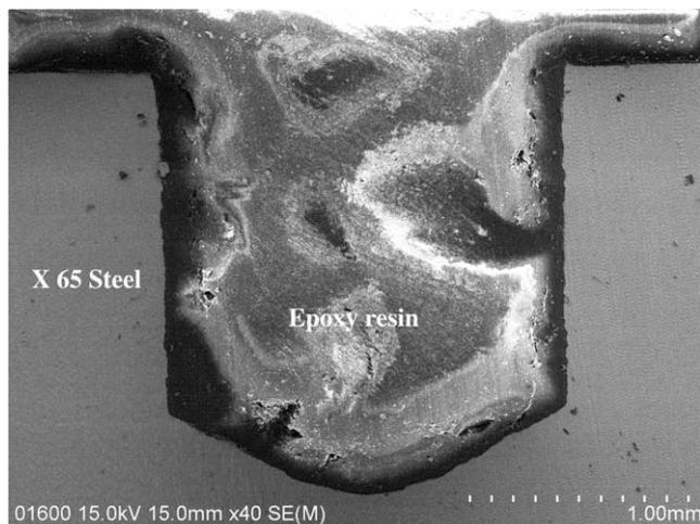
**Fig. 5.** SEM cross-section of 2 mm-depth attack on API 5L X65 sample after immersion during 3 months in 17 mM NaCl and 600 ppm HAC (0 bar CO<sub>2</sub>). The solution was continuously purged with nitrogen to prevent oxygen ingress.
