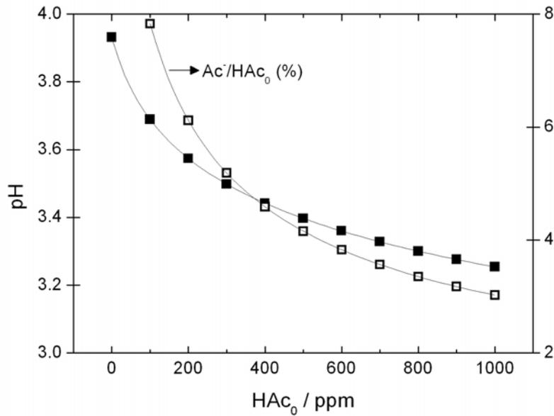
**Figure IV.1.** Simulated variation of pH with initial HAc concentration in simulated 17 mM aqueous NaCl solution saturated with 1 bar CO<sub>2</sub> at 25 °C (open system). In such a range of pH, acetic acid is clearly shown to be present mainly in its undissociated form (free HAc).
