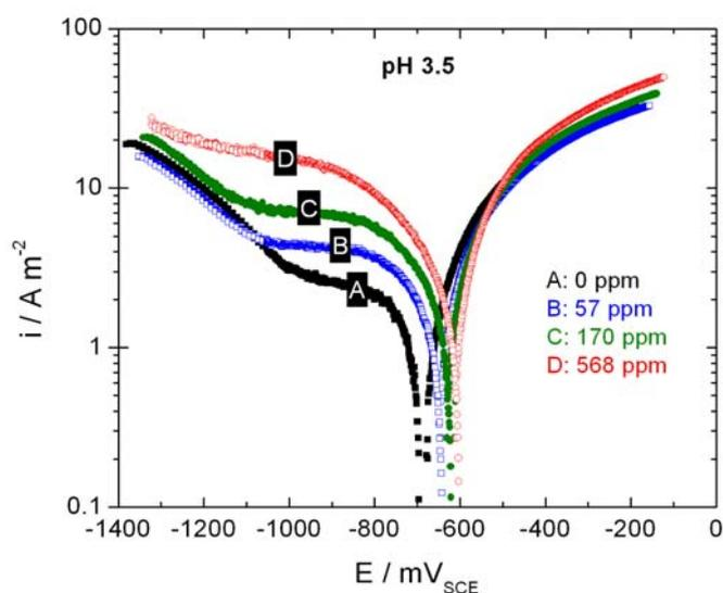
**Figure IV.4.** Polarization curves of X65 pipeline steel at room temperature in 1 bar CO<sub>2</sub>-saturated 17 mM NaCl solutions containing various amounts of free HAc (A-D) at pH 3.5.
