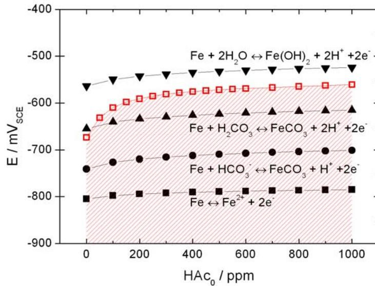
**Figure IV.9.** Comparison between the measured corrosion potentials of X65 pipeline steel (red unfilled-square symbols) and the calculated equilibrium potentials of anodic reactions (see Tables IV.2 and IV.4) for various concentrations of total HAC at free pH. 1 bar CO<sub>2</sub>, 17 mM NaCl, room temperature.
