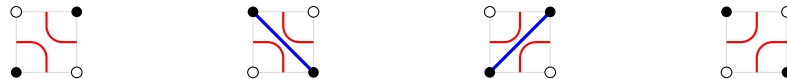
Figure 1.3: A map between the CPL and bond percolation in the odd sub lattice is given by the correspondence above. Here the odd sub lattice is represented by the filled circles.
