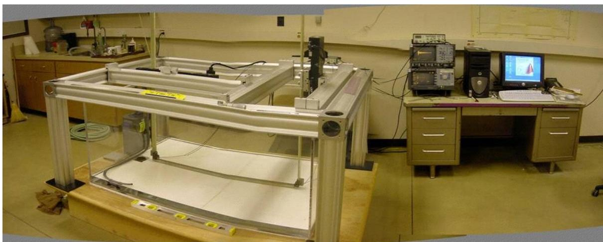
FIG. 2.14 : Cuve ultrasonore du Marine Physical Laboratory (MPL, San Diego).
