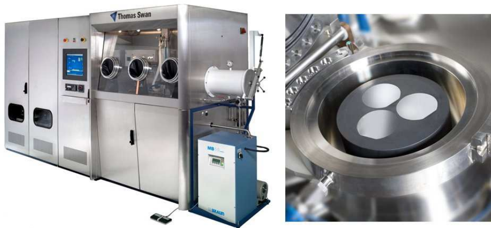
Figure 2.2 : The Thomas Swan (Aixtron) 3x2" CCS MOVPE reactor (left). View on the susceptor with three 2" substrates (right)
