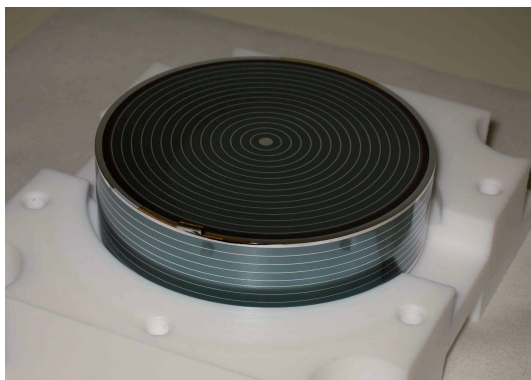
(e) Picture of a 400 g Fiducial Interdigitised Germanium detectors.
