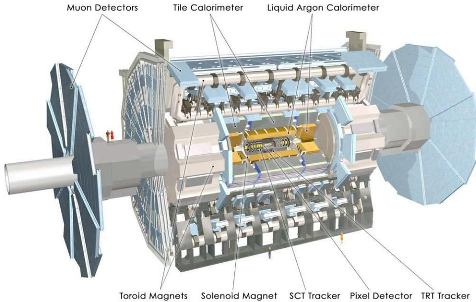
Figure 4.1: The ATLAS detectors and its sub-systems.
