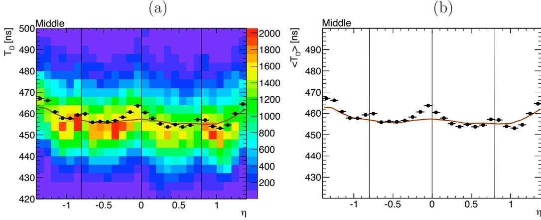
Figure 6.28: Drift time  $T_D$  as a function of  $\eta$  in the Middle, in bins of 0.1. Events are weighted by  $A_{max}^2$ . The black dots, displayed in (a) and (b), correspond to the Profile of the color plot. The orange line represents the prediction from absorber thickness measurements averaged in  $\phi$ .
