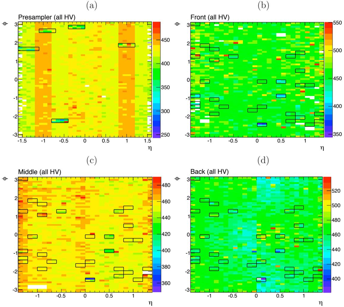
Figure 6.54:  $(\eta, \phi)$  map for TD (a) in the Presampler, (b) Front, (c) Middle and (d) Back, including all voltage configurations. The regions where the high voltage is lower than the nominal value are surrounded by black boxes. White zones correspond to regions of the detector where no data have been recorded.
