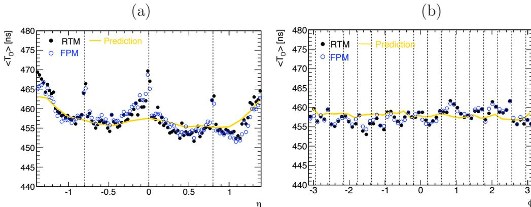
Figure 6.56: Distributions of  $T_D$  as function of (a)  $\eta$  and (b)  $\phi$  in the Middle obtained with the FPM and RTM methods. The prediction from absorber thickness measurements is also shown.
