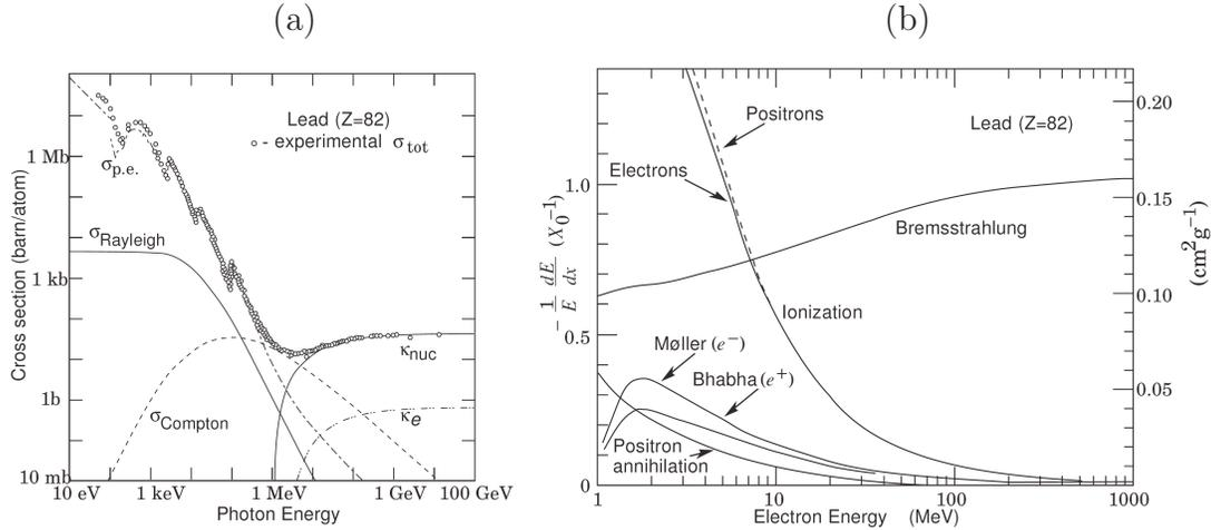
Figure 5.1: (a): Cross section of the photon interaction with matter as a function of its energy.  $\kappa_{nucl}$  and  $\kappa_e$  correspond to electron-positron pair creation by interaction with a nuclear and an electron, respectively. (b) Processes of electron interaction with matter as a function of its energy, per radiation length.
