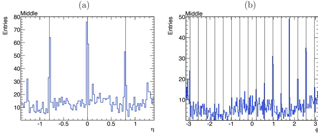
Figure 6.15:  $\eta$  and  $\phi$  distributions in the Middle, for events with  $TD > 550$  ns. The black lines represent the electrode and half-barrel transition zones in  $\eta$  and the inter-module separation in  $\phi$ .
