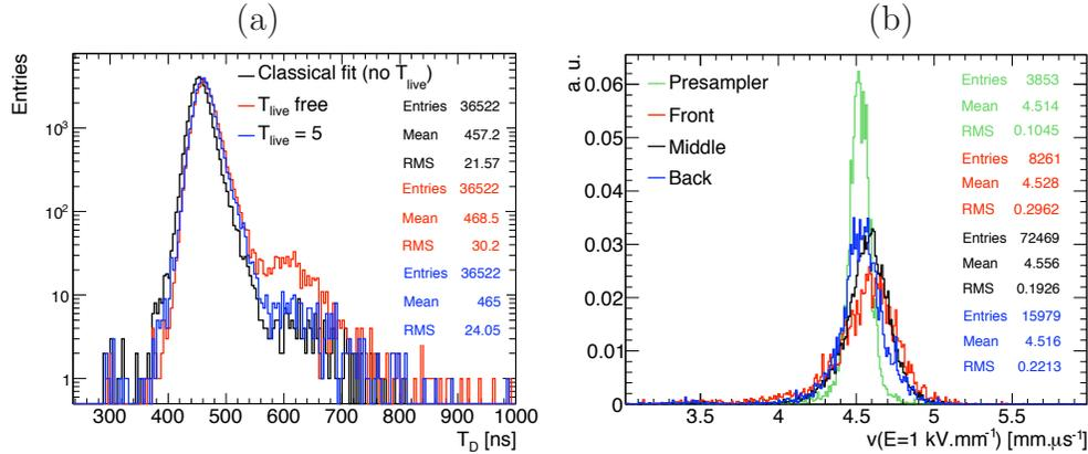
Figure 6.65: (a):  $T_D$  distributions: in black for the standard fit, in red for the fit with a free  $T_{live}$  parameter and in blue for the fit with  $T_{live}$  fixed to 5. (b): Drift velocity associated to a field of 1 kV/mm, for the fit with  $T_{live}$  free; in green for the Presampler, in red for the Front, in black for the Middle, and in blue for the Back.
