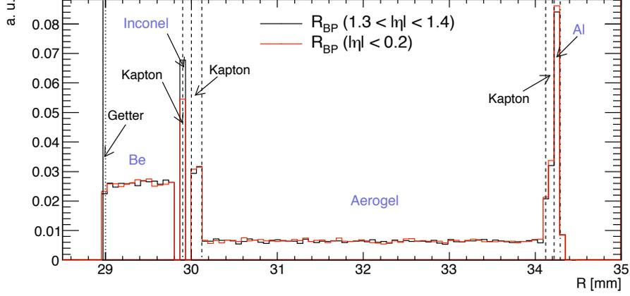
Figure 6.70: Radius of the Beam Pipe obtained with 7 TeV MC samples by counting the number of photon conversions with an energy greater than 1 GeV in red for  $|\eta| < 0.2$  and in black for  $1.3 < |\eta| < 1.4$ . The dashed lines separate the different components of the BP as quoted in the database of ATLAS.
