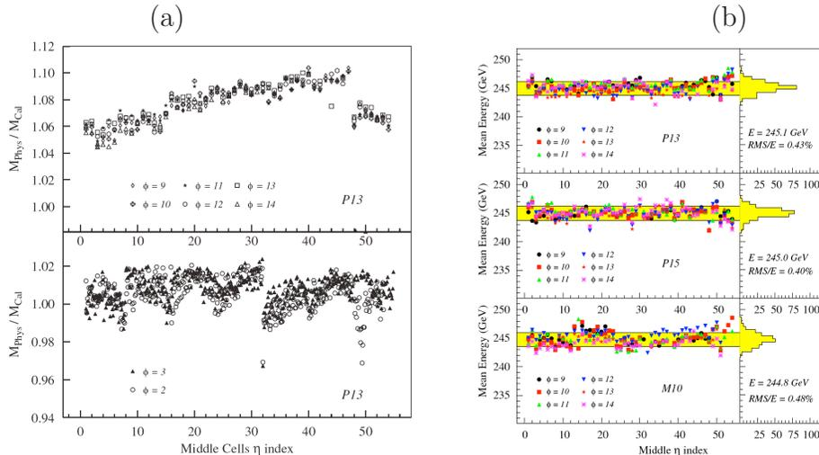
Figure 5.15: (a):  $M_{phys}/M_{cali}$  ratio as a function of the  $\eta$  index of the cells for the modules exposed to the test beam, for the Middle compartments on the top and the strips on the bottom. (b): Average reconstructed energy as a function of the  $\eta$  cell index. The RMS of the dispersion is quoted on the right. A dispersion better than 0.5% has been found in the three modules.
