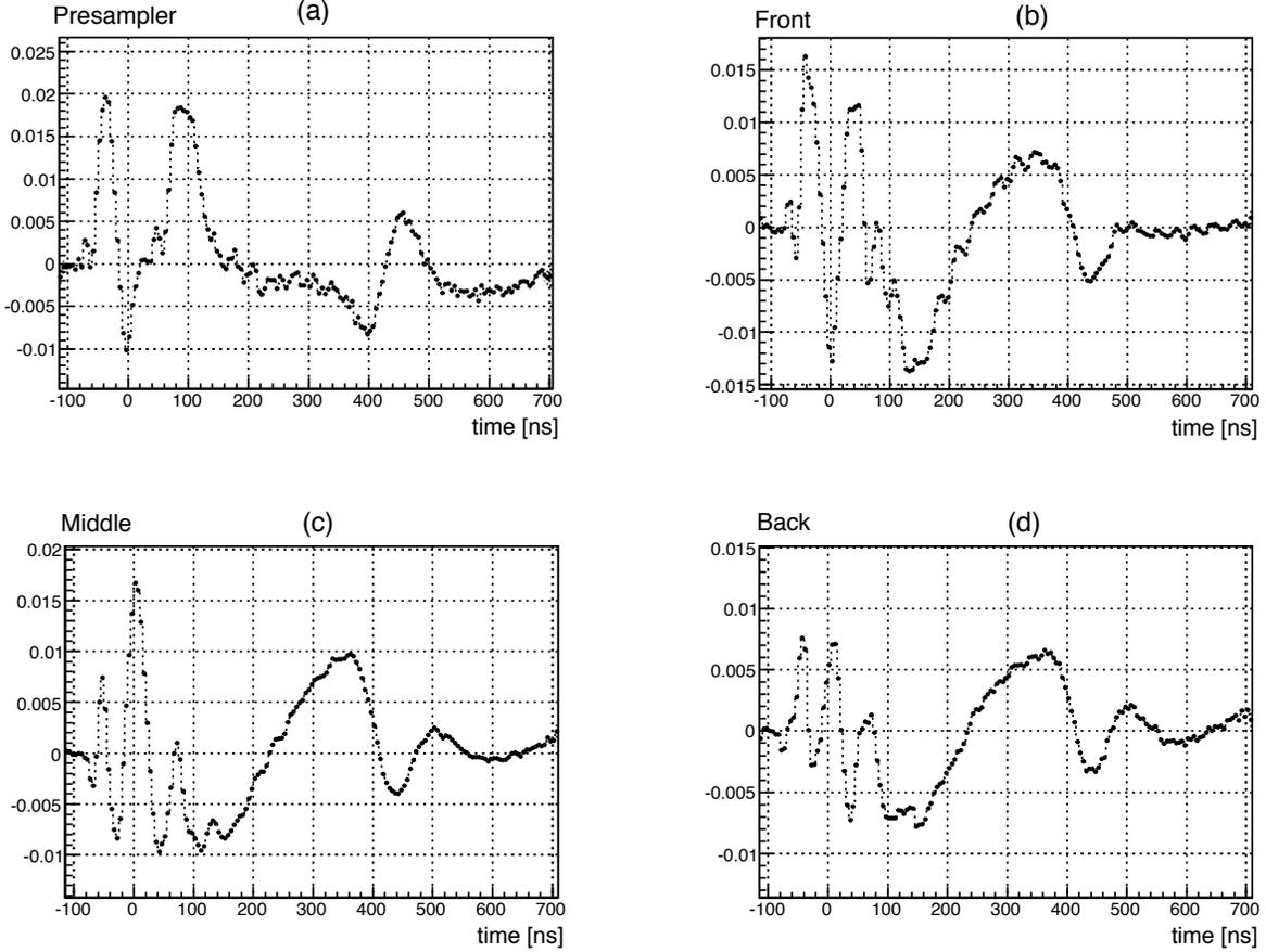
Figure 6.60: Profile of the normalized residuals  $(meas(i) - pred(i))/max(pred)$  as a function of time (equal to recorded time -  $t_{max(pred)}$ ) for events at nominal high voltage in: (a) Presampler, (b) Front, (c) Middle and (d) Back.
