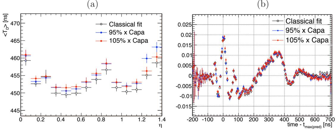
Figure 6.62: (a) Distribution of the average weighted  $T_D$  in bin of size 0.1 as a function of  $\eta$ . (b): Profile of the residual shapes, for different assumptions of capacitance for FT 25A in the Middle: in black the classical individual fit case, in blue and red for the capacitance decreased and increased by % respectively.
