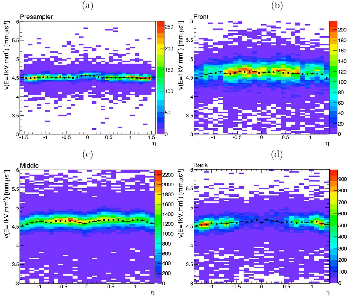
Figure 6.47: Drift velocity rescaled to an electric field  $E$  of  $1\text{kV}/\text{mm}$  in the Presampler and three barrel layers of the calorimeter, as a function of  $\eta$ . The selected events in this plots are at nominal voltage (2000 V).
