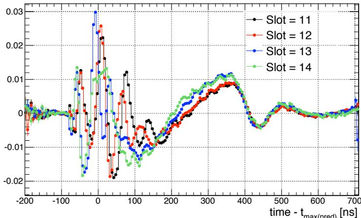
Figure 6.61: Profile of the normalized residuals  $(meas(i) - pred(i))/max(pred)$  as a function of Time (equal to recorded time -  $t_{max(pred)}$ ) for events with  $HV=2000V$  in different slots of the Middle: in black for Slot 11, in red for Slot 12, in blue for Slot 13 and in green for Slot 14.
