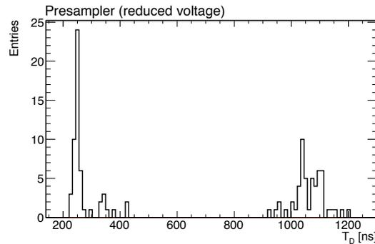
Figure 6.51: Distribution of the drift time in the Presampler in the case of reduced voltage.
