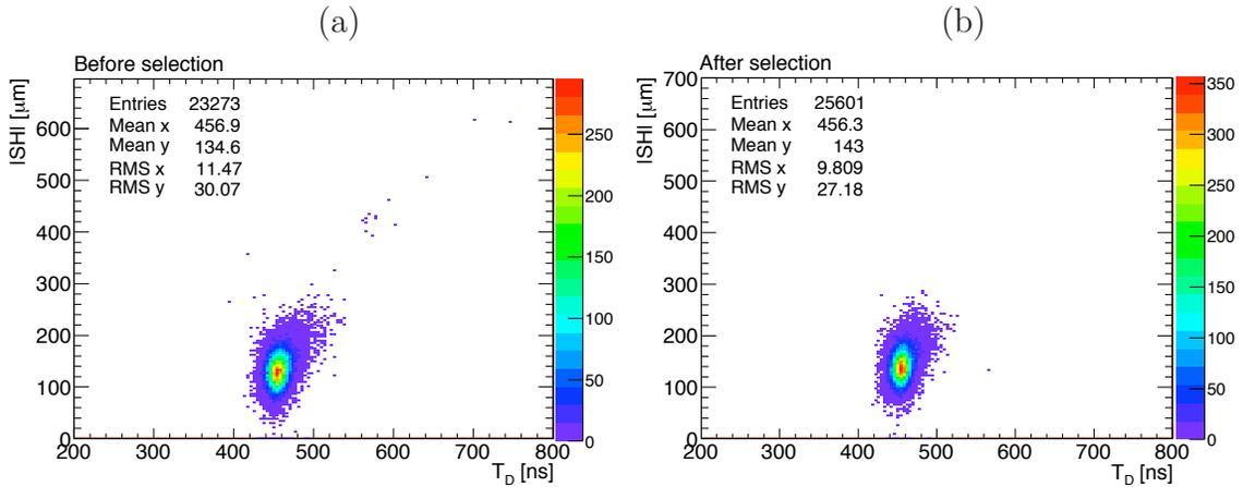
Figure 6.22:  $|SH|$  versus  $T'_D$  for the global cell based fit with  $N$  pulses in the Middle, (a) before and (b) after applying a fit quality selection in the same spirit as what was done in the individual fit case.
