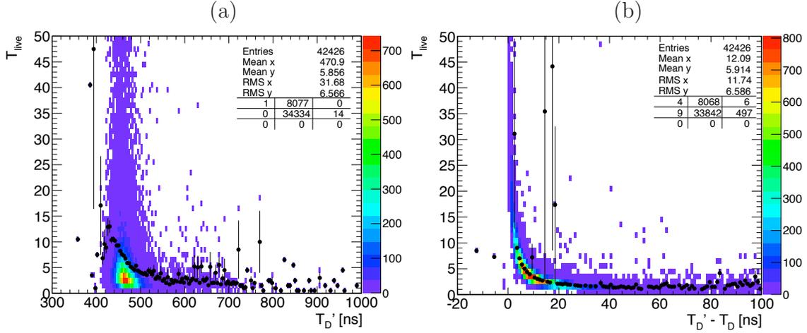
Figure 6.63: (a): Distribution of  $T_{live}$  as a function of the drift time  $T_D'$  for the the case with a free  $T_{live}$ . (b):  $T_{live}$  as a function of the difference between drift times with and without this new parameter in the fit.
