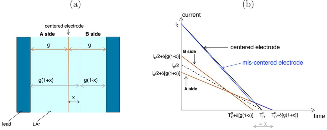
Figure 6.2: (a): Schematic view of the electrode shift (in the straight section) in LAr gap. The gaps are of size  $g(1 - x)$  and  $g(1 + x)$ ,  $x$  corresponding to the relative shift of the electrode with respect to its centered position. (b): The current collected by the electrode as a function of time is shown in the case of a centered electrode and when the electrode is shifted, as illustrated in (a).
