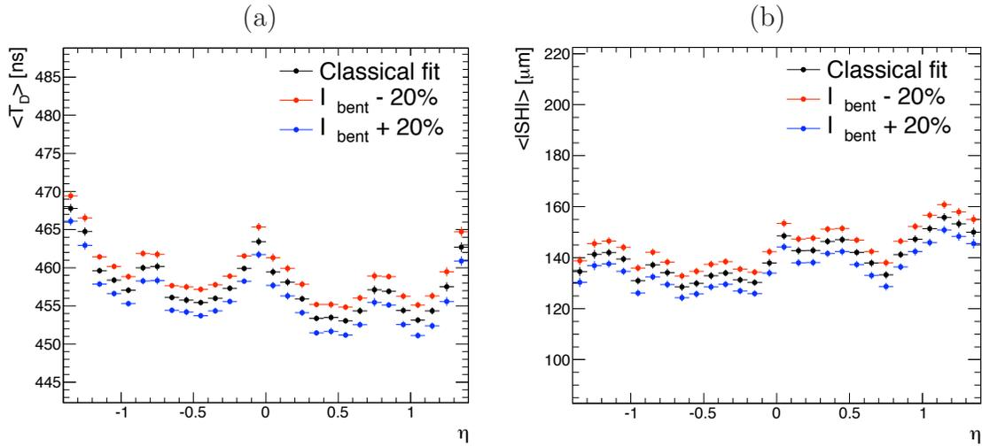
Figure 6.66: (a)  $T_D$  and (b)  $|SH|$  as a function of  $\eta$  in the Middle for different  $I_{bent}$  configurations: in black the standard case, in blue for  $I_{bent} + 20\%$  and in red  $I_{bent} - 20\%$ .
