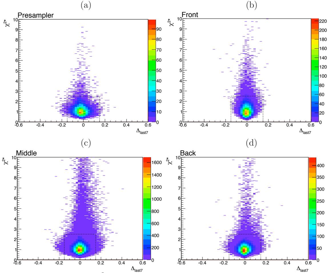
Figure 6.10: Distributions of  $\chi^{2*}$  as a function of  $\Delta_{last7}$  for the Presampler and the three barrel compartments. The black boxes represent the events passing the fit quality selection.
