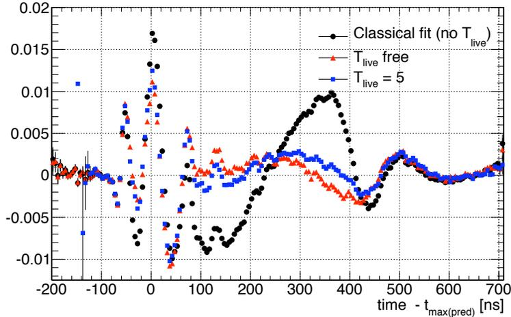
Figure 6.64: Profile of the normalized residual  $(meas(i) - pred(i))/max(pred)$  as a function of  $time$  (the maximum of the pulses are shifted to 0) in the Middle, in black for the standard fit, in red for the fits with  $T_{live}$  let free and in blue for the fits with  $T_{live}$  fixed to 5.
