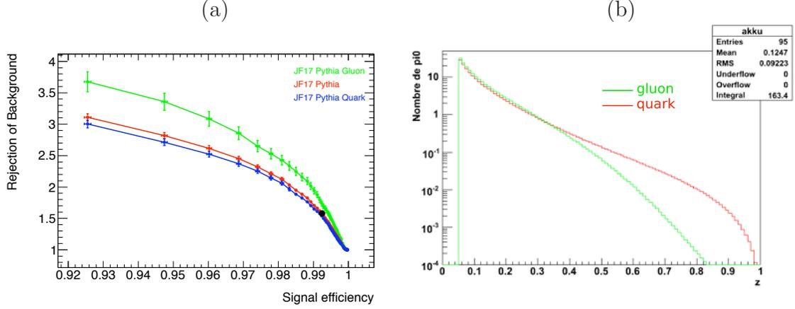
Figure 10.2: (a): Background rejection versus signal efficiency computed with Pythia  $\gamma$ -jet sample in red, for the jets originating from gluon or quark in green and blue respectively. The back point represents the selected threshold  $\sum_{Trks} P_T < 4 \text{ GeV}/c$ . (b): Quark and gluon probability of fragmenting into a  $\pi^0$  as a function of  $z = E_{\pi^0}/E_{q,g}$ .
