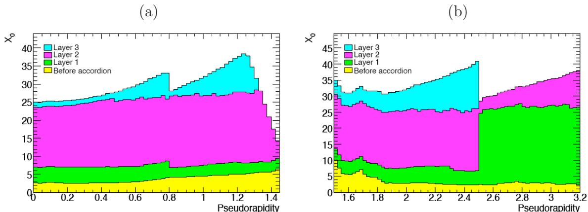
Figure 5.7: Distribution of the radiation length in as a function of  $\eta$  in the front of and in the different layers of the EM calorimeter, barrel part in (a), and end-cap in (b). At the transition between the barrel and end-cap, a large fraction of material causes important degradation in the measure of the energy.
