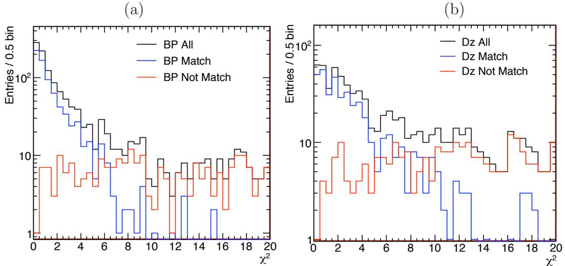
Figure 6.80: Distributions of the  $\chi^2$  of the reconstructed vertex of (a) BP conversions and (b) Dalitz decays, in black for all conversions passing the selection criteria, in red for these that match with the truth MC and in blue for the combinatorial background.
