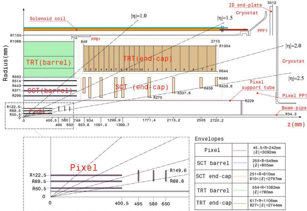
Figure 4.3: View of a quarter of the ID barrel and end-cap subsystems, in the  $R-z$  plan. The design of the ID in terms of layers in the barrel and end-cap regions and the separation of these regions is a compromise between available space and the minimal number of hits per charged particle for any kind of direction.
