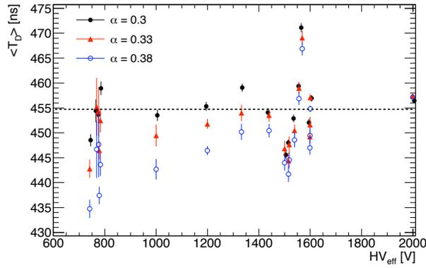
Figure 6.49: Corrected drift time  $T_D$  as a function of the effective high voltage, in the Middle. The black dots correspond to the case  $\alpha = 0.3$  in the relations 6.5-6.8, the red triangles to  $\alpha = 0.33$  and the blue open dots to  $\alpha = 0.38$ .
