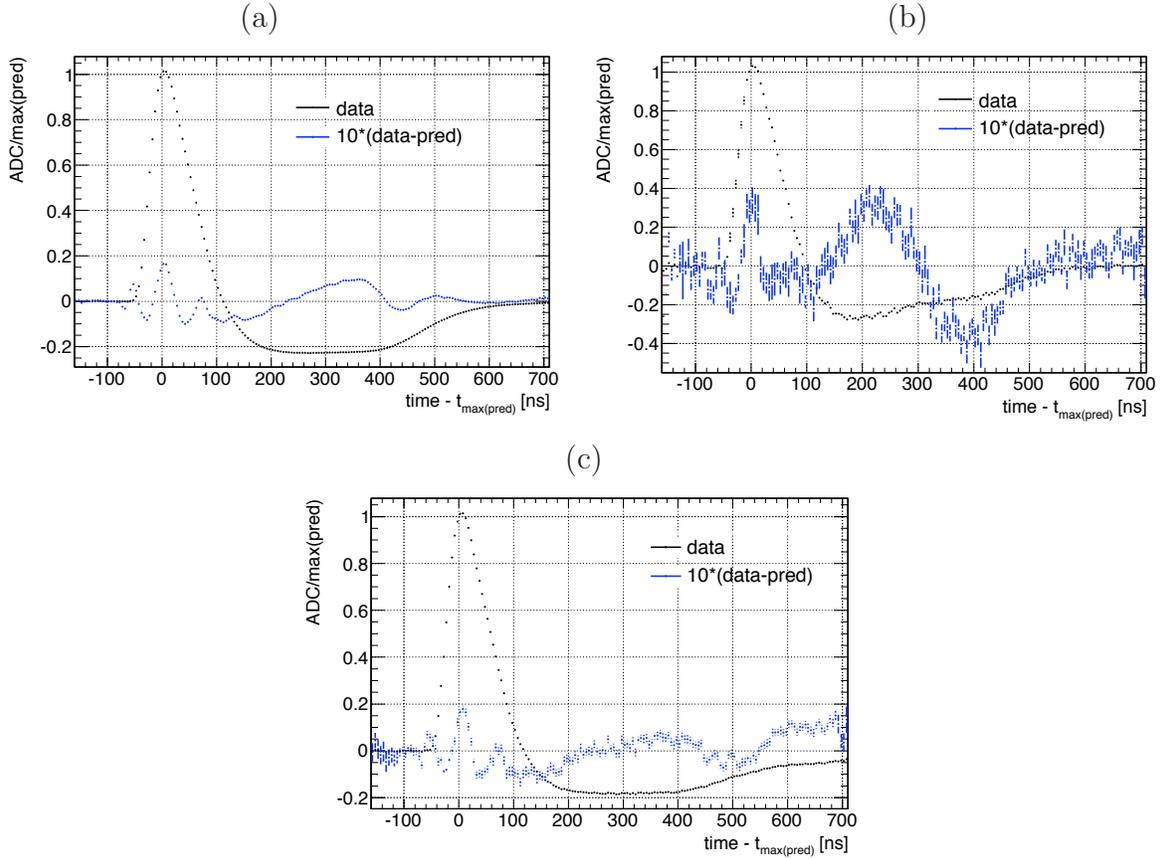
Figure 6.14: Profile of the normalized residuals multiplied by a factor 10 (in blue) as a function of time, to be compared to the normalized data (in black) in the Middle for 3 different  $T_D$  zones: (a)  $380 < T_D < 550$  ns, (b)  $T_D < 380$  ns (bulk of the events) and (c)  $T_D > 550$  ns.
