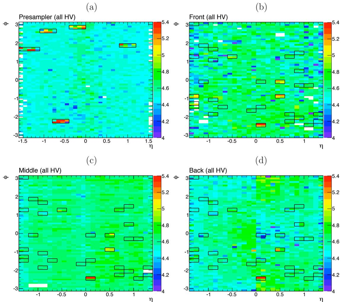
Figure 6.55:  $(\eta, \phi)$  map for the Drift velocity rescaled to a field of 1 kV/mm, in (a) the Presampler, (b) the Front, (c) the Middle and (d) the Back. The regions where the high voltage is lower than the nominal value are surrounded by back boxes.
