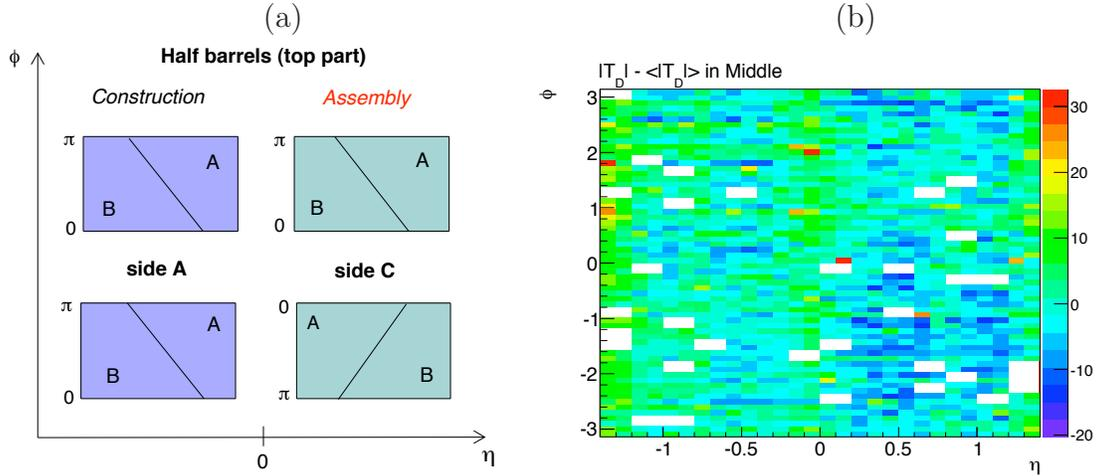
Figure 6.33: (a): schematic view of the half barrels construction and assembly in the  $(\eta, \phi)$  plane. (b):  $(\eta, \phi)$  map in which the difference between the local weighted average  $T_D$  and  $\langle T_D \rangle$  the global average is plotted per bin of size  $(0.1, 0.1)$ . White rectangles correspond to areas where the HV is not nominal or where no data have been recorded.
