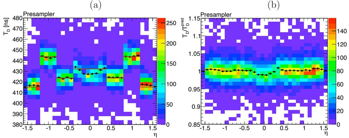
Figure 6.43: (a): Distribution of the drift time as a function of  $\eta$  in the Presampler, with  $A_{max}^2$  weight. The black dots correspond to the Profile of the color plot. In addition, the orange line represents the prediction starting from the region  $0.8 < |\eta| < 1.2$ , using the relation 6.16 and the gap values given in Table 6.6. (b): Distribution of the drift time  $T_D$  divided by the predicted value, as a function of  $\eta$ .
