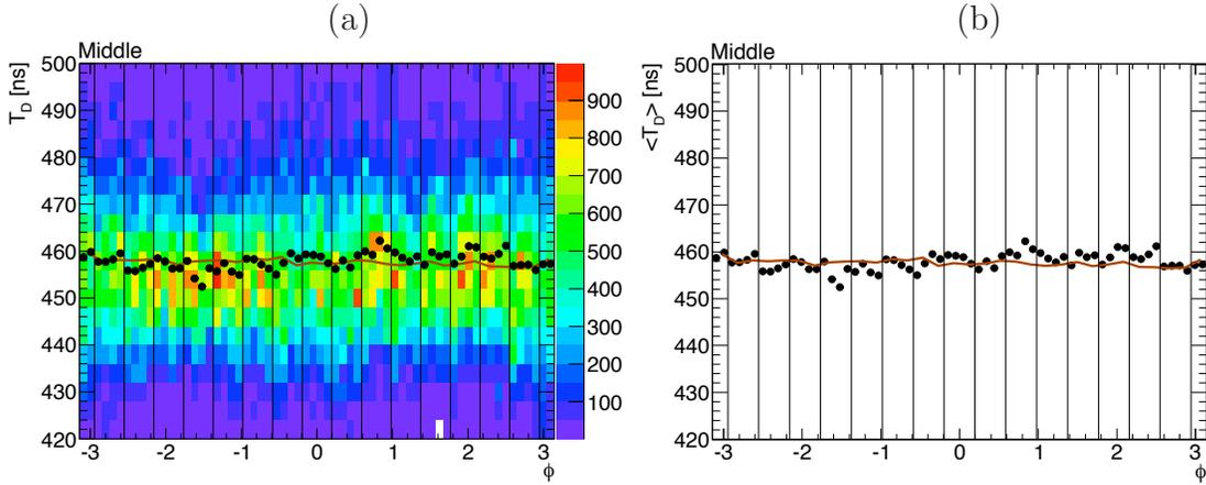
Figure 6.31: Distribution of the drift time as a function of  $\phi$  in the Middle. Events are weighted by  $A_{max}^2$ . The black dots correspond to the Profile of the color plot, they are displayed in (a) and (b). In addition, the orange line represents the prediction from absorber thickness measurements averaged in  $\eta$ . The vertical black lines represents the module separations.
