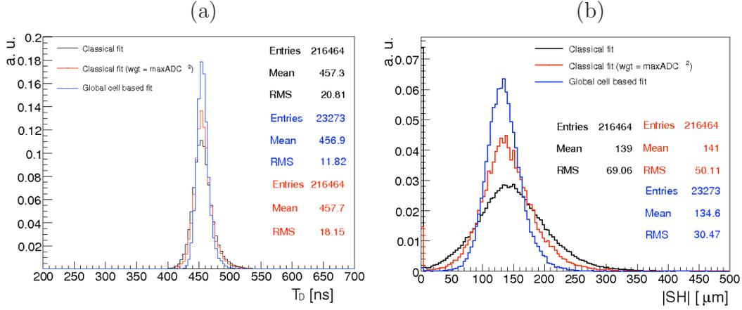
Figure 6.25: Distributions of (a) the drift time and (b) the absolute shift in the Middle, in black for the individual fit, in red for the individual fit weighted by  $A_{max}^2$ , and in blue for the global cell based fit methods.
