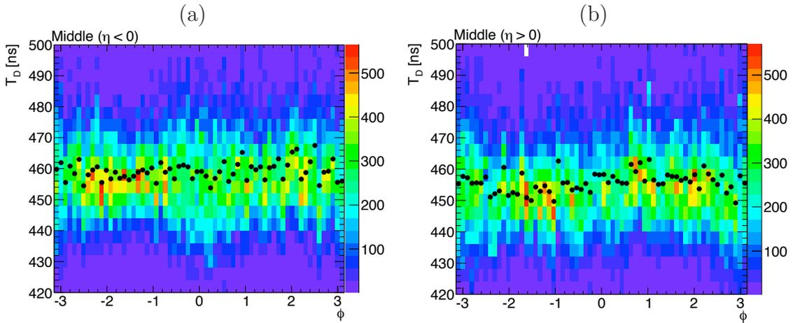
Figure 6.32: Drift time as a function of  $\phi$  in the Middle, for (a)  $\eta < 0$  (C wheel) and (b)  $\eta > 0$  (A wheel). Events are weighted by  $A_{max}^2$ . The black dots correspond to the Profile of the color plot.
