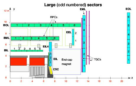
Figure 4.9: Sketch of the muon spectrometer in ATLAS detector. The precision measurement chambers, MDT and CSC, respectively in the barrel and end-cap parts are shown as well as the RPC and TGC chambers, dedicated to the trigger (Level1).
