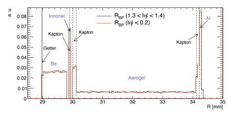
Figure 6.70: Radius of the Beam Pipe obtained with 7 TeV MC samples by counting the number of photon conversions with an energy greater than 1 GeV in red for  $|\eta| < 0.2$  and in black for  $1.3 < |\eta| < 1.4$ . The dashed lines separate the different components of the BP as quoted in the database of ATLAS.
