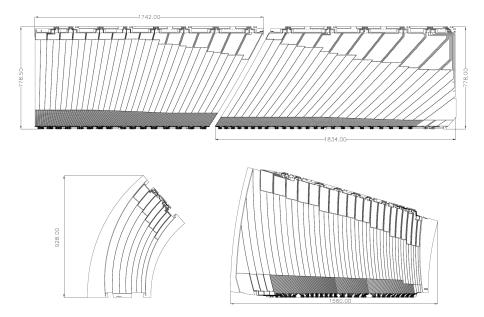
Figure 5.4: (b): Longitudinal segmentation of the EM calorimeter barrel and end-cap.
