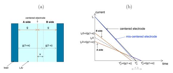
Figure 6.2: (a): Schematic view of the electrode shift (in the straight section) in LAr gap. The gaps are of size g(1-x) and g(1+x), x corresponding to the relative shift of the electrode with respect to its centered position. (b): The current collected by the electrode as a function of time is shown in the case of a centered electrode and when the electrode is shifted, as illustrated in (a).
