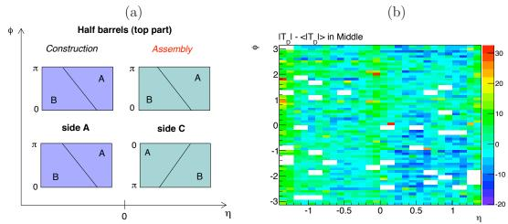
Figure 6.33: .(a):schematic view of the half barrels construction and assembly in the  $(\eta, \phi)$  plane. (b):  $(\eta, \phi)$  map in which the difference between the local weighted average  $T_D$  and  $\langle T_D \rangle$  the global average is plotted per bin of size (0.1, 0.1). White rectangles correspond to areas where the HV is not nominal or where no data have been recorded.
