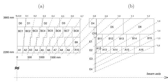
Figure 4.6: Segmentation in depth and  $\eta$  of the barrel (a) and extended barrel (b) of the Tile Calorimeter.
