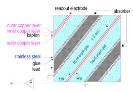
Figure 5.5: Sketch of the lead-LAr-lead sampling in the EMB (straight section).
