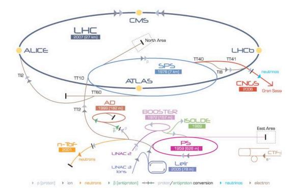
Figure 3.1: The CERN accelerator complex. Once injected in the LHC, the proton beams are accelerated to reach the 7 TeV energy and collide in four different points, where ATLAS, ALICE, CMS and LHCb experiments are installed.
