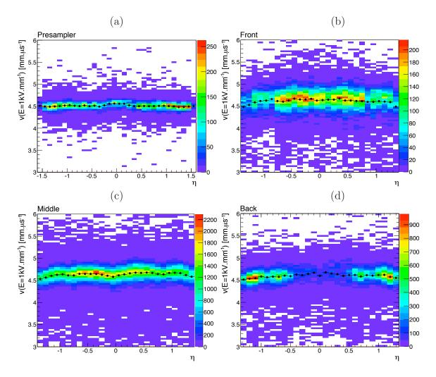
Figure 6.47: Drift velocity rescaled to an electric field E of 1kV/mm in the Presampler and three barrel layers of the calorimeter, as a function of  $\eta$ . The selected events in this plots are at nominal voltage (2000 V).
