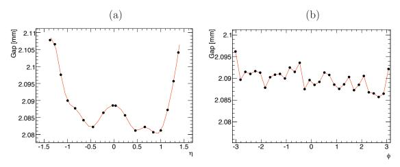
Figure 6.29: Variation of the gap in the Calorimeter along (a) the  $\eta$  and (b) the  $\phi$  directions, calculated from the measured absorbed thicknesses.
