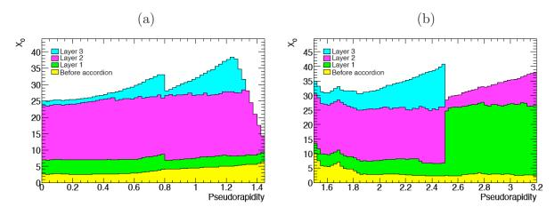
Figure 5.7: Distribution of the radiation length in as a function of  $\eta$  in the front of and in the different layers of the EM calorimeter, barrel part in (a), and end-cap in (b). At the transition between the barrel and end-cap, a large fraction of material causes important degradation in the measure of the energy.
