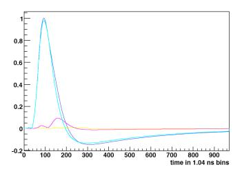
Figure 5.13: Typical calibration signal shape. The direct, first reflection and two reflections components of the signal are illustrated.
