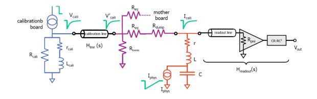
Figure 5.12: Sketch of the electronic chain; the ionization signal is represented by a current  $I_{phys}$  following a (r,L,C) circuit; the calibration signal  $V_{cali}$  is generated in the calibration board outside the cryostat and routed inside through inductive cables.
