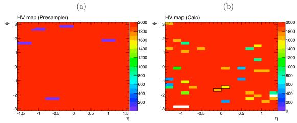
Figure 6.7: HV map in  $(\eta, \phi)$  for (a) the Presampler and (b) the Calorimeter. Black boxes in b) indicate the region where the HV is reduced on both sides of the electrode, otherwise the second side is always at nominal voltage.
