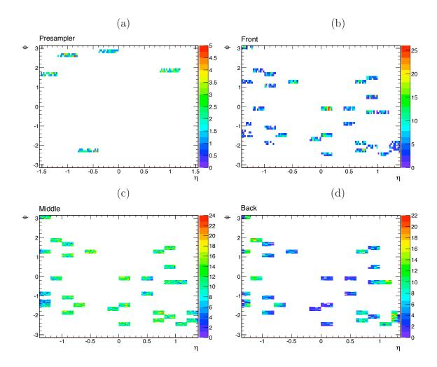
Figure 6.6: Coverage for the reduced voltage case, in: (a) Presampler, (b) Front, (c) Middle and (d) Back.
