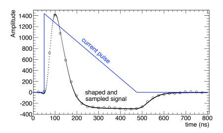
Figure 5.10: Example of ionization current and bipolar shaped sampled signal in time.
