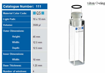
Figure 3.10: Quartz cuvettes from Hellma, suitable for IUVS experiments. The viton O-ring is inserted as a gasket around the stopper, which is pressed in order to prevent sample evaporation into the 10^{-7} mbar sample chamber.
