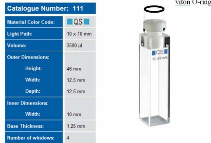
Figure 3.10: Quartz cuvettes from Hellma, suitable for IUVS experiments. The viton O-ring is inserted as a gasket around the stopper, which is pressed in order to prevent sample evaporation into the 10^{-7} mbar sample chamber.
