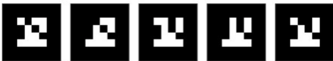
Figure 3.6: Examples of fiducials/markers used for pose estimation in AR applications
