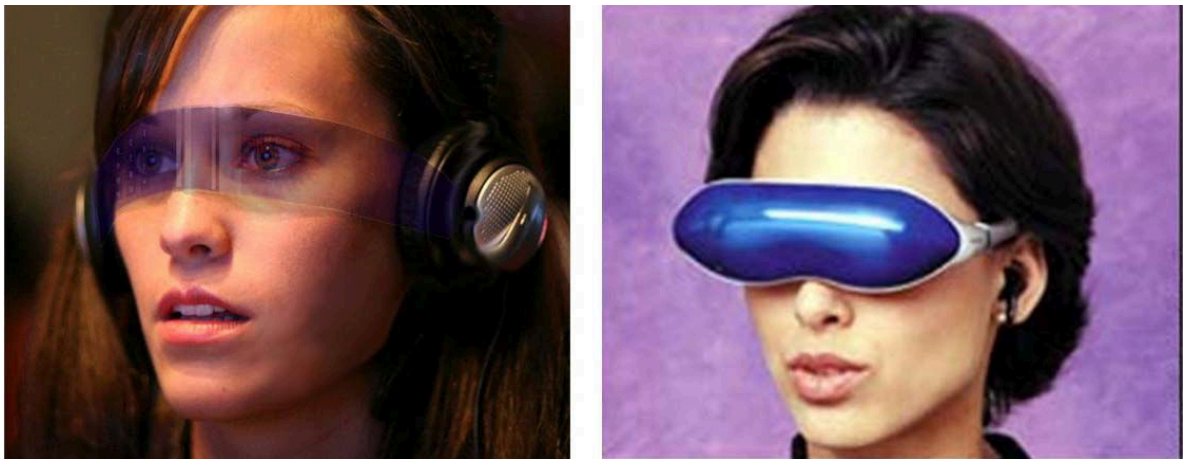
Figure 3.8a-3.8b: A. Mockup of lightweight optical display (Low, October 27th, 2008) and B. The Sony Glasstron video see-through display (CNN, February 2, 2000)
