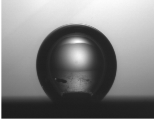
Figure 4.3.9: Stable bubble growth: when the bubble becomes larger than the capillary length, the hypothesis of spherical shape is not valid anymore. The pressure is larger at the bottom, creating the buoyancy force. The real bubble is taller than predicted by the model
