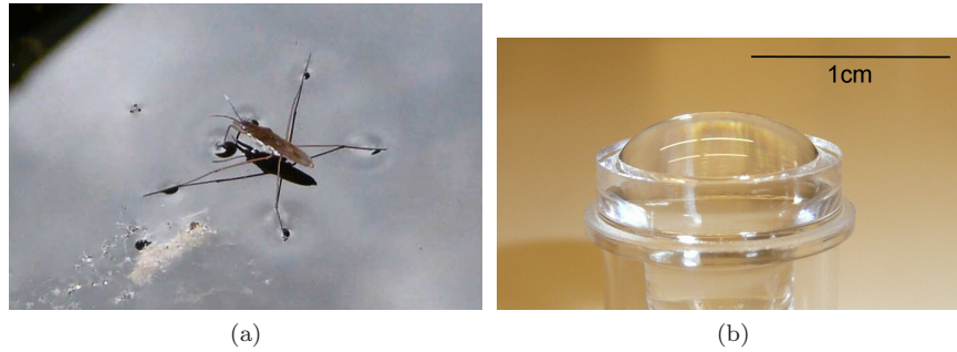
Figure 3.1.1: Illustration of surface tension. (a) An insect, called water strider, is able to float on the surface of water because surface tension compensates its weight. (b) It is possible to fill a container slightly above its rim without creating an overflow, because surface tension confine the liquid
