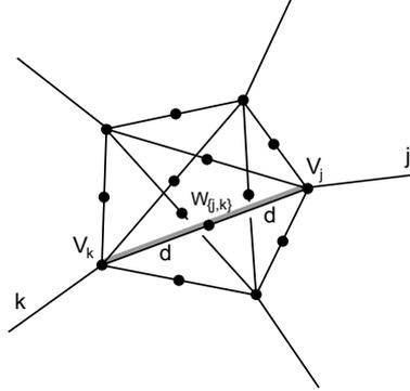
Figure 1: The scheme of the approximation. All inner links are of length  $2d$ . Some connection links may be missing if the conditions given in the text are not satisfied. The quantities corresponding to the index pair  $\{j, k\}$  are marked, and the grey line symbolizes the vector potential  $A_{(j,k)}(d)$ .
