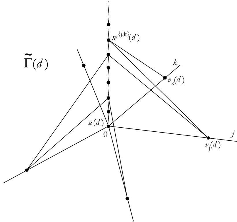
Fig. 2. Approximating graph: A star amended by connections of the edges, with a  $\delta$  coupling in the center, one  $\delta$  coupling at each edge and one  $\delta$  interaction at each (broken) connection segment.
