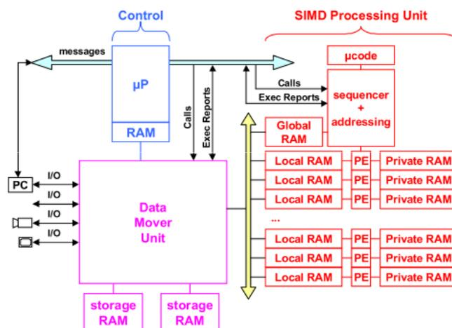
FIGURE 2.6 – Circuit Ter@Core [14]
