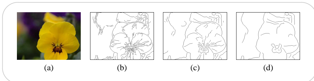
Figure 5.1: Edge importance. (a) The input image. (b-d) Canny edges at increasing scales.
