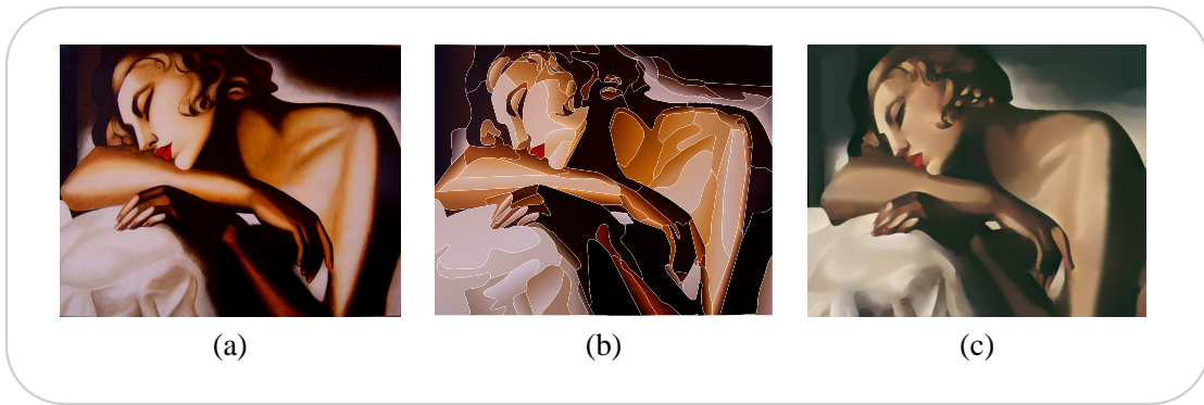
Figure 5.8: Comparison with Ardeco [LL06]: (a) original image; (b) the vectorization result. Note that, while the gradient inside regions is well approximated, sharp transitions between regions are noticeable. Image taken from [LL06]. (c) Our result. Note that the smooth color transition is preserved both along and across the geometric curves.
