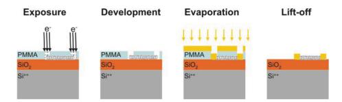
Figure 3.3: The four-step lithographical process which we use for nanofabricating our devices. As an example, the last lithography step is illustrated. In this step the Single-Walled Carbon Nanotube is contacted and connected to metallic leads.
