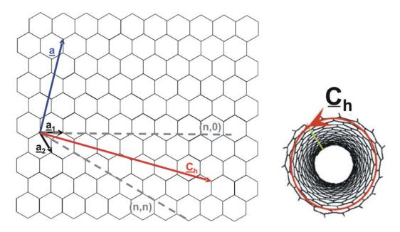
Figure 2.1: (Left) The lattice of graphene is spanned by two primitive lattice vectors  $\vec{a}_1$  and  $\vec{a}_2$ . The index numbers n and m define the chirality of a tube which contains information on diameter and material properties. (Right) The chirality vector  $\vec{C}_h$  describes the axis along which the graphene sheet is rolled up to form a nanotube.
