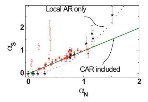
Figure 4.15: We plot  $\alpha_S$  as a function of  $\alpha_N$  for both triple points and single resonances. As expected, single resonances fall on a parabola whereas triple points fall on a linear function. This proves the existence of CAR in our beamsplitter device.
