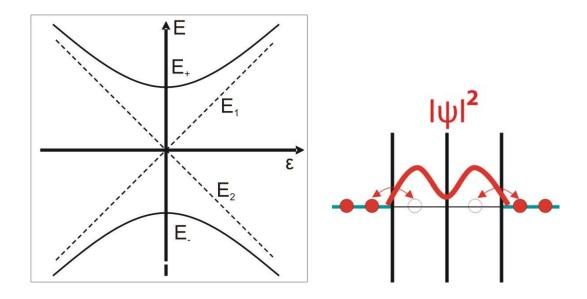
Figure 2.9: (Left) When tunnel coupling between the two dots of a double quantum dot is introduced, the single dot energies  $E_1$ ,  $E_2$  repel each other and form an anticrossing with energies  $E_+$ ,  $E_-$ . (Right) The new energy levels, referring to bonding and antibonding wave-function of a molecular state, are delocalized over the quantum dot. The square of the wave-functions describing the molecular state is the probability distribution where to find an electron.
