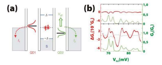
Figure 5.1: (a) The measurement method of the Basel group: In the middle-injection setup, the differential conductance is measured at 1st and 2nd lead. The 1st quantum dot is held at resonance while the 2nd dot is swept through a conductance resonance. (b) The additional conductance measured at the 1st lead is attributed to CAR. (Figures taken from reference [116])
