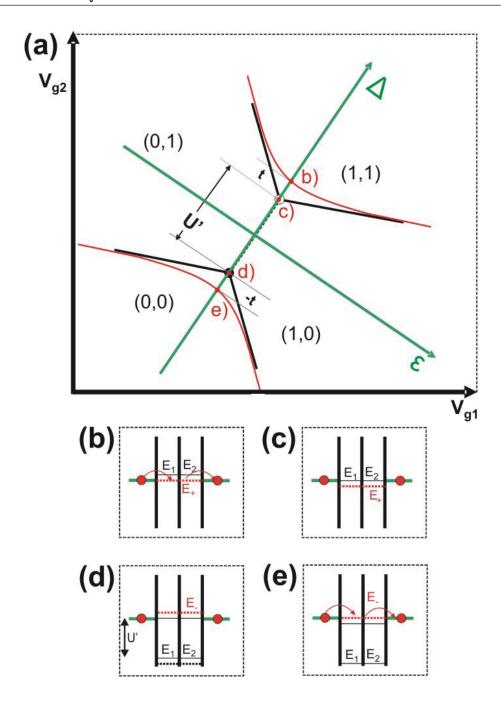
Figure 2.11: In real double quantum dots, the separation of the anticrossing lines has two reasons: Electrostatic coupling and tunnel coupling.
