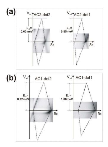
Figure 4.18: (a) The finite bias Coulomb diamonds in the middle-injection setup along AC2 for both dots of the double quantum dot are depicted here. (b) Similar measurement as above along AC1.
