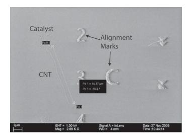
Figure 3.2: A typical Single-Walled Carbon nanotube as grown in our systems. It has a length of roughly  $14\mu m$  and grows from a catalyst spot. Catalyst spots are typically around  $1-2\mu m$  in size.
