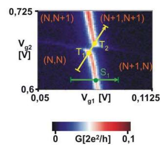
Figure 4.12: Stability diagram of a typical anticrossing in the middle-injection setup. The yellow arrow defines the scanning direction across two adjacent triple points  $T_1$  and  $T_2$ . We measure the zero bias conductance at left and right lead simultaneously, following the indicated direction. The same is carried out for the single resonance  $S_1$ .
