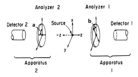
Figure 1.2: Setup to illustrate the Einstein-Podolsky-Rosen Gedankenexperiment, taken from Clauser and Horne [31].
