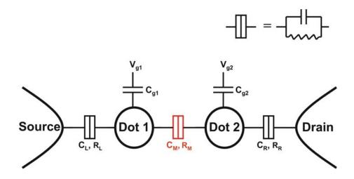
Figure 2.6: Electrical circuit representation of a double quantum dot: The coupling capacitance  $C_M$  and the coupling resistance  $R_M$  are the decisive elements for the electronic behavior of the dot.
