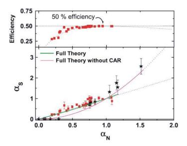
Figure 4.20: We show the splitting efficiency of our Carbon Nanotube beamsplitter for every triple point presented in figure (4.15). Splitting efficiencies up to 50 per cent are reached.
