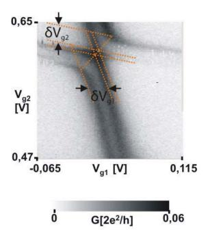
Figure 4.7: The anticrossing presented in figure 4.6(b) at  $V_{bias} = 200 \mu V$ . The parameters  $\delta V_{g1}$  and  $\delta V_{g2}$  allow to calculate the charging energy of 1st and 2nd dot.
