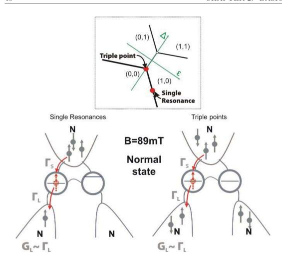
Figure 2.18: At B=89mT, the Aluminum contact is in the normal state. Hence only single particle tunneling contributes to transport and the conductance measured at the left lead is proportional to the coupling energy of the left lead. Therefore it makes no difference if we measure the conductance at a single resonance or at a triple point.
