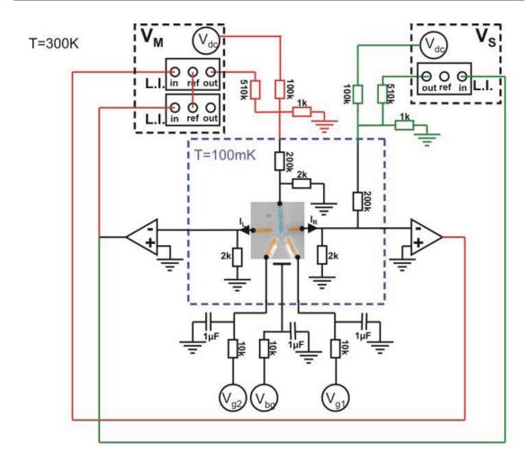
Figure 3.5: Our two different injection schemes are illustrated in this figure. We either inject at one of the side normal contacts  $(V_S)$  or at the superconducting contact in the middle  $(V_M)$ . In both cases we apply a voltage which induces a current through the nanotube. The current is changed into voltage by the two grounded resistors mounted adjacent to the normal leads. We then amplify the voltage and measure it with standard Lock-In technique.
