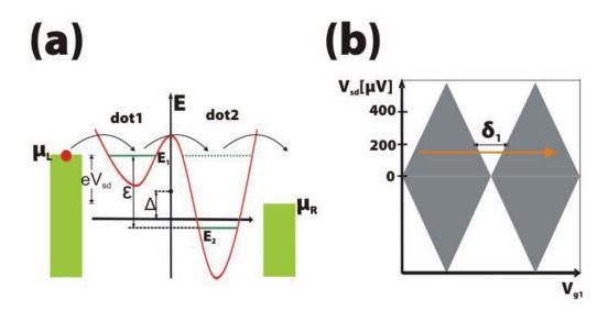
Figure 4.9: (a) If the detuning of  $E_1$  and  $E_2$  becomes big, no molecular state develops. That means that the double quantum dot behaves like a single quantum dot far away from the triple points. The second dot is traversed by co-tunneling. (b) We obtain Coulomb-diamonds as a function of applied  $V_{sd}$  and  $V_{g1}$ . The second quantum dot can be interpreted as part of the right contact.
