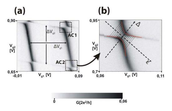
Figure 4.6: (a) The dimensions of the honeycomb cells define the gate capacitances. Furthermore the charging energy can be extracted. (b) The separation of the two anticrossing lines along the axis of detuning  $\epsilon$  gives insight in both electrostatic and tunnel coupling.
