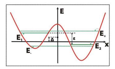
Figure 2.10: Double-well potential of a double quantum dot. At high interdot tunnel coupling, the two single-dot energy levels  $E_1$  and  $E_2$  form bonding and antibonding state  $E_{\pm}$ .
