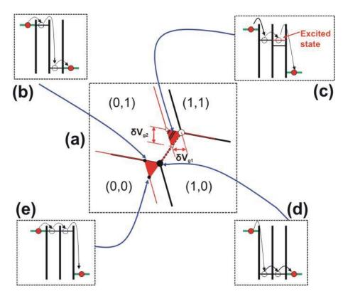
Figure 2.8: (a) At finite bias triple points split into triangular regions. (b),(d),(e) A detailed analysis of the mutual position of the energy levels explains how these enlarged resonances are possible. (c) If bias is sufficiently high, excited states contribute to transport.
