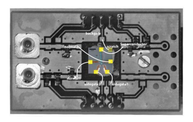
Figure B.1: The Printed-Circuit-Bord used for our measurements. To illustrate how the sample was mounted on chip, a sketch of the sample is put in the middle of our sample holder. The contact pads of the sample contacts are bonded to the respective pads of the PCB. Note that at the corner of the sample we scratch the wafer and thus destroy the oxide layer between surface and bulk. We can thus connect the backgate of the chip with a contact pad on our sample holder.
