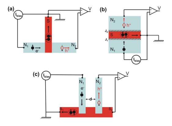
Figure 2.14: Crossed Andreev Reflection illustrated in three different sample geometries. Sample (a) describes the beamsplitter setup (topview), sample (b) describes the sample used by Russo et al. [100](crosssection) and sample (c) describes the sample of Eichler et al. [101] (topview).
