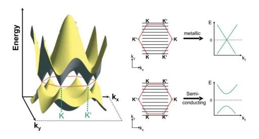
Figure 2.2: (Left) The tight binding calculation of the bandstructure of graphene. (Taken from http://www.als.lbl.gov/pics/154graphene01.png and modified). (Right) Zone folding leads to an additional quantization in  $k_{\perp}$  direction. Only if the line-cuts intersect with K and K' the nanotube is metallic. Otherwise a gap develops and the tube is semiconducting.
