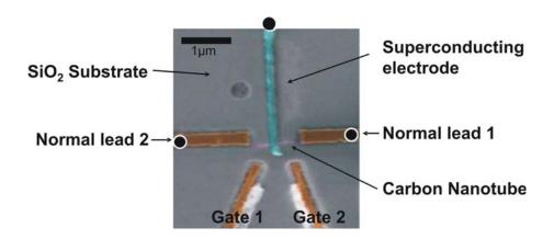
Figure 3.1: A typical Single-Walled Carbon nanotube beamsplitter sample. The different parts of the sample are illustrated by false colours. The picture was taken with a standard Scanning Electron Microscope.
