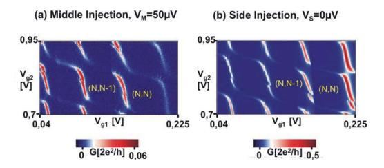
Figure 4.5: This figure shows the equivalence of the line shapes within the stability diagram in middle- and in side-injection. In (a), the middle-injection pattern is depicted. In comparison to the side-injection pattern (b), it is shifted a little bit down and to the left. Otherwise it is completely equivalent.
