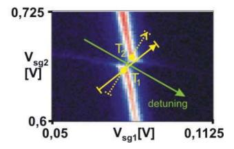
Figure 4.19: In case of the measurement of AC2 presented in figure (4.13), the gate trajectory illustrated by the yellow solid line is slightly tilted. The direct trajectory would correspond to the dashed line.
