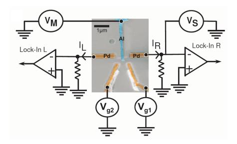
Figure 4.2: In this figure, our two different injection schemes are illustrated. We either inject at one of the side normal contacts  $(V_S)$  or at the superconducting contact in the middle  $(V_M)$ . We use side-injection to characterize our sample as a double quantum dot. In the middle-injection setup we show the injection and splitting of Cooper pairs.
