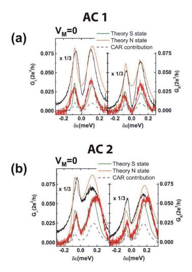
Figure 4.17: We calculate the zero bias conductance at the triple points at middle-injection in the superconducting (green curve) and normal (orange curve) state. We compare the results to our measurements presented in figure (4.13). The dashed black line quantifies the contribution from CAR to the total transport as extracted by Alfredo Levy-Yeyati's theory.
