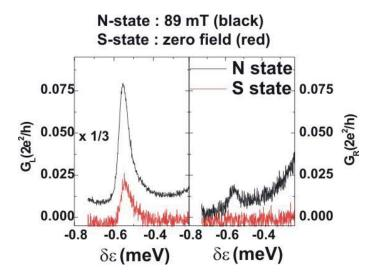
Figure 4.14: We measure the zero bias conductance across the single resonances, as shown in figure 4.12. Data for one typical single resonance is shown. The normal state is represented by the black line (scaled down in the figure) whereas the data in the superconducting state is given by the red line. Most importantly, the conductance ratio between left and right lead changes if we switch from the normal to the superconducting state.
