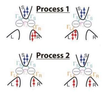
Figure 2.17: The figure illustrates the competing processes in our double dot beam-splitter. Process 1 shows how both electrons of an incoming Cooper pair tunnel to the same normal contact. Process 2, on the contrary, illustrates Crossed-Andreev Reflection.
