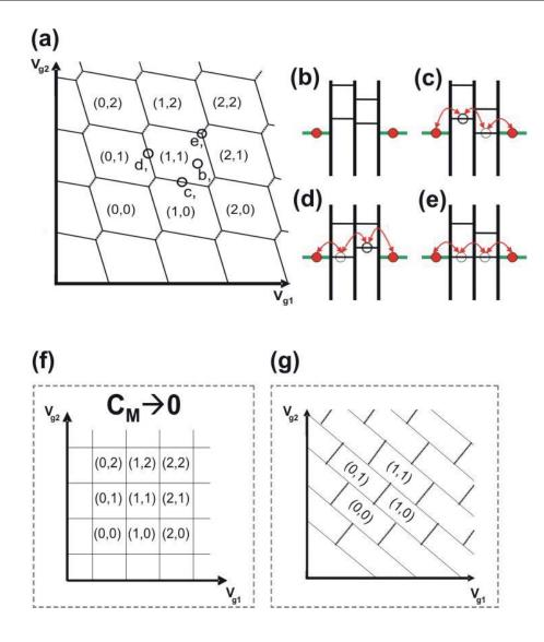
Figure 2.7: (a) A typical honeycomb stability diagram is shown here. Each honeycomb cell has a fixed number of electrons on left and right dot. (c)-(f) The corresponding energy level diagrams for the different transport configurations of the double dot. (g) Stability diagram of the double dot for  $C_M \to 0$ . (f) Stability diagram for very high capacitive interdot coupling.
