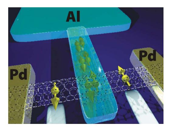
Figure 4.1: The Carbon Nanotube beamsplitter: A Single-Walled Carbon Nanotube is connected to two normal metal leads (Pd or Ti/Au) and a third, superconducting electrode in the middle (Al). The nanotube parts in-between two contacts act as a quantum dot. Hence the whole system is a double quantum dot attached to a superconducting reservoir.
