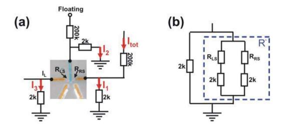
Figure 4.4: (a) In the side-injection setup, the total injected current splits into three branches. (b) Equivalent circuit scheme of the side-injection setup.
