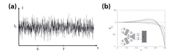
Figure 5.2: (a) Typical current noise spectrum as a function of time (taken from [118]). (b) Current-current noise correlations at both ends of the nanotube as a function of the transparency  $\epsilon$  between superconductor and nanotube (taken from [70]).
