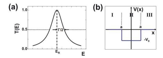
Figure 2.20: (a) The line shape of the transmission probability around a resonance  $E_R$  is given by the so-called Lorentzian or Breit-Wigner function. (b) In a very basic approach, a quantum dot can be modeled as a potential well.
