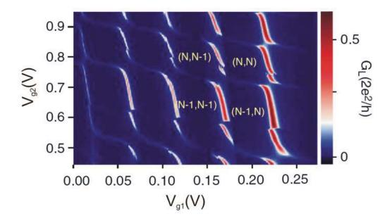
Figure 4.3: Typical stability diagram of our samples. The yellow number insets define the number of electrons on 1st and 2nd dot, respectively.
