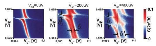
Figure 4.8: Stability diagram of the same anticrossing at B=90mT at three different bias voltages. The line splitting increases as a function of the bias voltage.
