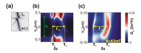
Figure 4.21: (a) The scanning direction is defined as the trajectory across the anticrossing AC2. (b) Finite bias dependence of the differential conductance measured at the left normal lead in the middle injection setup in the superconducting state. (c) The measurement is repeated in the normal state, at B = 63mT.
