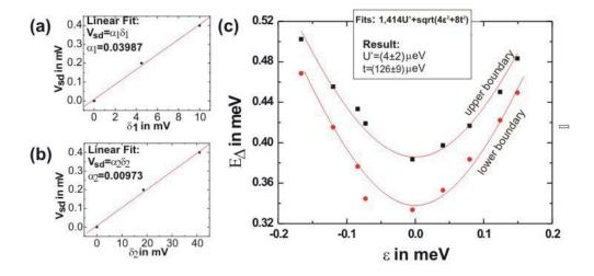
Figure 4.10: (a),(b) The line splitting as a function of bias voltage defines the conversion factors of the two gate voltages to the absolute energy scale. (c) The separation of the two anticrossing lines allows the determination of both tunnel and electrostatic coupling between the two dots of the double dot device.
