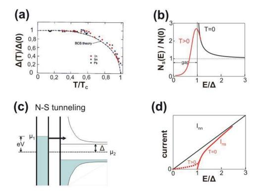
Figure 2.12: (a) Behavior of the superconducting gap if  $T \mapsto T_C$  (taken from [93]). (b) The BCS density of states. The sharp peak at the gap edge is washed out for finite temperature. (c) Schematical illustration of tunneling processes at N-S junctions: The potential difference applied at the leads has to exceed the superconducting gap  $\Delta_S$ . (d) I-V characteristic for a NS tunnel junction.
