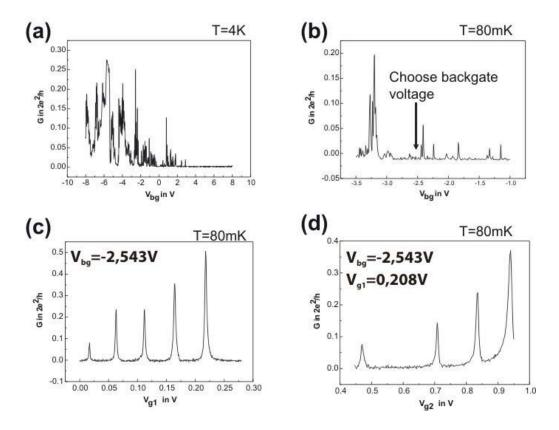
Figure C.1: In (a) Coulomb oscillations between the two normal contacts at T=4K are depicted. Clearly, the nanotube is semiconducting with a pinch-off voltage around 2V. (b) We choose a smooth gate region to fix the backgate voltage. In (c) we sweep sidegate 1. Once we find nice oscillations we fix sidegate 1. (d) Next we sweep sidegate 2. If we find nice oscillations also as a function of sidegate 2, we start the measurement of the stability diagram.
