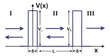
Figure 2.21: Our Carbon nanotube quantum dot is modeled by two potential barriers which can be approximated as Dirac  $\delta$ -functions. We calculate the transmission probability for incoming particles with an energy E > 0.
