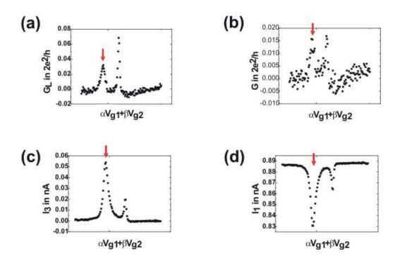
Figure D.1: We measure the differential conductance in the middle-injection setup at left (a) and right (b) lead. Afterwards we switch to the side-injection setup and measure the same region again. We measure  $I_1$  and  $I_3$  as defined in figure (4.4).
