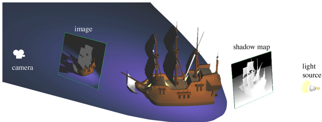
FIG. 11.1: Shadow map principle. A shadow map is computed from the point of view of the light source (z-values are represented as grey levels). Then each point in the final image is tested for shadow occlusion by projecting it back in the shadow map (gallion model courtesy of Viewpoint Datalab).
