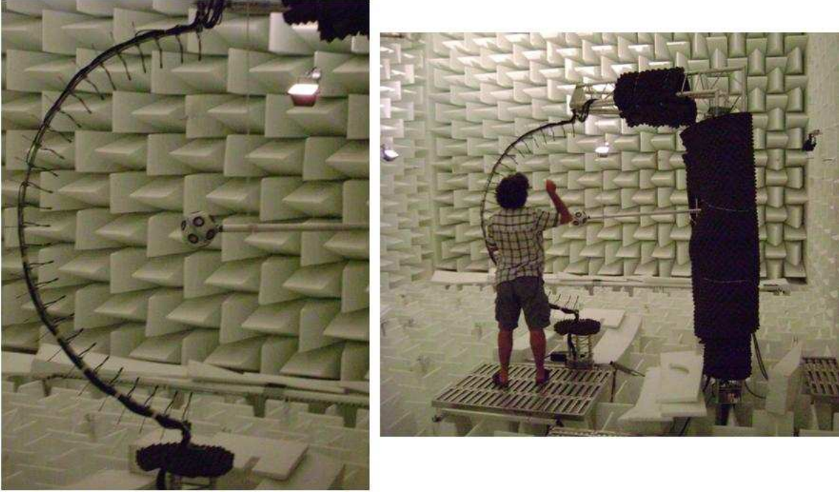
Figure 6.11: Experimental set-up for the directivity measurements at the large anechoic chamber of the Laboratory of Mechanics and Acoustics of the National Center for Scientific Research (UPR-7051, CNRS, Marseille, France).
