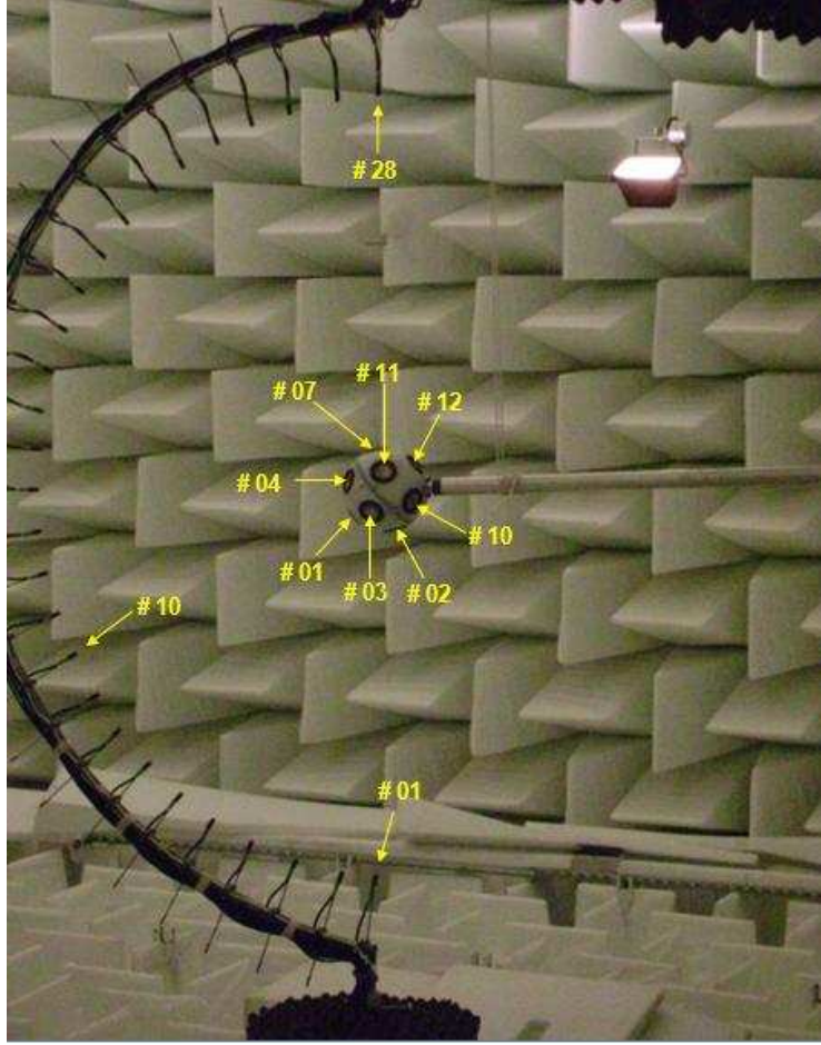
Figure 6.12: Experimental set-up for the directivity measurements with the driver and microphone labels indicated.
