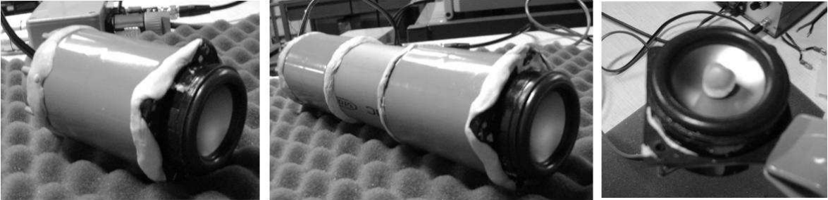
Figure 6.2: Experimental set-up for the electrical impedance measurements.
