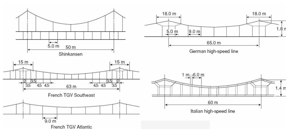
Figure 2.3. Some examples of overhead lines currently used [13].
