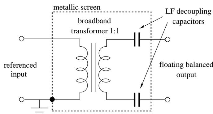
Figure 4.23. The schematic of the balun.
