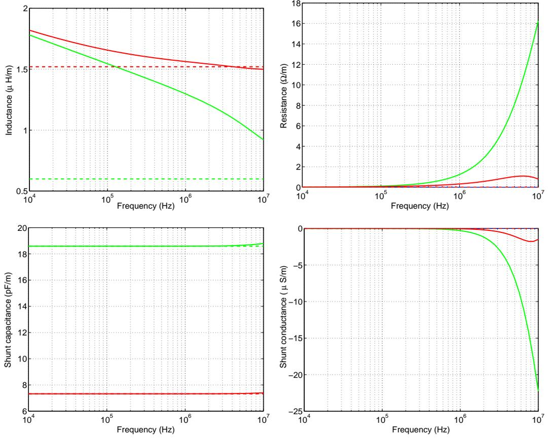
Figure 3.12. Per-unit-length parameters for a single wire line above a ground-plane, for  $h = 10 \text{ m}$  (red line) and  $h = 50 \text{ cm}$  (green line). Solid lines refer to an average soil ( $\sigma_g = 10 \text{ mS/m}$ ,  $\epsilon_g = 10$ ), whereas dashed ones refer to a PEC soil.
