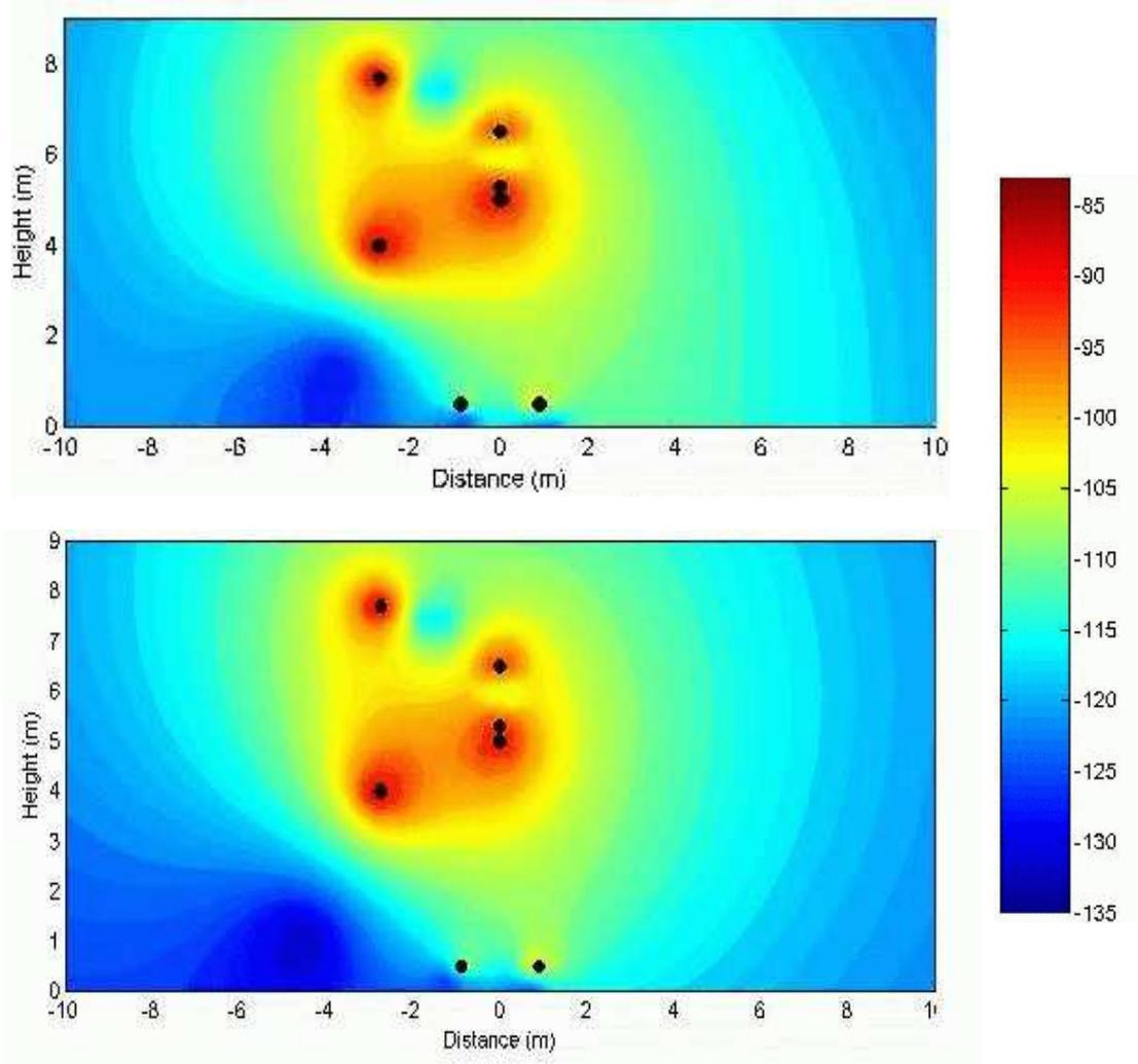
Figure 3.27. Transversal field topography at  $z_0 = 1500$  m for 3 km long railway line: (a) PEC soil, (b) average soil ( $\sigma_g = 10$  mS/m,  $\epsilon_g = 10$ ). The frequency here investigated is 1 kHz, dimensions in dB A/m.
