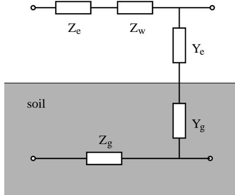
Figure 3.9. An electric-network interpretation of the per-unit-length parameters for a single-wire line above a finitely conducting soil, with the additional series and shunt terms accounting for the soil non-ideality.
