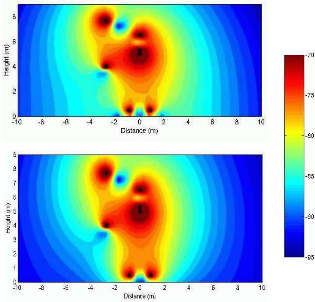
Figure 3.28. Transversal field topography at  $z_0 = 1500$  m for a 3 km long railway line: (a) PEC soil, (b) average soil ( $\sigma_g = 10$  mS/m,  $\epsilon_g = 10$ ). The frequency here investigated is 2 MHz, dimensions in dB A/m.
