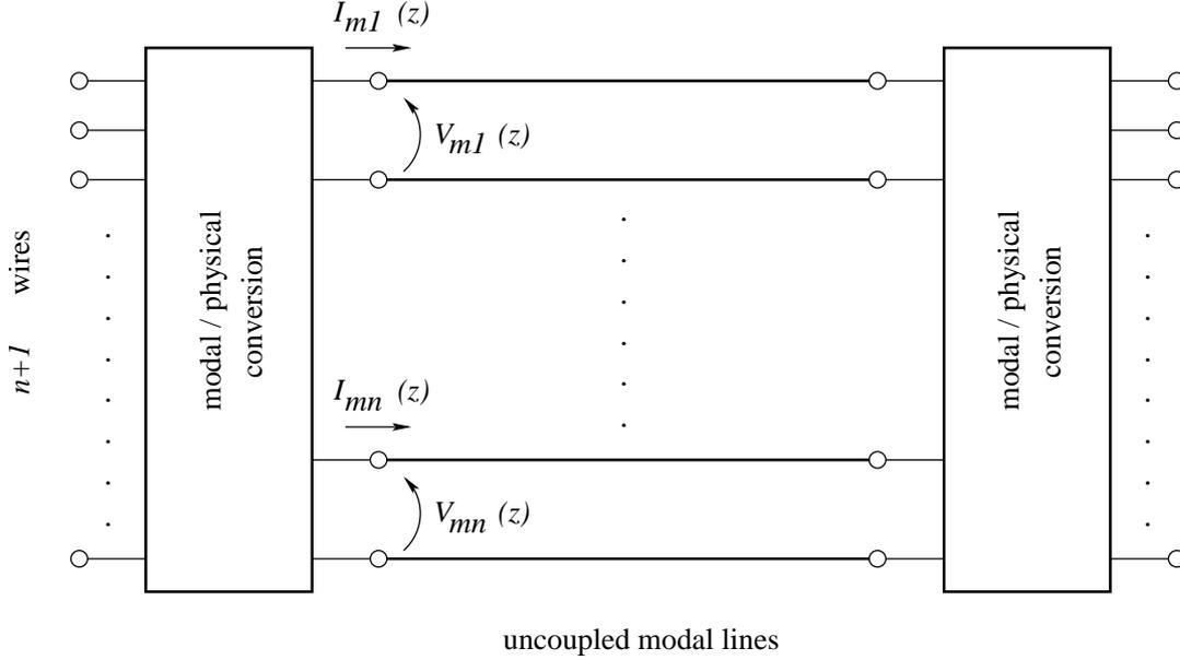
Figure 3.6. An electric-network interpretation of the modal theory, with uncoupled scalar modal lines, connected to two networks allowing the conversion from modal quantities back/to physical ones.
