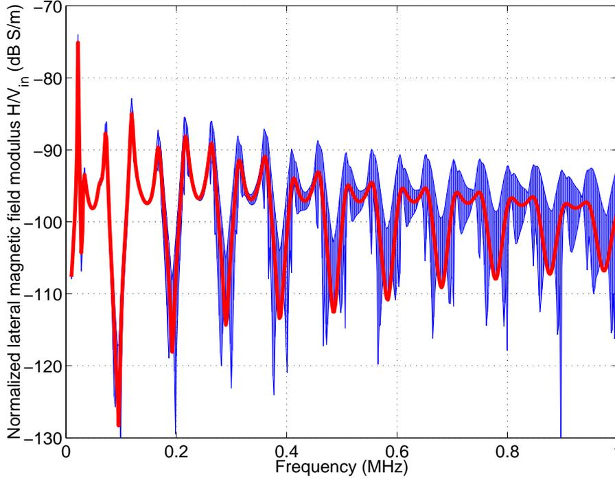
Figure 4.19. The magnetic field computed for the line in Figure 3.25, with its far-end open-circuited, for nominal values (solid line) and the  $\sigma_H$  margin (shaded area) estimated from the small-error sensitivity analysis, for relative errors set to 5 %, but for the line length, set to 1 %.
