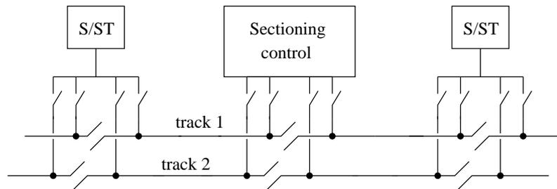
Figure 2.10. A general bilateral layout for a DC supply for a two-track line. The sectioning control unit allows the tracks to be connected in parallel or to cut off one half of them.
