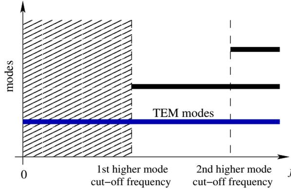
Figure 3.2. Mode-density vs. frequency for an MTL. For the shaded frequency range the propagation along the MTL is dominated by TEM modes.
