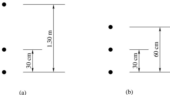
Figure 4.6. The configuration chosen for assessing the importance of the catenary camber on the per-unit-length parameters of the catenary. The two cases refer to the two extreme positions of the catenary camber, for a composite overhead line.
