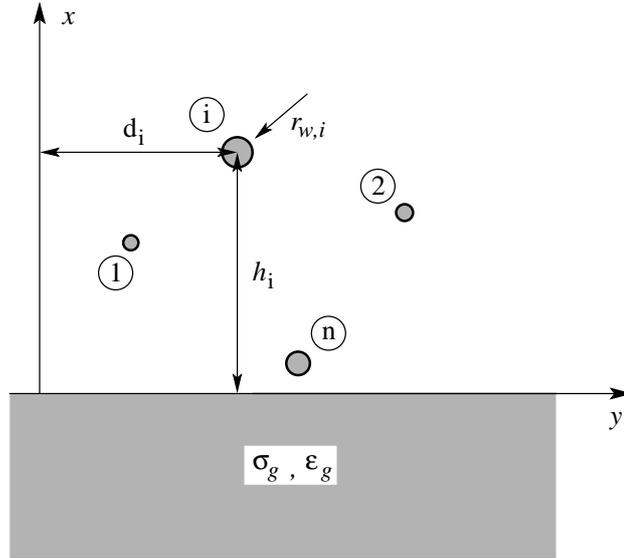
Figure 3.13. A multiconductor transmission-line above a homogeneous soil.
