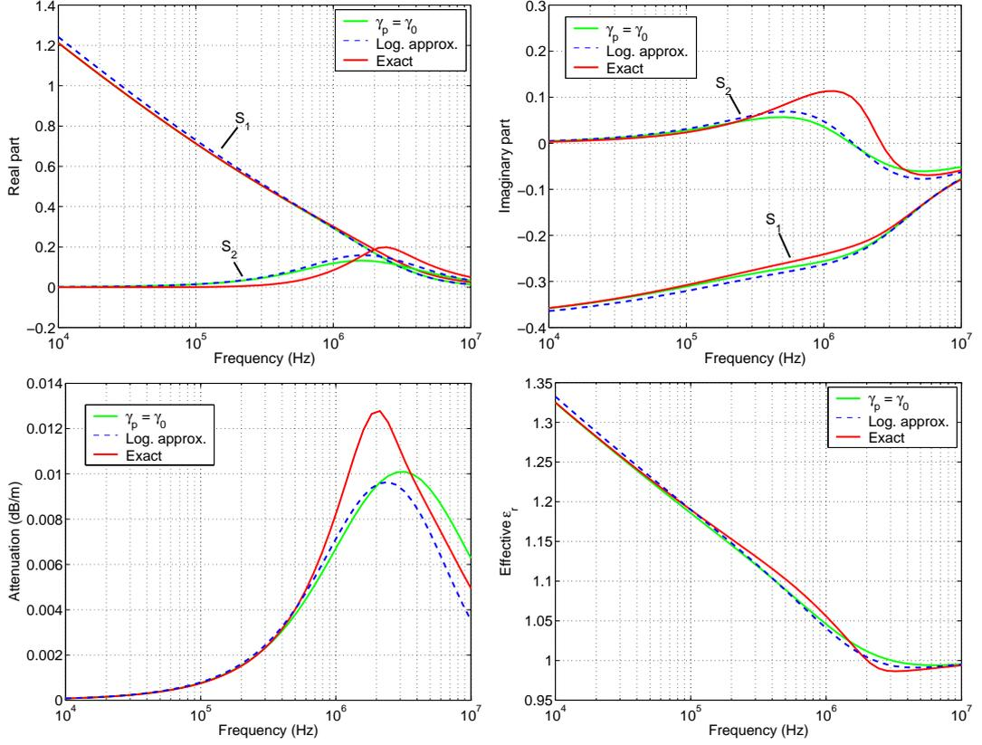
Figure 3.10. Single-wire line (10 m high) over an average soil ( $\sigma = 10$  mS/m,  $\epsilon_g = 10$ ): Sommerfeld's integrals (a)-(b), line attenuation (c) and effective dielectric constant (d).
