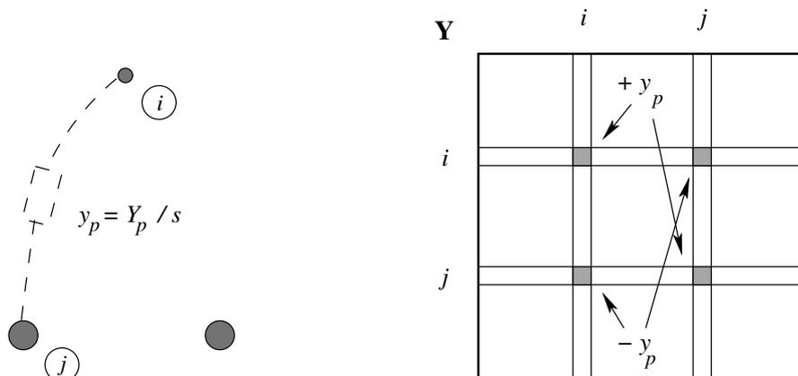
Figure 4.11. An example of how identical lumped admittances  $Y_p$  periodically connected with spacing  $s$  can be included into the per-unit-length admittance matrix. The admittances are connected between the conductors  $i$  and  $j$ .
