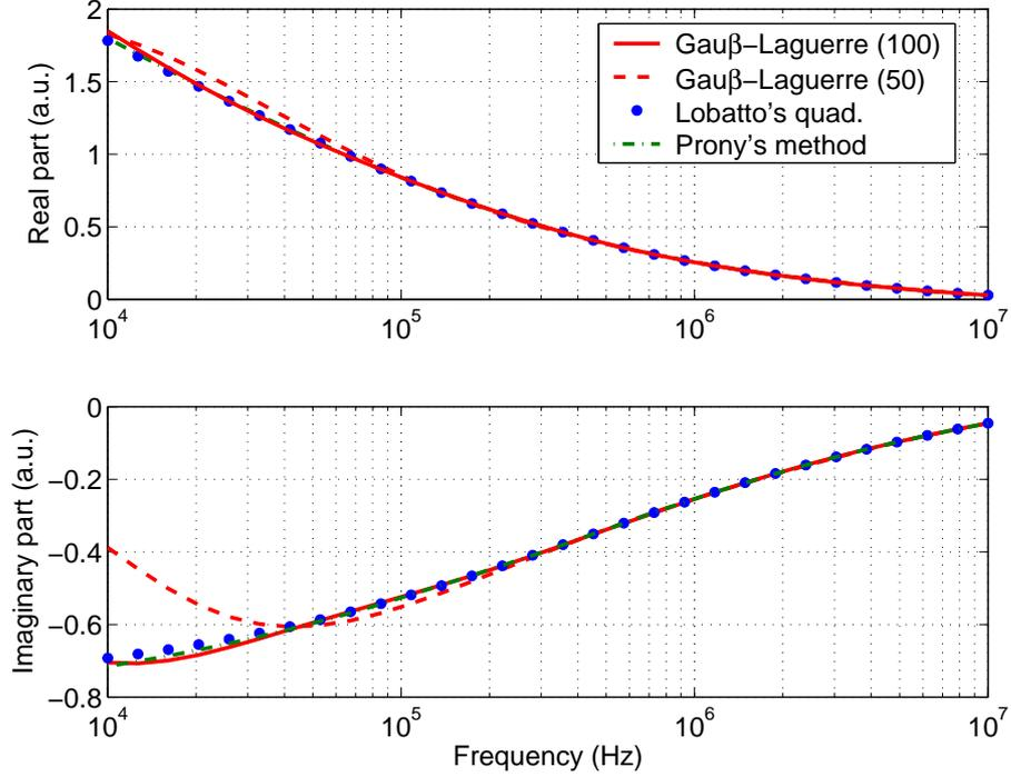
Figure 3.20. A comparison between the results obtained with different numerical integration algorithms, as applied to  $\mathcal{S}_3$ , with  $h = 5$  m,  $x = 2$  m,  $y = 10$  m,  $\sigma_g = 10$  ms/m and  $\epsilon_g = 10$ .
