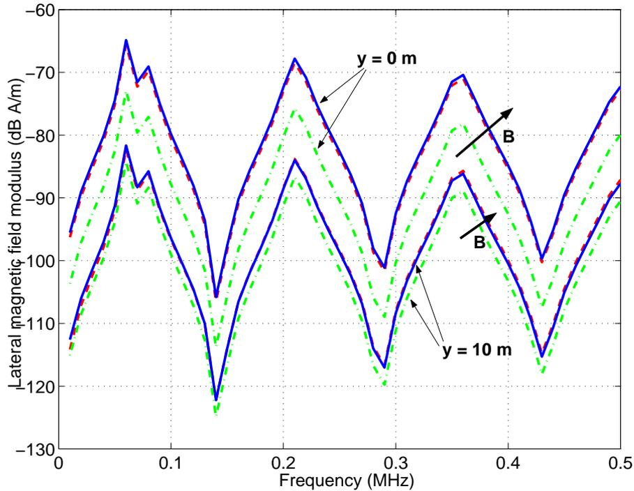
Figure 3.23. The lateral component of the magnetic field as computed by Sommerfeld’s model. The two groups of spectra refer respectively to  $y = 10$  m and  $y = 0$  m. In the first case three spectra have been computed for  $B = \{10,20,100\}$  m and in the latter one for  $B = \{2,5,20\}$  m. The arrows shows the evolution of the spectra as  $B$  gets bigger.
