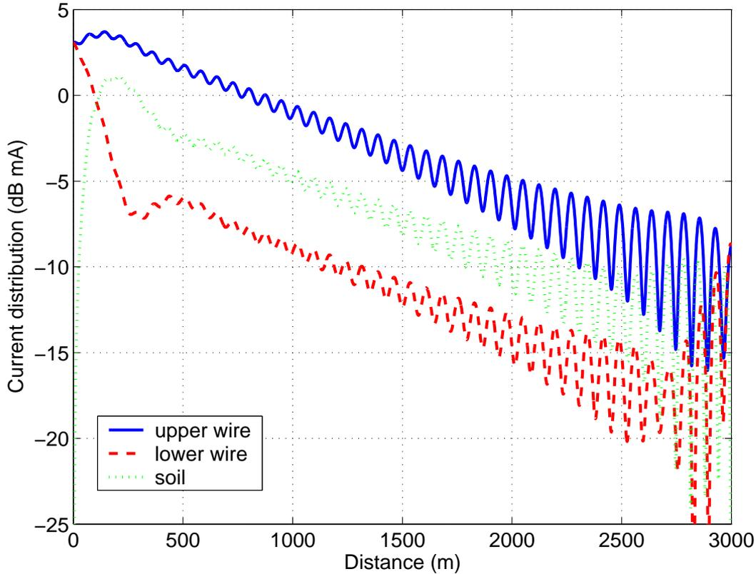
Figure 3.26. The current distribution along the two conductors of the line in Figure 3.25, for a far-end load of  $50 \Omega$ , at 2 MHz.
