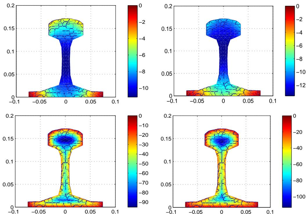
Figure 3.15. The current density distribution inside a rail 10 cm above the soil interface, at 1 kHz (first row) and 2 MHz (second row), for an average soil (first column,  $\sigma_g = 10$  mS/m,  $\epsilon_g = 10$ ) and a perfectly conductive one (second column). The colors represent the normalized intensity of the current density, as expressed in dB.
