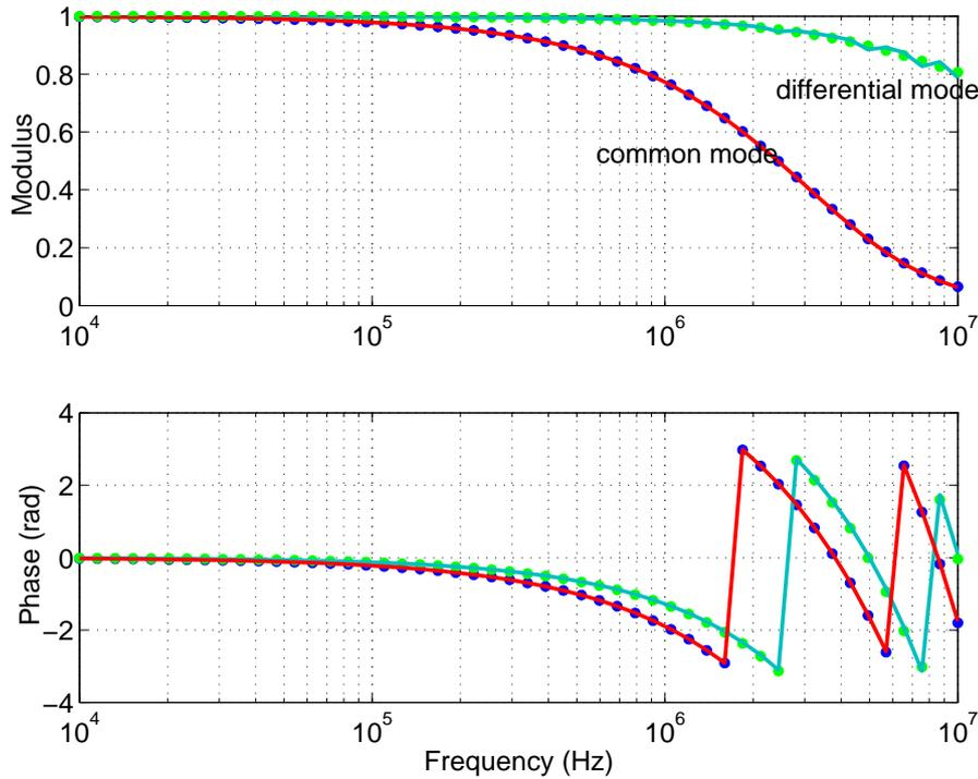
Figure 4.13. The attenuation and phase of the forward-travelling propagation exponential, as computed for a uniform two-wire line (dots) and for a periodically loaded one (solid lines), with spacing 60 m and periodical shunt-capacitances of 10 pF. The only visible effect of shunt-capacitances on the propagation is in the attenuation of the differential mode (the least attenuated one) in the higher frequency-range.
