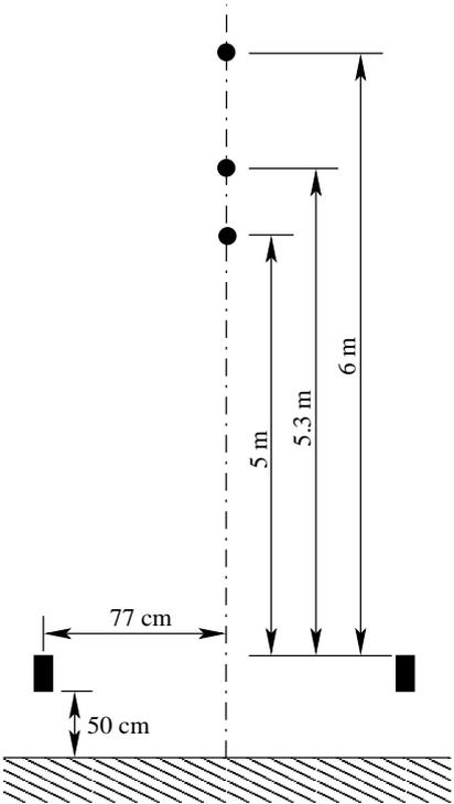
Figure B.1. The cross-section configuration referred to throughout this dissertation. The radius of the three overhead wires is 6 mm.
