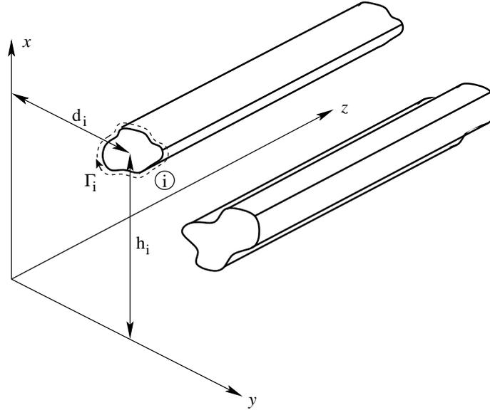
Figure 3.1. The generic structure of a uniform open multiconductor transmission-line.
