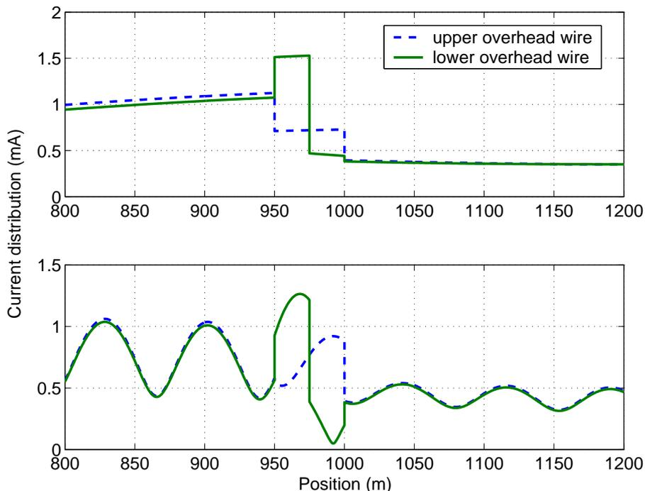
Figure 4.3. The current distribution along a two-wire catenary, 2 km long with droppers every 50 m, with a  $200\ \Omega$  load at  $z = 975$  m, connected as in Figure 4.2b. The two figures refer, respectively, to the current distribution at 100 kHz and 2 MHz. Although differential modes are excited in the proximity of the connection, a couple of droppers suffice for enforcing again a common-mode propagation.
